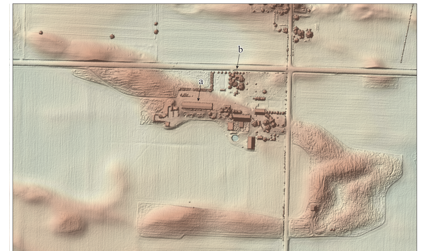
Figure 3 LIDAR-based digital surface model (DSM) of the same dune feature. In contrast to a DTM, which represents only ground features, a DSM portrays all aboveground features. Compare the landscape features observable on the DSM with the features visible on this DTM. For example, note the farmstead structures situated atop the dune at (a) and the farmstead house situated at the base of the dune, surrounded by trees (b). Scale is 1:6,000 (1 in. = 500 ft).
