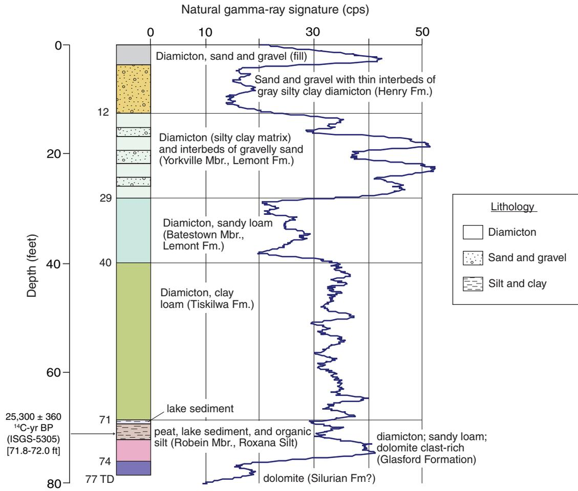
**Figure 7** Lithologic and gamma-ray log of boring 34553 (SE NE Sec. 21, T41N, R8E, elevation 807 feet) located in College Park, Elgin, Illinois. This boring was sampled by continuous coring and is used in cross sections C–C' and E–E'.
