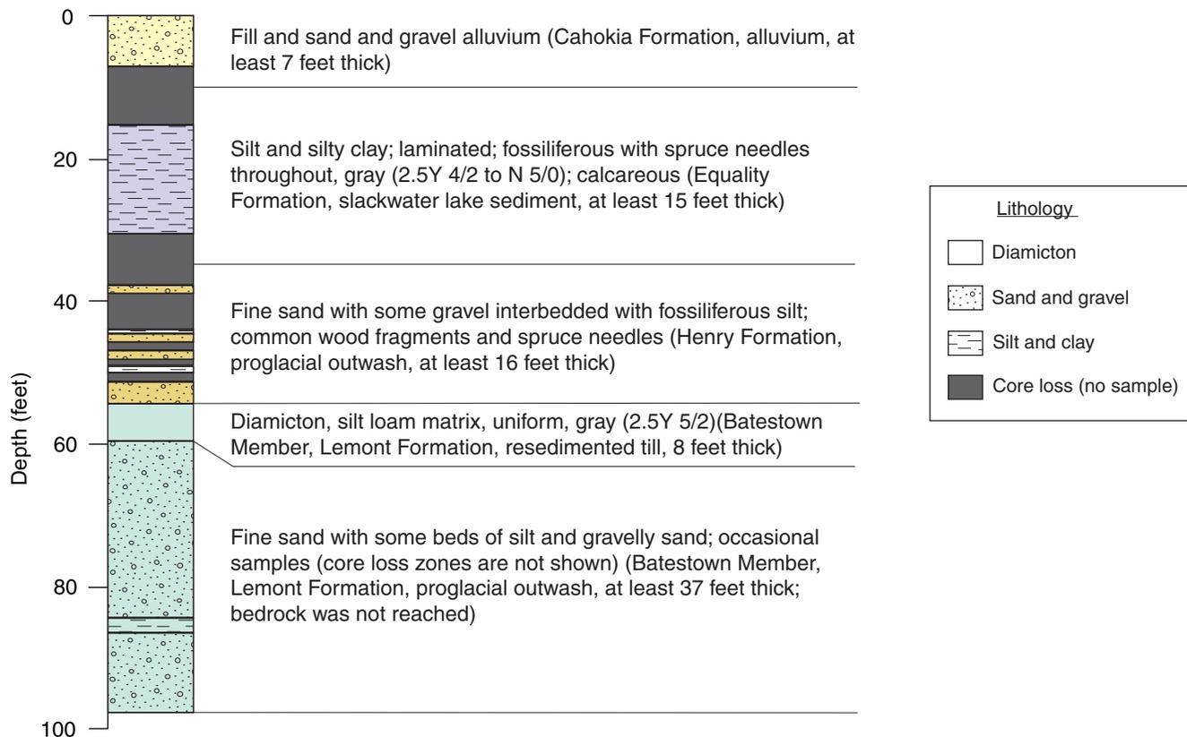
**Figure 8** Lithologic log of boring 34268 (NW NW Sec. 9, T41N, R8E, elevation 815 feet) located in the floodplain of Tyler Creek about 150 feet east of the Randall Road bridge, Elgin, Illinois. Core loss zones are indicated in black. Cores were sampled from a depth of 0 to 53 feet; the boring was extended to 97 feet by augering. This boring was not used in a cross section.
