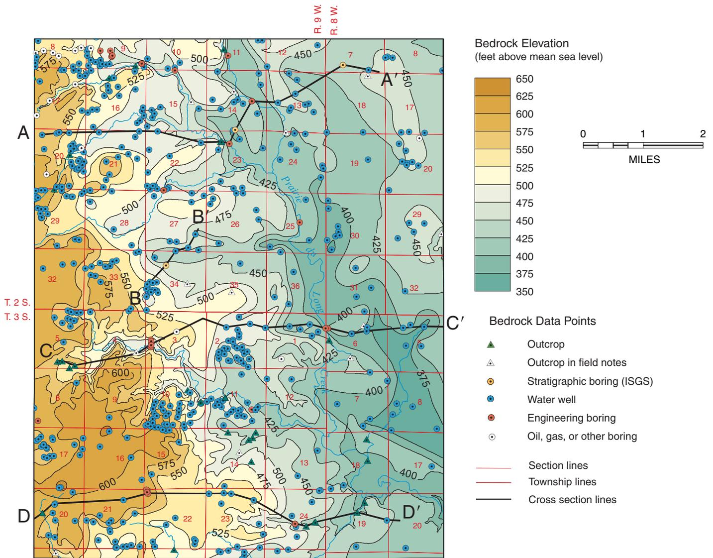
**Figure 2** Bedrock topography of the Paderborn Quadrangle with shaded relief. Localities of all borehole and outcrop data that reliably indicate the bedrock surface are shown (many data are not shown on the surficial map). In the southeast, the main valley is buried by 70 to 100 feet of sediment. Bedrock crops out in most tributary valleys west of Prairie du Long Creek. Scale is 1:100,000.
