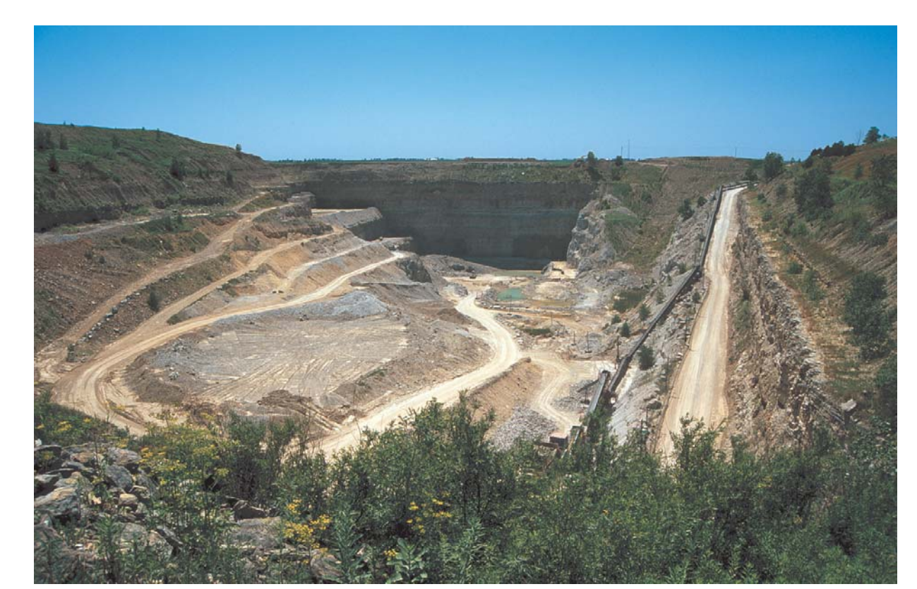
View of the Tuscola Quarry (Section 6, T. 15 N., R. 9 E.), looking west. The quarry is the only site in the quadrangle where the bedrock surface is exposed. The dolomite and limestone forming the vertical wall of the quarry consist of the Devonian Lingle and Grand Tower Formations.
