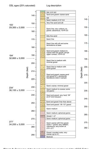
Figure 2. Boring log of the basal sand and gravel interval of the ISGS Fidler #1 boring and optically stimulated luminescence (OSL) ages.
