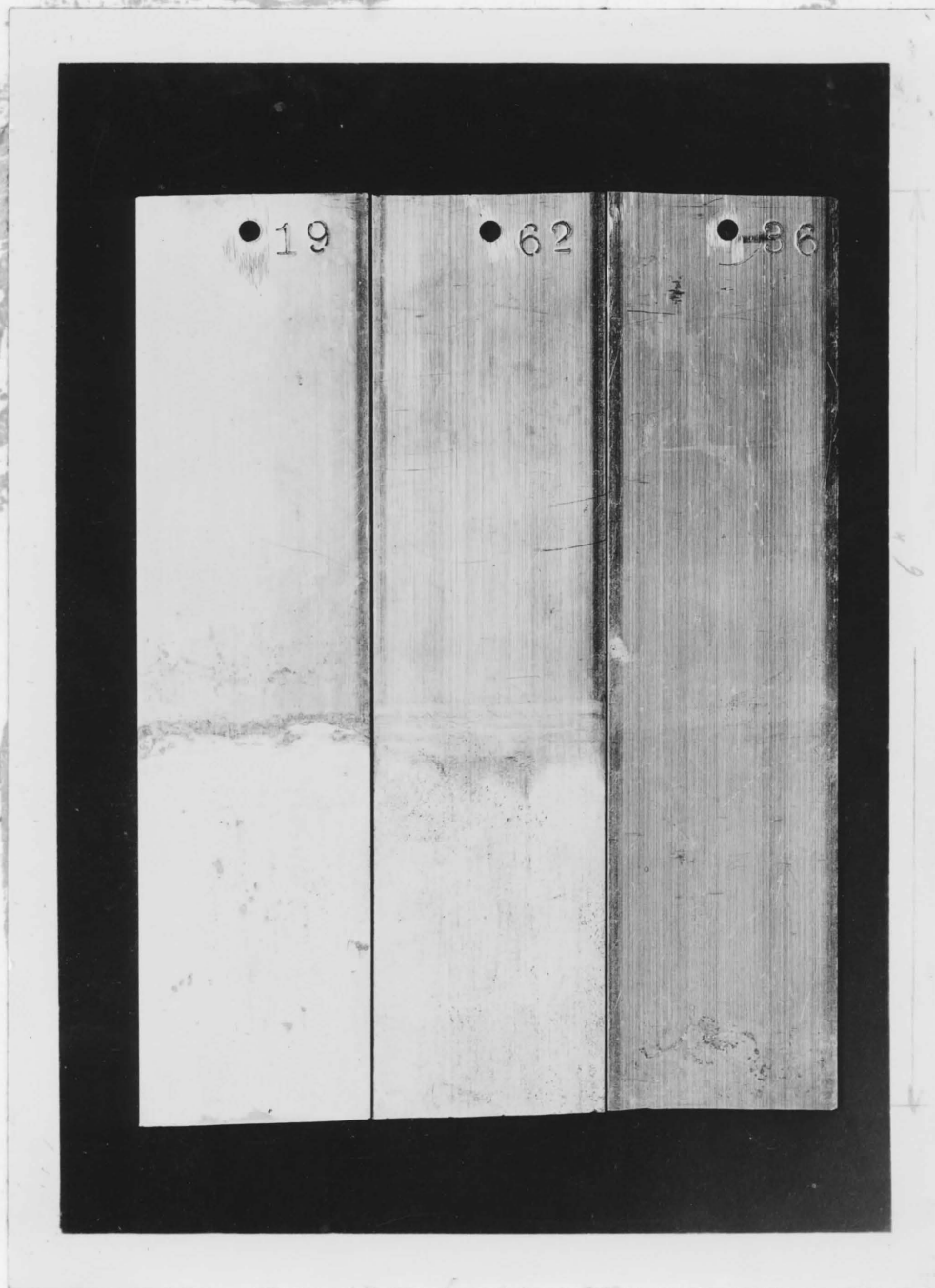
Figure 6. Steel strip samples, anodic (A), neutral (B), and cathodic (C) continuously immersed in Tóhill brine for two weeks with a current density of 0.22 ma. per sq. in. Natural size.
