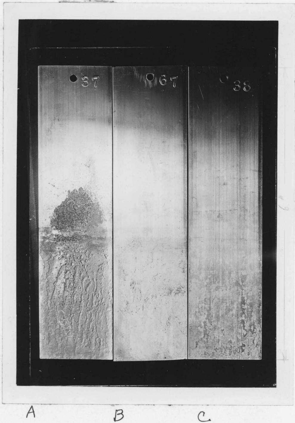
Figure 8. Steel strip samples, anodic (A), neutral (B), and cathodic (C) intermittently immersed in Tohill brine for two weeks with a current density of 1.1 ma. per sq. in. Natural size.
