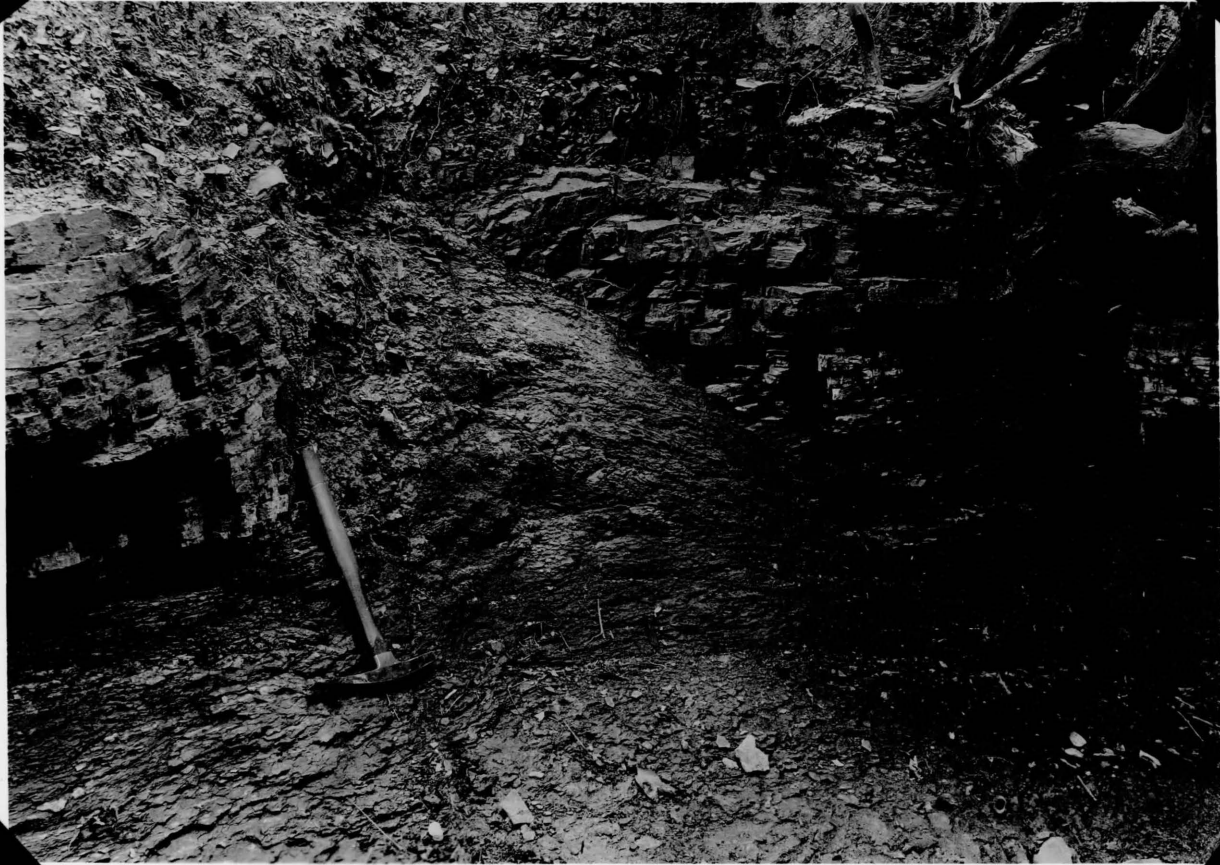
Fig. 133 . Horseback (left) and clay vein (right) in the Springfield (No. 5) coal along a ravine in the SE. \frac{1}{4} sec. 13, T. 6 N., R. 3 E. (Putnamwp.) (See also fig. 59 )
