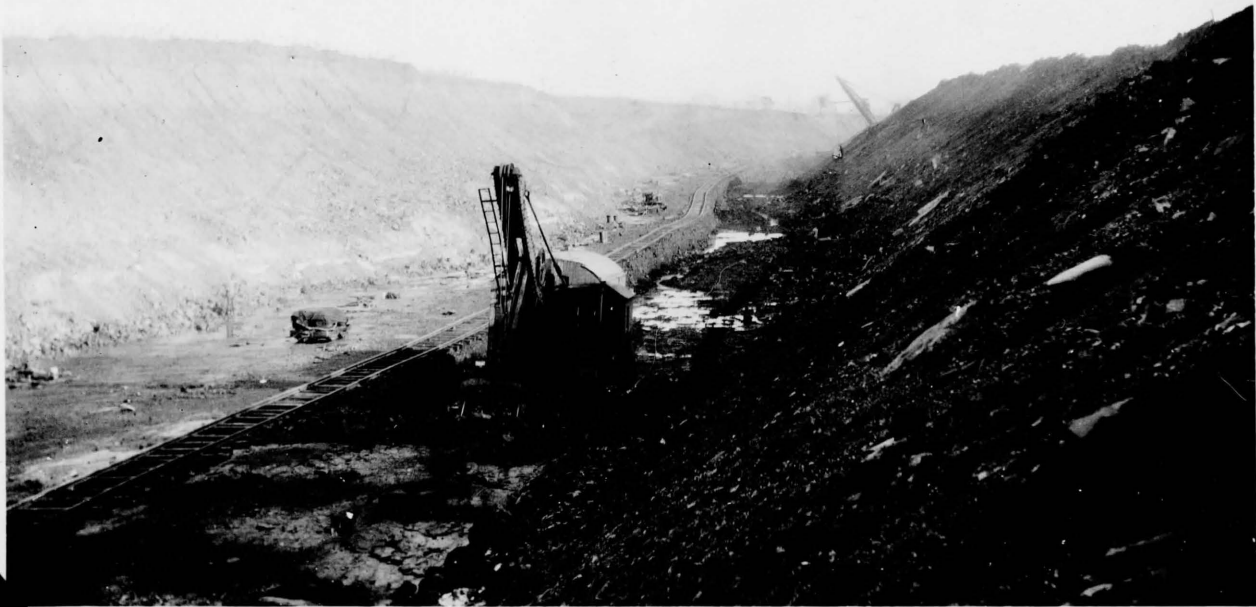
Fig. 102. General view of a stripping face of the United Electric Coal Company's Mine no. 9, southeast of Cuba in the SW. \frac{1}{4} NW. \frac{1}{4} sec. 27, T. 6 N., R. 3 E. (Putman wp ). The strip face at the left is about 30 feet high, consisting of about 19 feet of loess and drift and 11 feet of shale and limestone. Several large blocks of the St. David limestone are seen in the debris pile# at the right.
