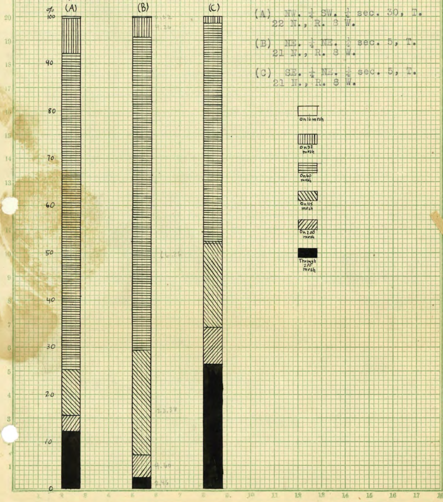
Fig. 9a. Sieve analyses of (A) sandy loam from level part of later Wisconsin terrace, (B) sand from top of sand dune and (C) sandy loam from the bottom of a poorly drained depression enclosed by sand dunes to show the relation between topographic position and the concentration of the fine silts (through 200 mesh) in the surface soil.
