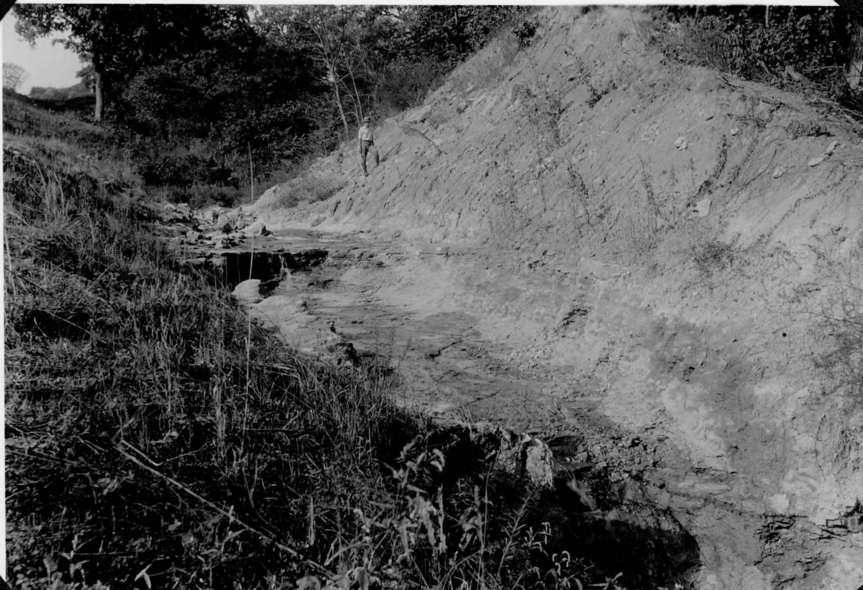
Fig. 144 Exposure of Pottsville strata in the small ravine south of Otter Creek just west of State Highway 31 in the NW. \frac{1}{4} SE. \frac{1}{4} sec. 30, T. 4 N., R. 3 E. (Isabel) wp . Clay samples 118 and 119 were taken from this exposure, no. 118 from the lowest bed exposed here, shown at the lower right, and no. 119 from the clay or shale below the ledge of sandstone which forms a waterfall in the middle distance. The man is standing at the horizon of the Seahorne limestone, which is separated from the sandstone below by a layer of clay containing gypsum crystals.
