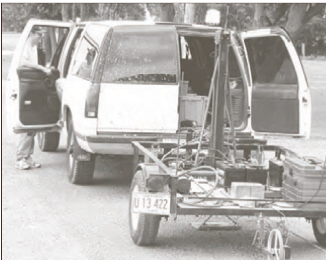
André Pugin, ISGS geophysicist, in the process of collecting seismic reflection data about the Mahomet Sand. The landstreamer, an ISGS innovation, allows these descriptive data to be collected faster and more effectively, with fewer staff, than previous collection technology.
