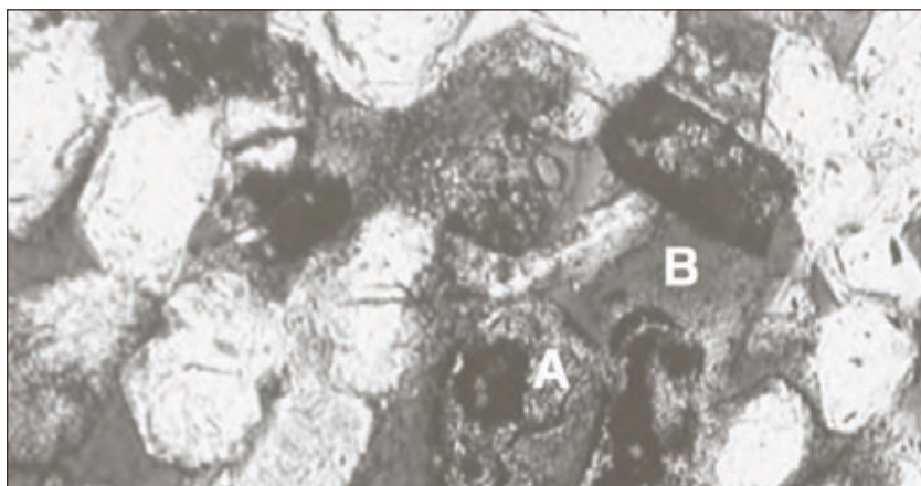
Benoist reservoir sandstone, showing potassium feldspar grains undergoing degradation (A) and secondary porosity formed from dissolution of grains (B). Shell Oil Company, Hanseman No. 2 Well, depth 1,367 feet.
