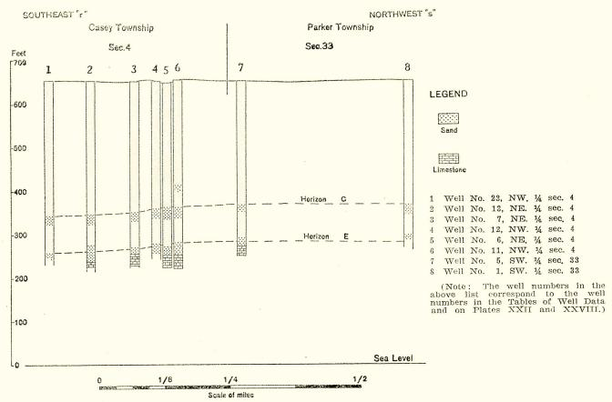
Detailed cross-section (r-s, Plate XXI), showing the Pennsylvanian sands and the top of the Lower Mississippian lime along a northwest-southeast line across the North Casey pool. The stratigraphic position of contour horizons C and E is shown diagrammatically on Plate XXIII. Note the lesser thickness of Pennsylvanian sand where the lime is high (No. 7), than where it is lower (Nos. 2, 3, 5, and 6).
