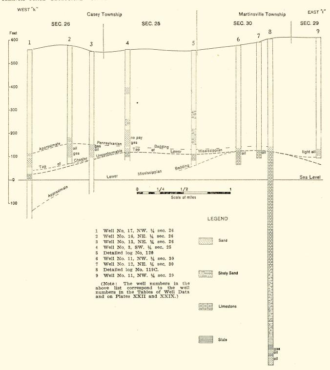
Detailed cross-section (k-l, Plate XXI), showing the Pennsylvanian sands and bedding, the Chester remnant, the eroded top of the Lower Mississippian, and the Lower Mississippian bedding, in the Casey and Martinsville pools.
