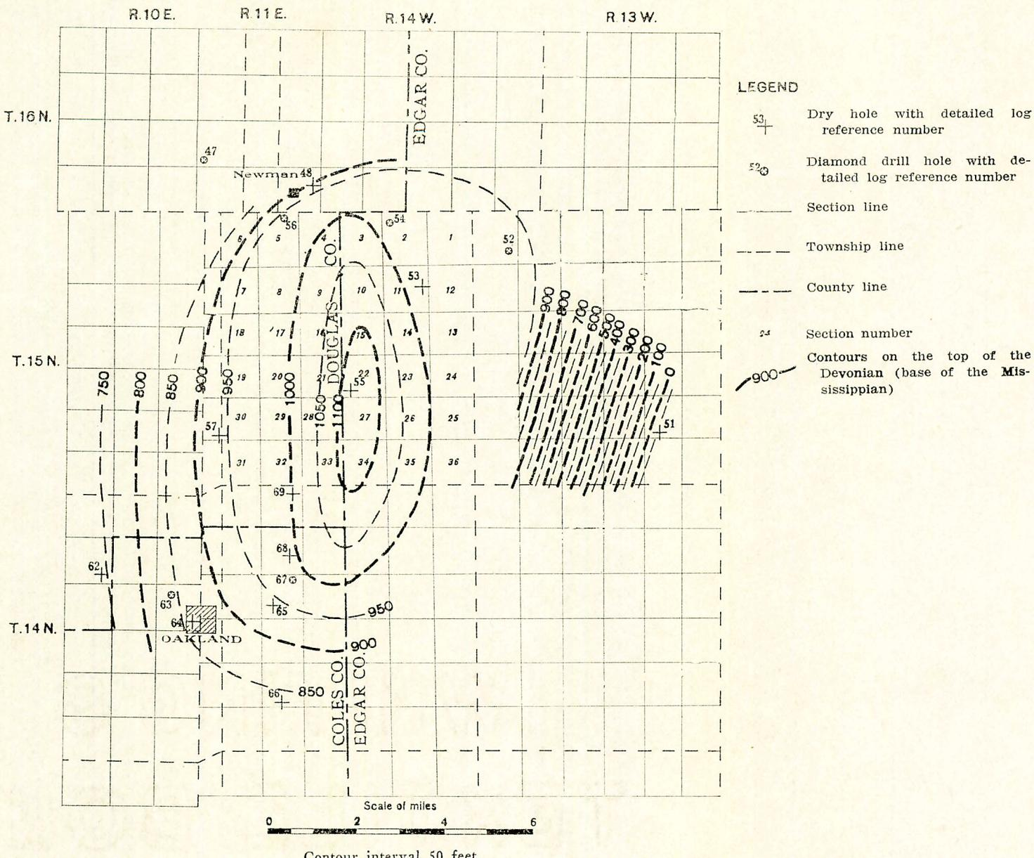
Structure contour map of the Oakland dome. The contours give the elevations of the top of the Devonian (base of the Mississippian) above a datum 1200 feet below sea level. Holes Nos. 62, 65E, and 66 penetrated the "Trenton," but all others penetrated only short distances into the Devonian. Cross fold No. 8 may modify the contours on the eastern side of the dome.
