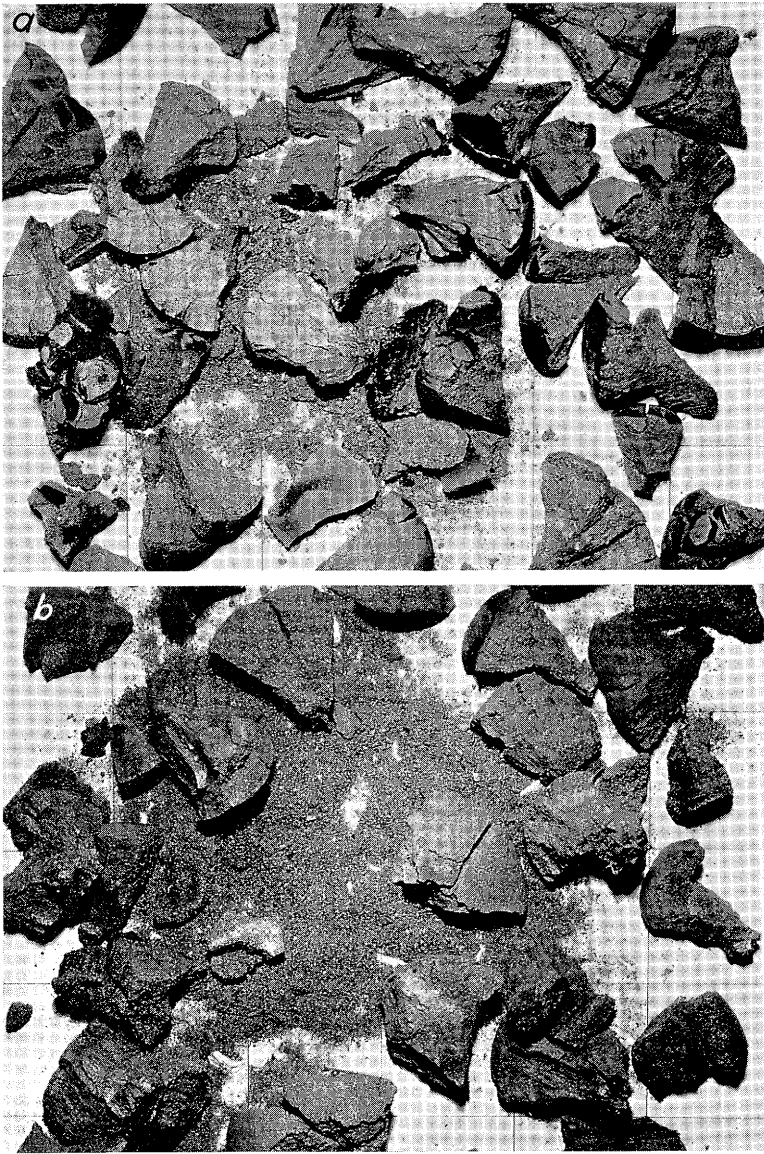
Fig. 49.—COKES FROM FRANKLIN AND RANDOLPH COUNTIES, ILLINOIS, No. 6 COAL, MADE IN SIX-INCH RETORT (3-INCH GRID).
