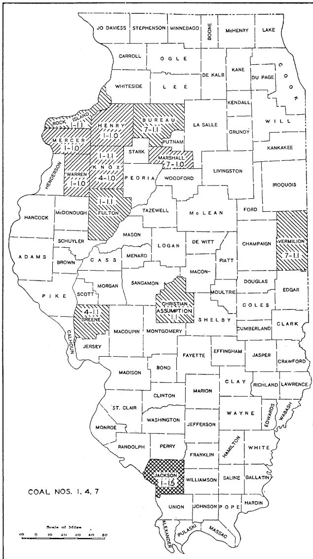
Fig. 13.—COUNTY AVERAGE CARBON RATIOS FOR COAL NOS. 1, 4, AND 7 AND ASSUMPTION COAL IN CHRISTIAN COUNTY.
