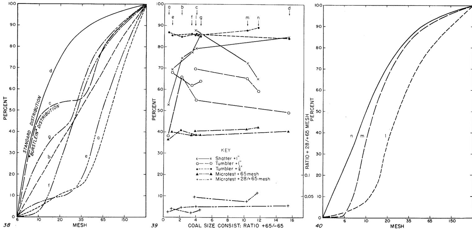
FIG. 38.—No. 6 coal: Influence of selective breakage on distribution of particle size for series 1 and 2. Reference pillar. Use with fig. 39 (table 12).
