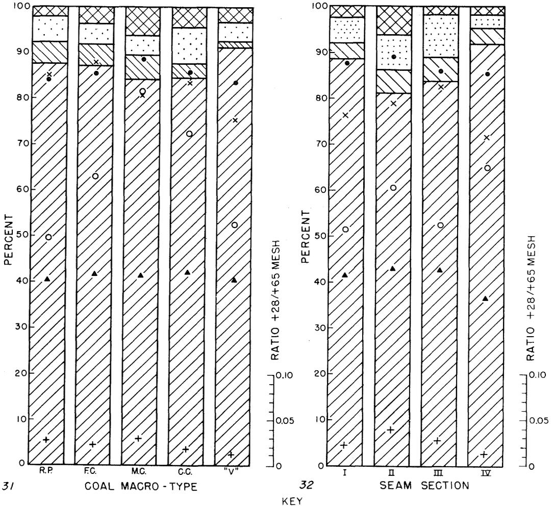
FIG. 31.—No. 6 coal: Influence of coal macro-type on coke. Reference pillar, fine, medium and coarse clarains, "vitrain" all in standard size consists, and standard coking conditions (tables 3A, 10).
