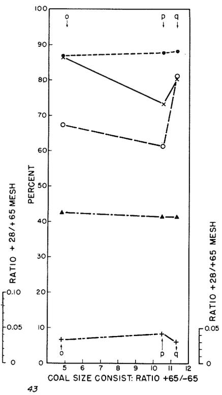
FIG. 41.—No. 6 coal: Influence of selective breakage on distribution of particle size for series 3 and 5. Reference pillar and medium clarain. Use with figs. 42 and 43 (table 12).
