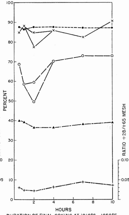
FIG. 27.—No. 6 coal: Influence of final coking temperature on coke. Reference pillar, standard size consist, standard charging temperature, rate of temperature increase, and final coking period 2 hours (table 8).
