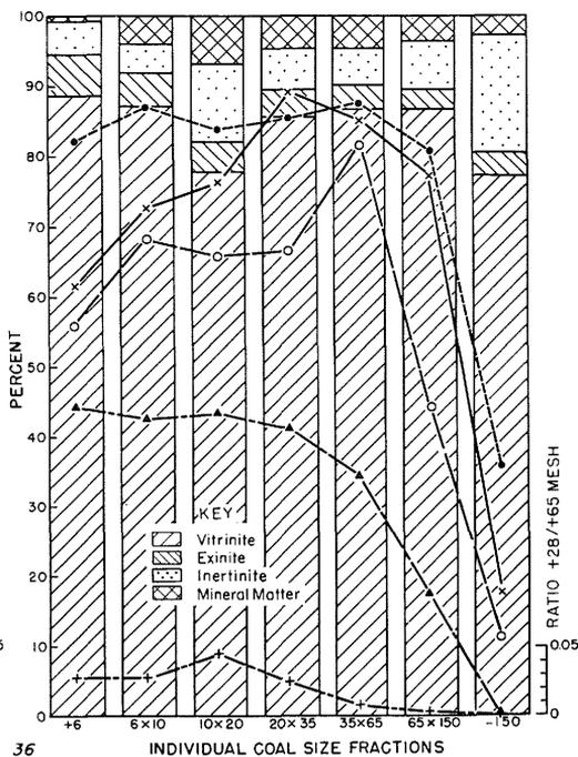
FIG. 36.—No. 6 coal: Character of coke produced from individual size fractions related to petrographic constitution (vitrinite, exinite, inertinite, and mineral matter). Medium clarain, standard coking conditions (tables 3B, 11).
