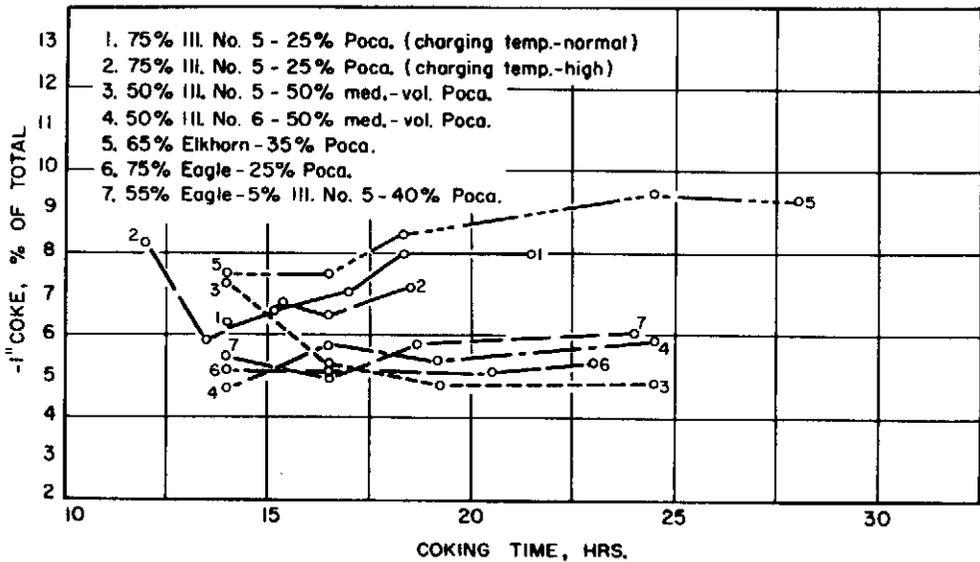
Fig. 11. - Minus 1-inch coke vs. coking time.
