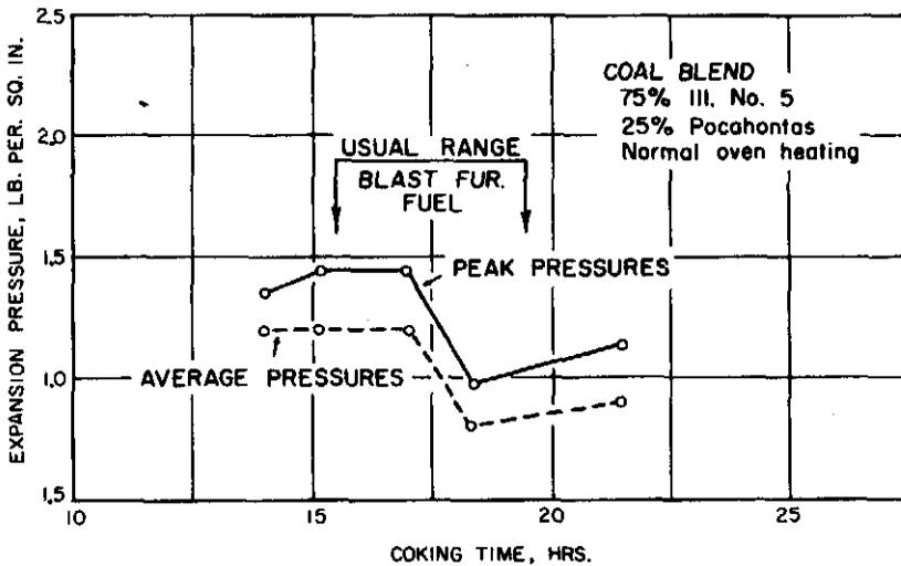
Fig. 3. - Expansion pressure vs. coking time.
