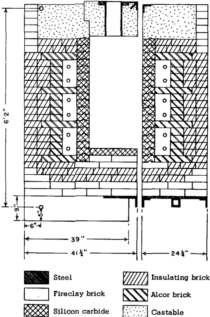
Fig. 1. - Cross section of oven through brickwork.
