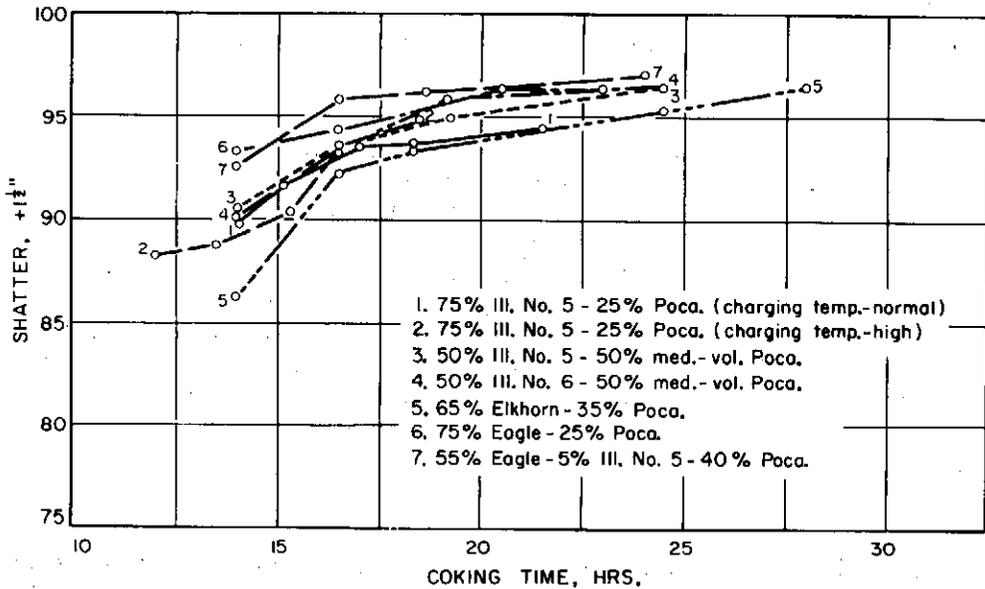
Fig. 13. - Shatter (plus 1 1/2-inch) vs. coking time.
