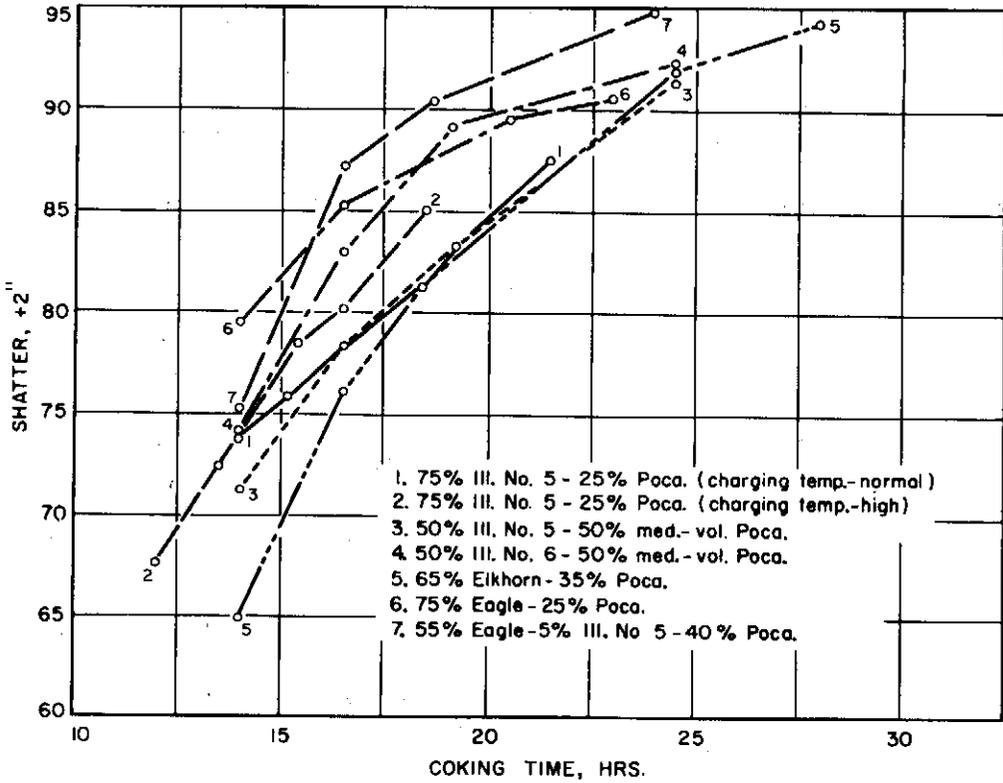
Fig. 12. - Shatter (plus 2-inch) vs. coking time.
