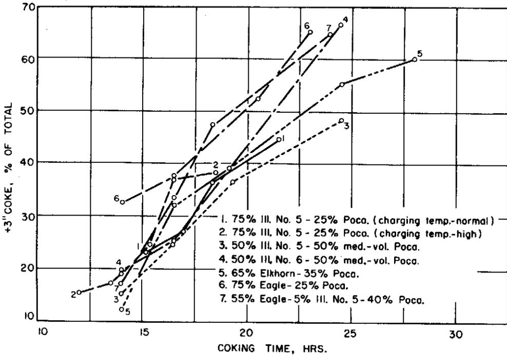
Fig. 10. - Plus 3-inch coke vs. coking time.
