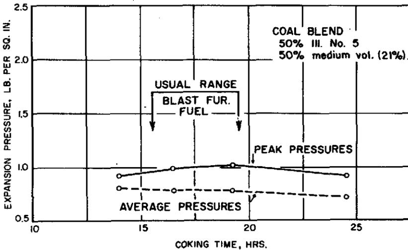
Fig. 5. - Expansion pressure vs. coking time.
