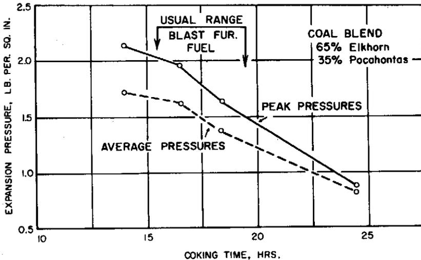
Fig. 7. - Expansion pressure vs. coking time.
