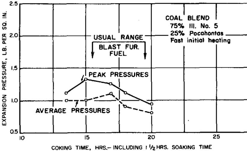
Fig. 4. - Expansion pressure vs. coking time.
