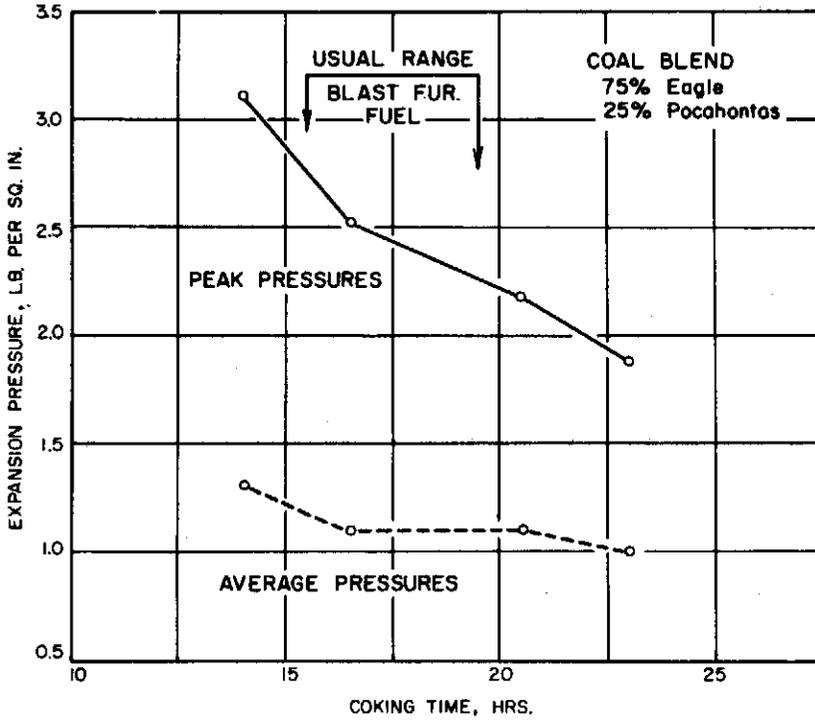
Fig. 8. - Expansion pressure vs. coking time.
