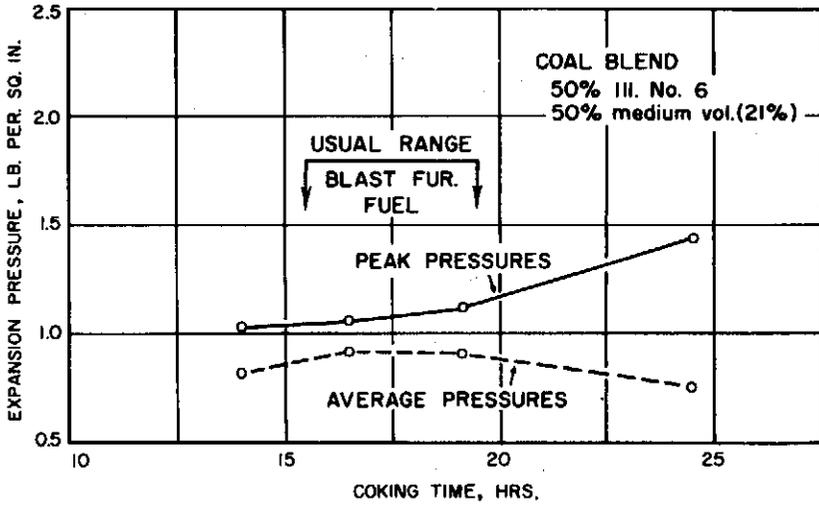
Fig. 6. - Expansion pressure vs. coking time.
