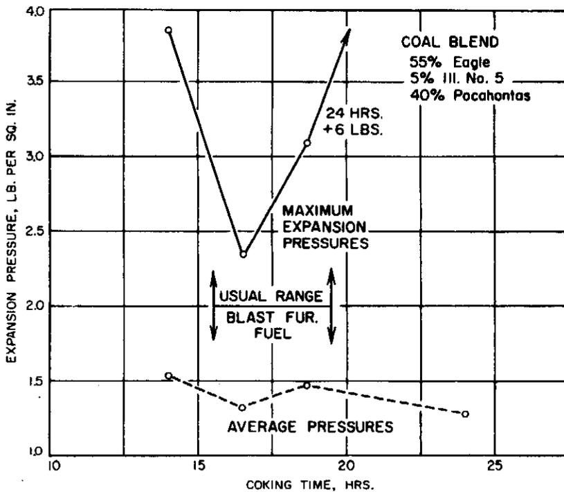
Fig. 9. - Expansion pressure vs. coking time.
