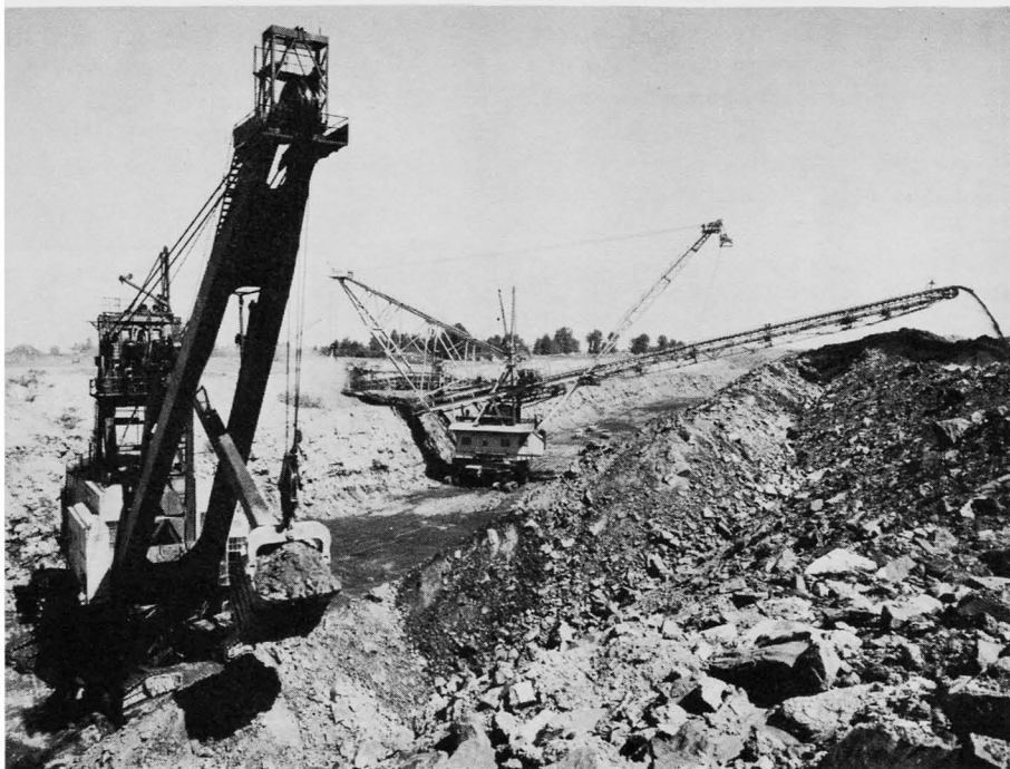
A. - Wheel excavator removing unconsolidated overburden from No. 6 Coal west of DuQuoin, Perry County.
