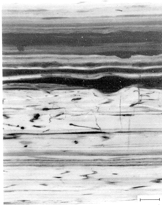
FIGURE 15. Thickly laminated Selmier Shale. The base of the granular appearing calcareous silt bed at the top of the sample pinches and swells, probably because of soft sediment deformation. Several pyritic burrows, deformed by compaction, are present in the massive central portion of the sample. Radiograph, Orbit Gas #1 Clark core, 2263.7 ft (sample 1KY7L1), Christian County, Kentucky. Bar scale = 1 cm.
