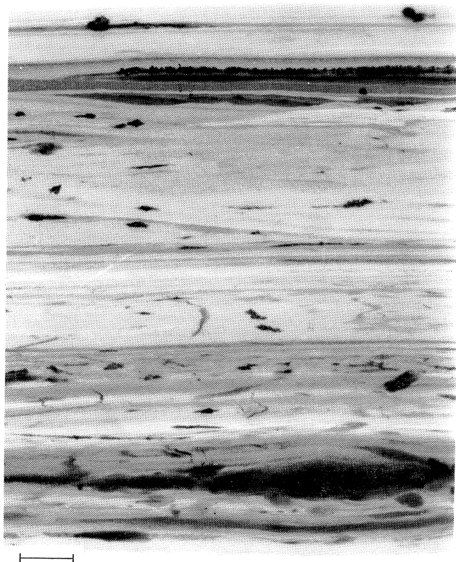
FIGURE 14. Poorly laminated Selmier Shale. Laminae are discontinuous and widely spaced; the large lenticular feature near the base of the sample may be a soft sediment deformation structure. Several faint silt filled burrows cut across the bedding and truncate laminations. Radiograph, Orbit Gas # 1 Clark core, 2270.2 ft (sample 1KY8C1), Christian County, Kentucky. Bar scale = 1 cm.
