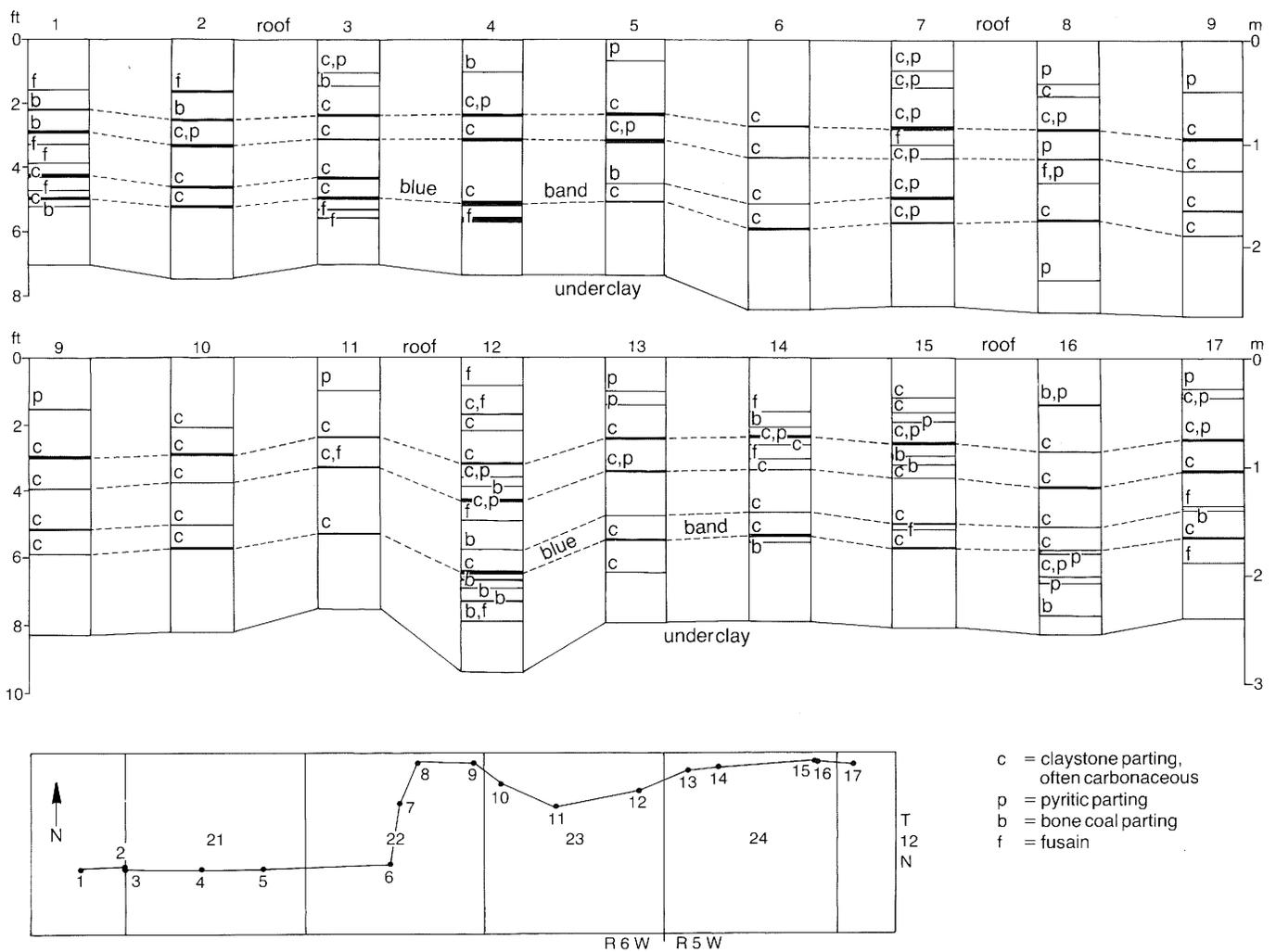
**Figure 5** Measured sections of Herrin Coal at Crown II Mine, illustrating continuity of shale partings; length of traverse is about 5 miles (8 km). By Philip J. DeMaris.
