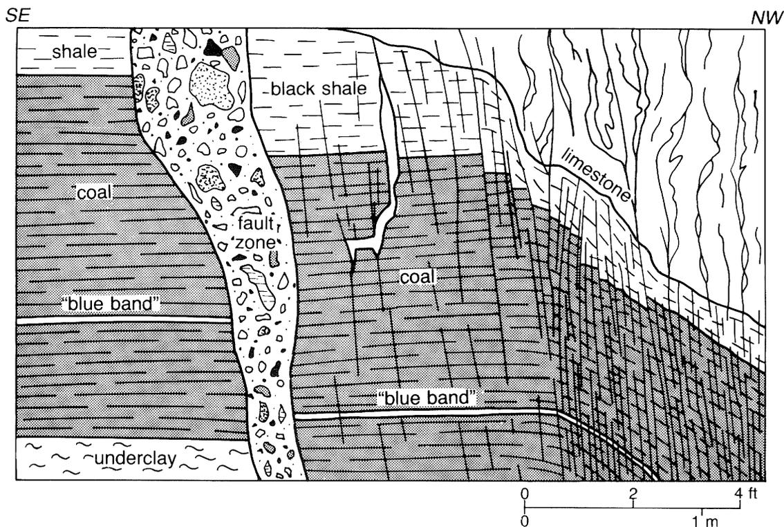
**Figure 20** Field sketch of part of strike-slip fault zone in Crown II Mine. The wide vertical fissure (left of center) contains a loosely packed jumble of coal, shale, limestone, and sandstone fragments. To the right, coal and roof are shattered by hundreds of vertical fractures, many of them open. Fissures and open fractures yield large amounts of water.
