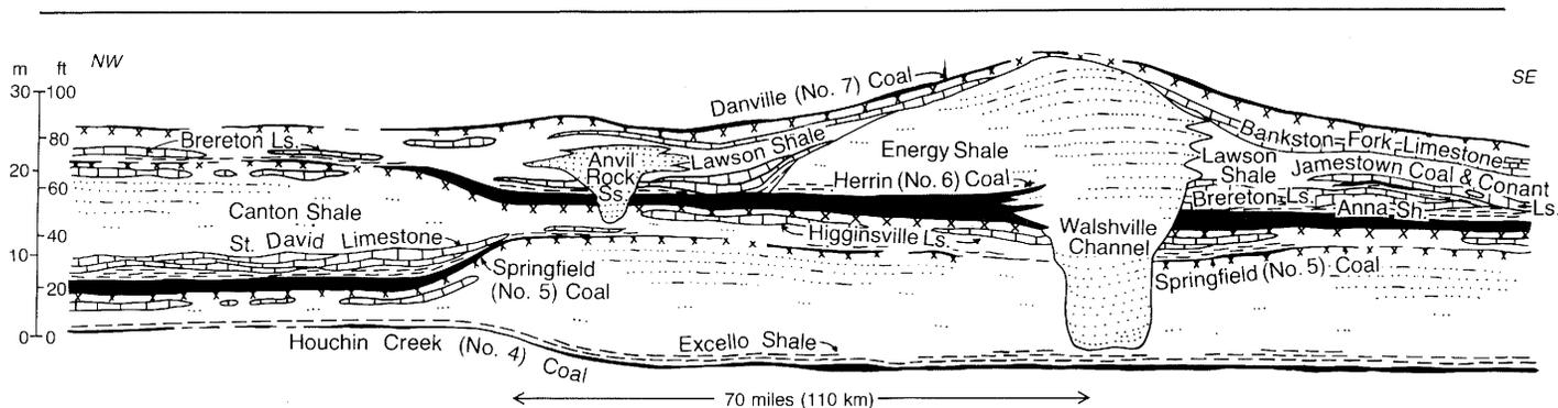
Figure 4 Generalized stratigraphic cross section of the interval from the Houchin Creek to the Danville Coal from northwestern Sangamon (left) to southeastern Montgomery County.
