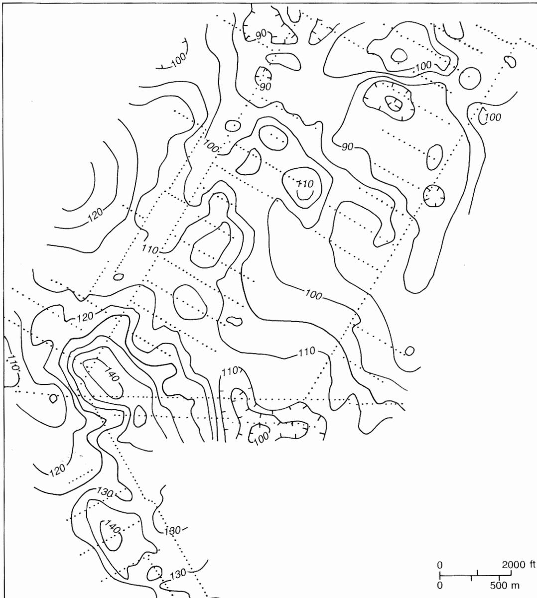
**Figure 18** Structure of base of Herrin Coal in Hillsboro Mine, T7N, R3W, Montgomery County. Contour interval is 5 feet (1.5 m). Tiny dots represent datum points from surveyed elevations along mine entries. Modified from Krausse et al. (1979).
