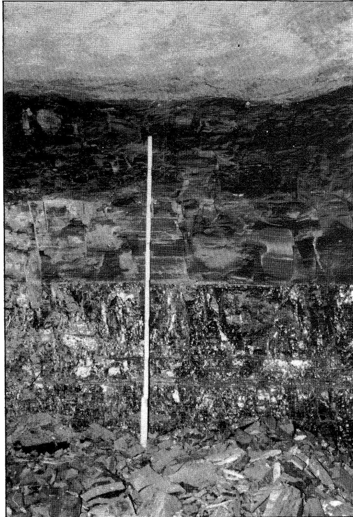
**Figure 10** Anna Shale overlain by smooth-bottomed Brereton Limestone. Lower half of Anna is hard, fissile, and well jointed; upper half is less competent and more massive. Ruler measures 4 feet (1.2 m).
