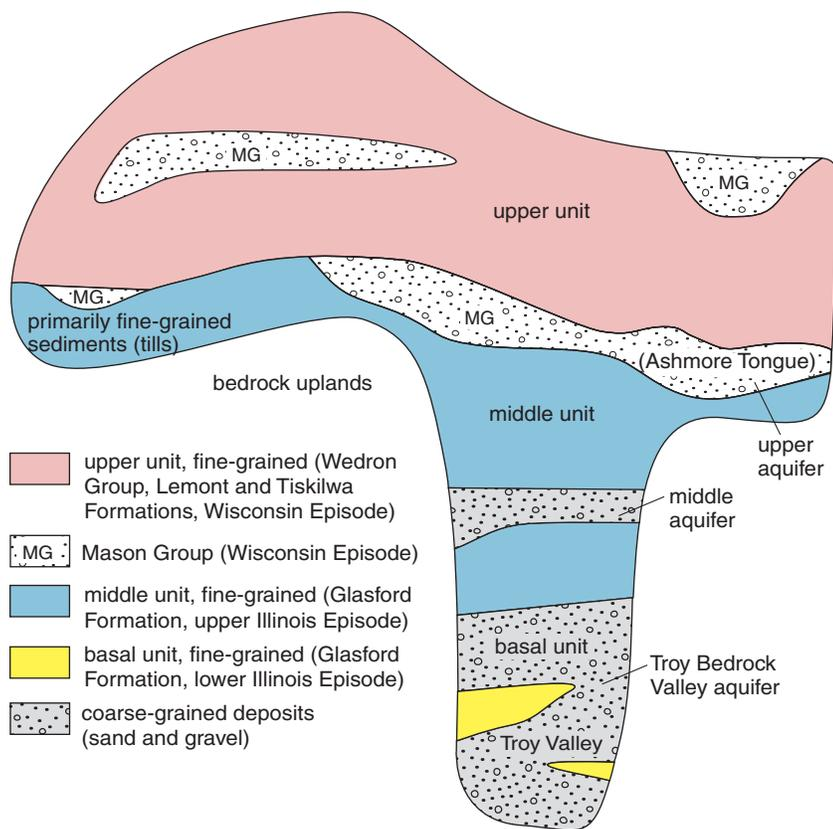
**Figure 10** Schematic diagram of glacial sediments showing their stratigraphic relationships.
