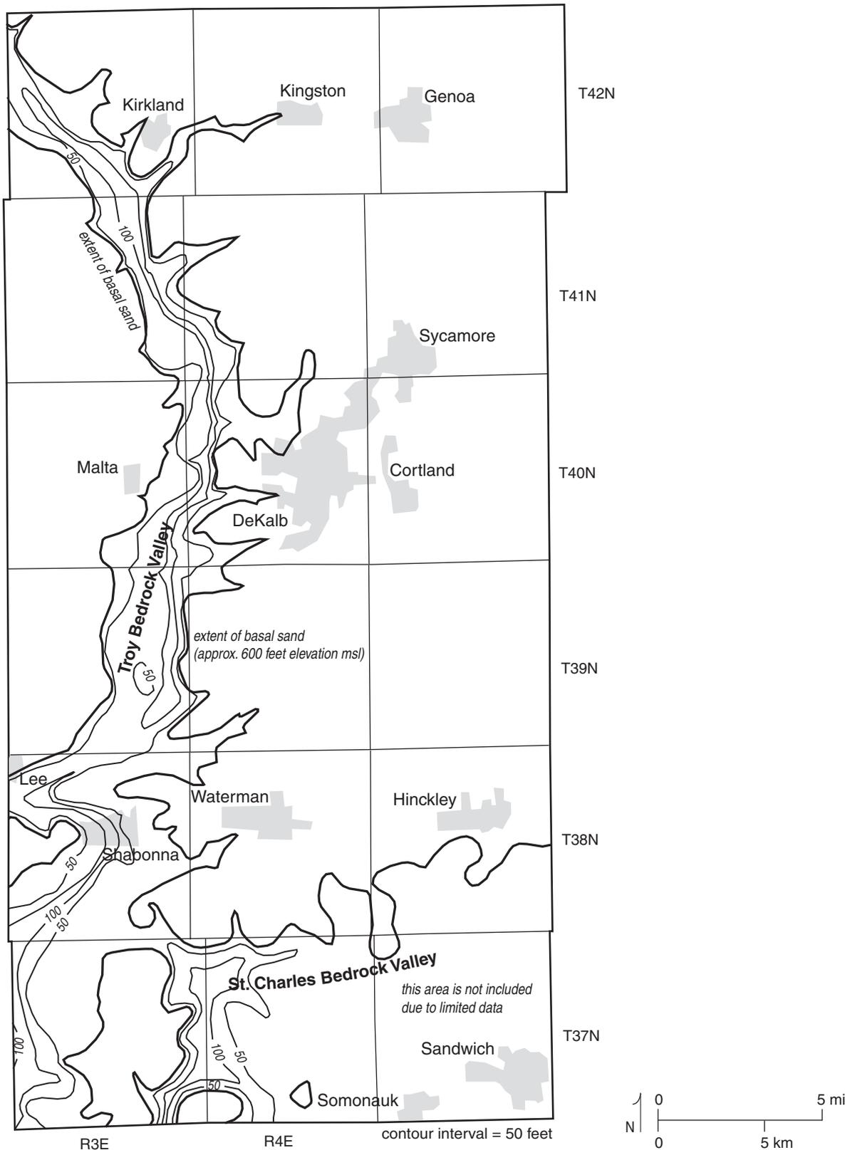
**Figure 16** Thickness of the basal sand in the Troy Bedrock Valley. msl, mean sea level.
