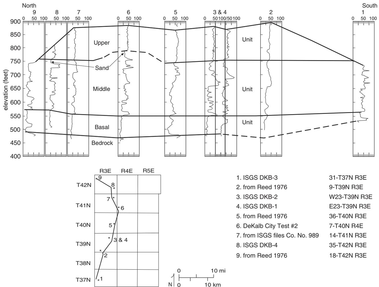
Figure 15 Down-valley geophysical log information for cross section A-A'.
