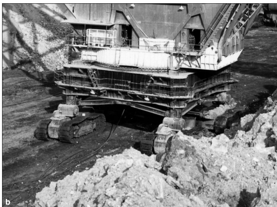
Figure 229 Peabody Coal Company, River King Mine, near Freeburg, St. Clair County. This is a view of the same mine shown in Figure 227, but from the other end of the pit. This Bucyrus-Erie wheel excavator is removing the unconsolidated overburden and depositing it far behind the active face of mining, which prevents the waste material from sliding back down into the pit onto the coal that is being removed. The detail shown in the enlargement (b) illustrates the supporting framework for this massive machine.
