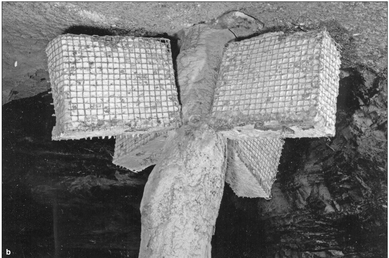
Figure 156 Old Ben Coal Corporation, No. 15 Mine, near West Frankfort, Franklin County. Another approach to rock dust safety that Buchanan and Jones tried was to fill wire baskets with dust. The force of an explosion would knock the dust out of the baskets and disperse it to quench the flame. In a humid mine, the dust might not disperse as predicted (Ledvina et al. 1992).
