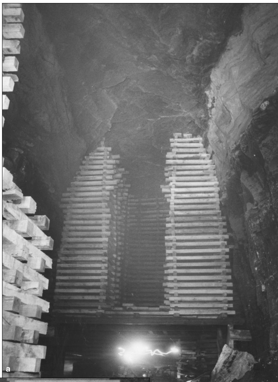
Figure 146 Peabody Coal Company, No. 10 Mine, Christian County. (a) These stacked timbers are called “cribbing.” The roof fall shown here was about 35 feet high, and the coal here was up to 13 feet thick. (b) The enlarged portion shows the steel I-beams that support the cribbing and the size of one of the blocks that has fallen from the roof (ISGS Coal Section mine notes).
