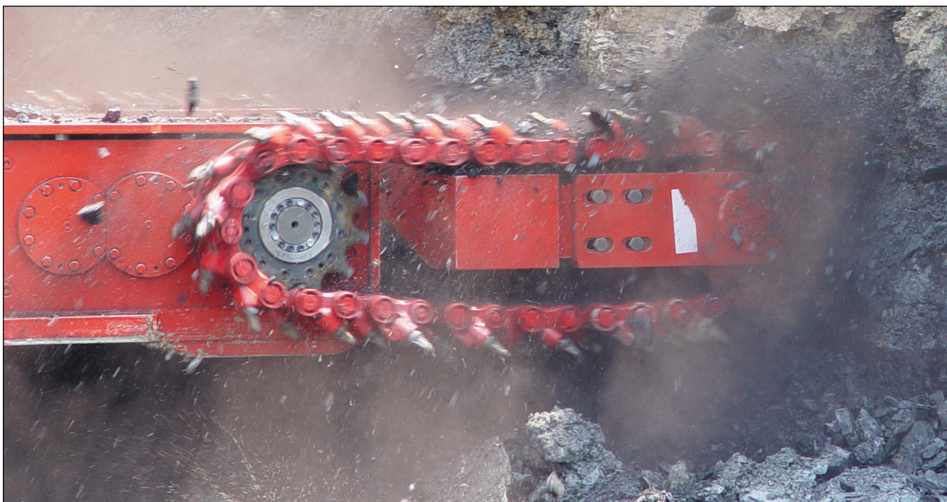
Figure 275 Knight Hawk Coal, LLC, Creek Paum Mine, Jackson County. The ripping-type continuous miner portion of the Superior Highwall Miner progressing into the seam. A chain conveyor in the center of the cutting head gathers the coal and sends it back to the augers in the pushbeams.
