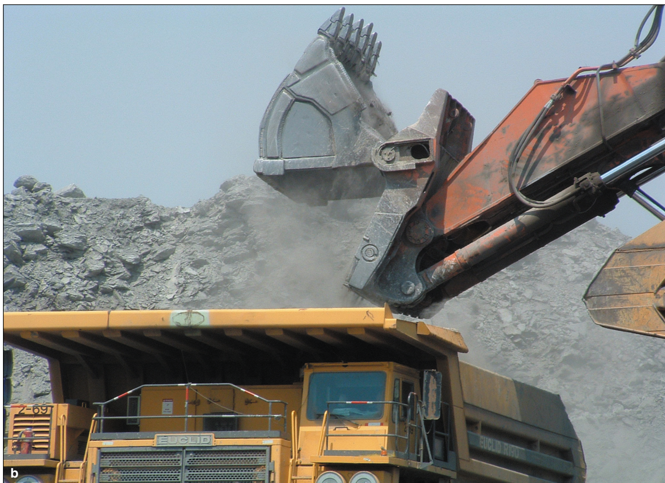
Figure 268 Vigo Coal Company, Wabash County. The Hitachi EX3500 loading shovel in the background (a) has a novel method of dumping, lifting the bucket away from its base (b). The protective canopy on the haul truck is also shown (b). In the rush to load, the shovel operator may overshoot the bed of the truck, but with the reinforced canopy above the truck operator, any damage is minimized.
