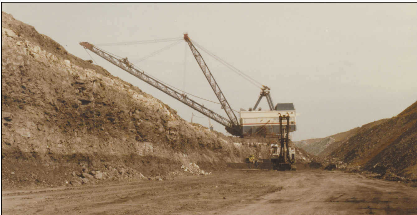
Figure 249 Arch of Illinois, Inc., Captain Mine, Perry County. This Bucyrus-Erie Model 2570-W dragline had a 105-cubic yard bucket on a 325-foot boom. Bucyrus-Erie sold 27 of this model after it was introduced in 1973 and later upgraded the model to a super dragline, designated by the WS extension, with larger buckets and longer booms (Haddock 2001).
