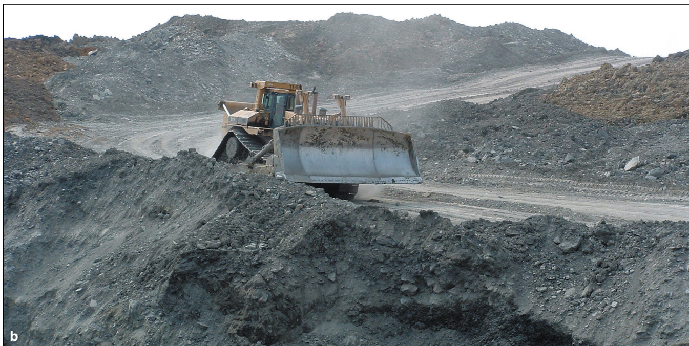
Figure 269 Vigo Coal Company, Wabash County. Construction and maintenance of haulage roads out of the pit is a major enterprise. The slope is dictated by the power of the trucks; switchbacks are inserted so that no segment will exceed the allowable slope.
