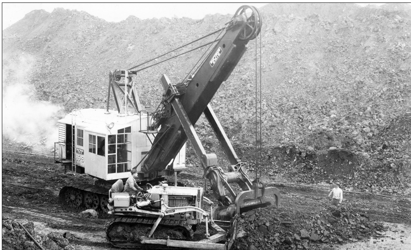
Figure 202 Little Sister Coal Company, Little Sister Mine, near St. David, Fulton County. Bucyrus-Erie 5-cubic yard 85-B loading shovel (Williamson and Myers 1955) and Caterpillar Diesel bulldozer with Bucyrus-Erie blade working in tandem.
