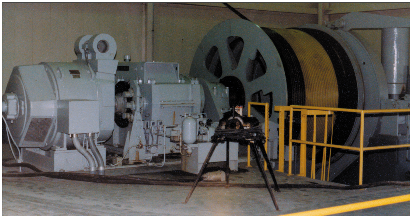
Figure 11 Freeman United Coal Company, Orient No. 4 Mine, Williamson County. The hoisting engine and cables for the No. 3 Portal for this mine. Earlier versions of hoisting engines are shown in a later part of this report.
