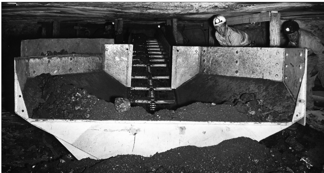
Figure 74 Mine and location unknown. A coal transfer point for secondary haulage in a mine is shown.
