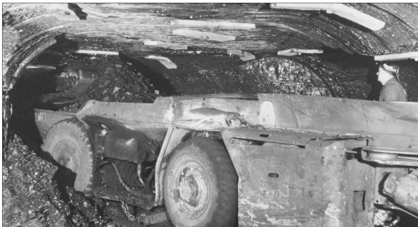
Figure 91 Bell & Zoller Coal Company, No. 3 Mine, Zeigler, Franklin County. This shuttle car or buggy is being loaded behind a boring-type continuous miner. The tail (conveyor) of the miner is discharging coal into the shuttle car. The boring machine was pioneered mostly by Old Ben Coal Corporation, but contributions were made by Freeman United and Zeigler Coal Companies as well. The last boring machines were taken out of service in the mid-1980s (Ledvina et al. 1992).
