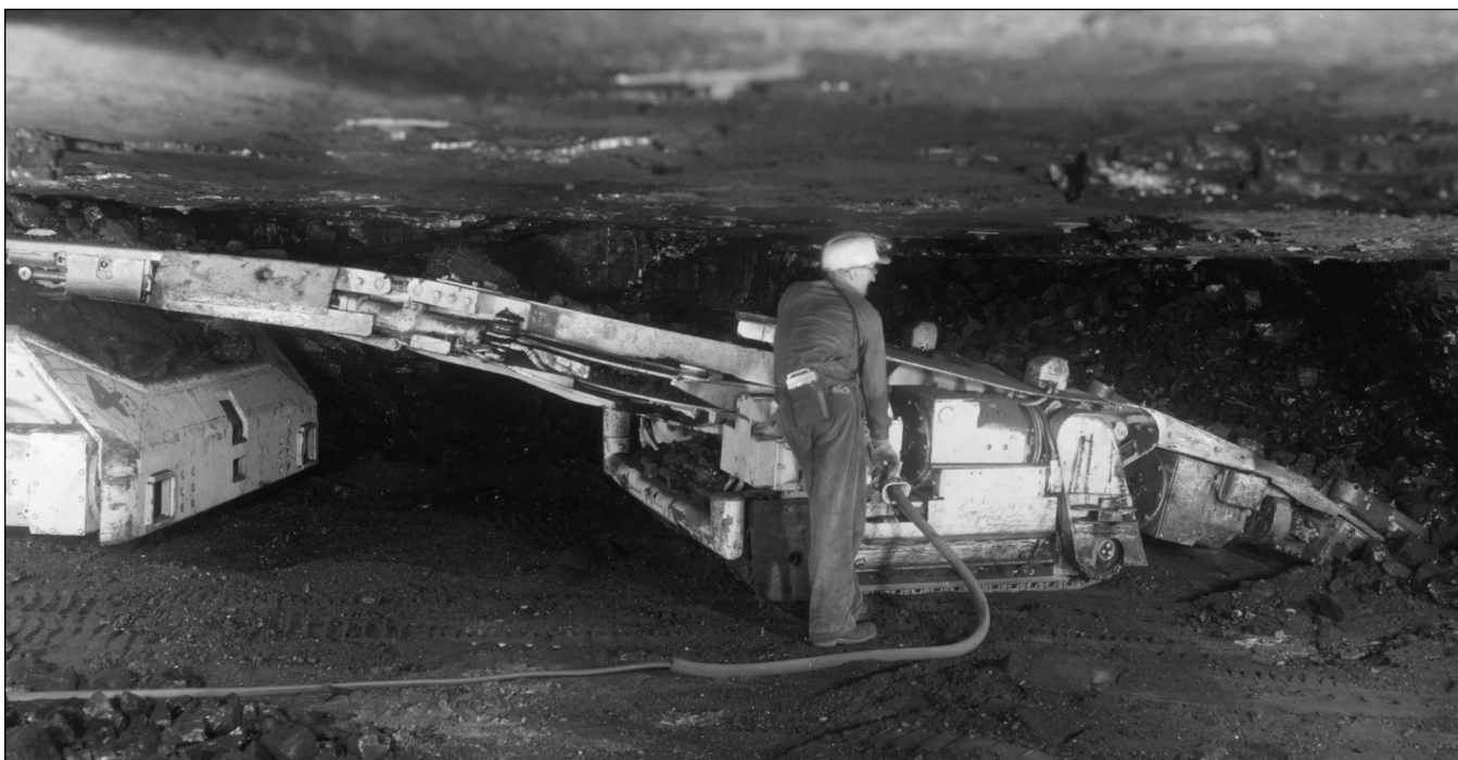
Figure 59 Mine and location unknown. A few roof bolts with metal plates support the roof where this loader is working. The loader has a gathering chain with teeth that brings the coal into the center conveyor and then loads the shuttle car (to the left, mostly out of the photograph). Most loaders could move 10 tons per minute or more, and the capacity of coal movement was limited more by the shuttle cars than by the loader speed (Jeffrey Manufacturing Company undated).
