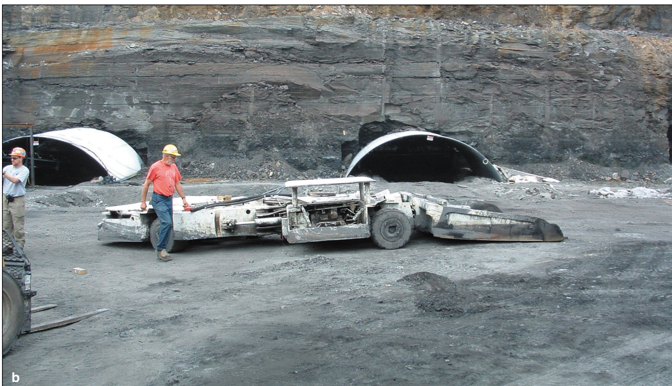
Figure 273 Illinois Fuels Company, LLC, I-1 Underground Mine, Saline County. Drift mines go directly into the coal from the surface without the need for a shaft to get down to the level of the coal. (a) The timbers on the left support steel I-beams that in turn support the roof. The machine shown in photograph (b) is a scoop tram, similar to a front end loader. This low-profile vehicle has an open bucket on the front, with a ram to aid unloading by pushing the coal out the front again when it is stopped at a coal transfer point. Other techniques for underground mining are described more fully in the previous section of this report.
