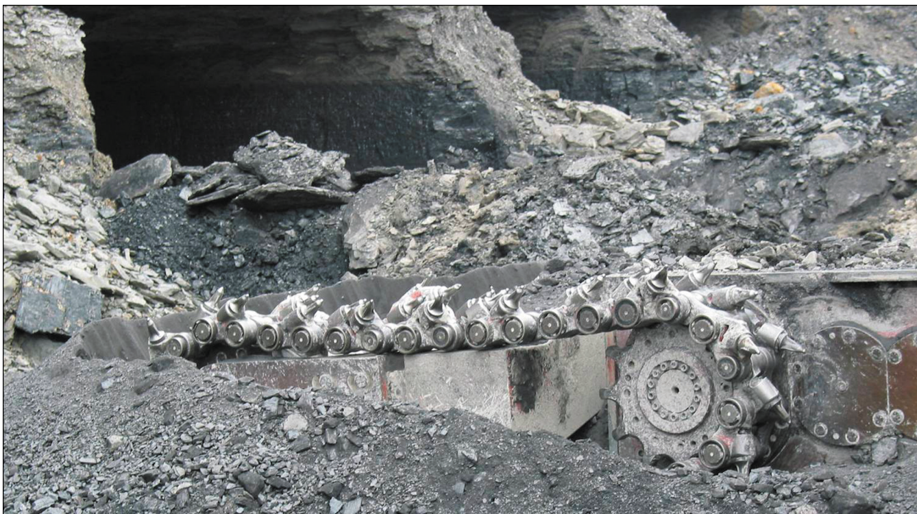
Figure 276 Mine and location unknown, Ohio. This photograph shows the distinctive rectangular opening made by the ripping-type continuous miner. The Superior Highwall Miner precisely monitors position to keep the continuous miner properly aligned so that the designated pillar width is left between excavated rooms.
