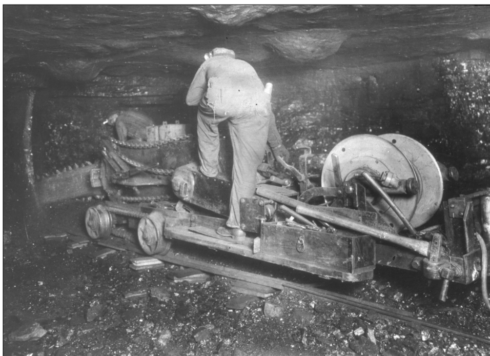
Figure 33 Peabody Coal Company, No. 5 Mine, Pawnee, Sangamon County. A vertical shearing machine cuts the coal so that blasting can loosen it from the face more effectively. In mines with a weak roof, top cutting was also done to protect the roof from the effects of the blast (Malesky 1973). The roof in this photograph shows protrusions from the roof, called limestone bosses, which are very hard on bits in coal cutting machines.
