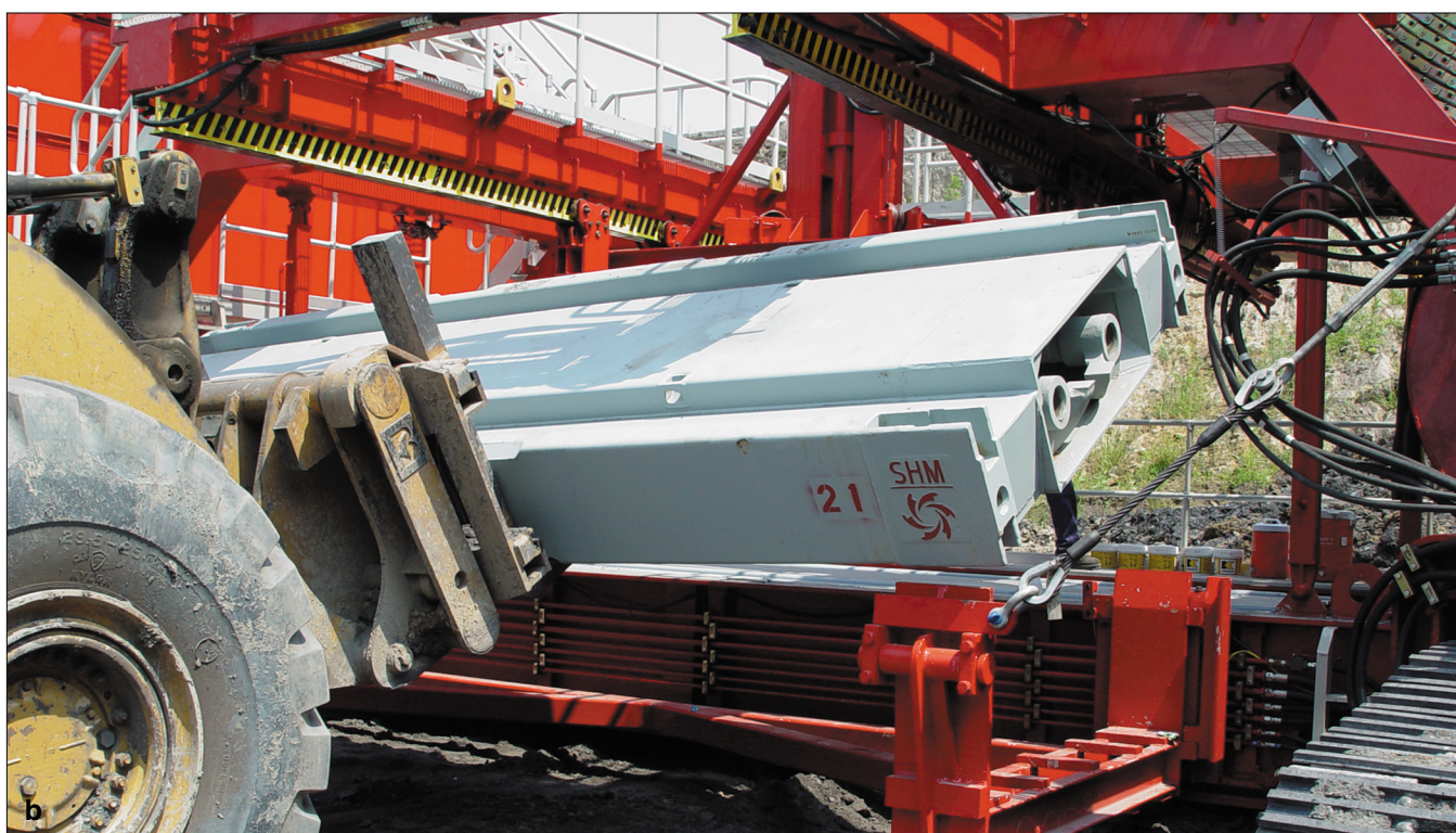
Figure 274 Knight Hawk Coal, LLC, Creek Paum Mine, Jackson County. The Superior Highwall Miner deploys a continuous miner up to 1,000 feet into the highwall of a surface mine while the operators work above ground (Schafer 2002). Conveyors attached to the continuous mining machine carry the coal to the surface. (a) The entire miner is shown. The reel on the left contains the hose reel assembly, which holds electric power and methane sensor cables. Behind the machine are stacks of pushbeams that attach directly behind the continuous miner. The pushbeams have an internal pair of 18-inch augers to shift the coal to the conveyor belt (shown at right), which protects the coal from out-of-seam dilution, such as shale falling from the roof into the mined coal. (b) The interlocking portion of the pushbeams; this portion requires a forklift working with the highwall miner.
