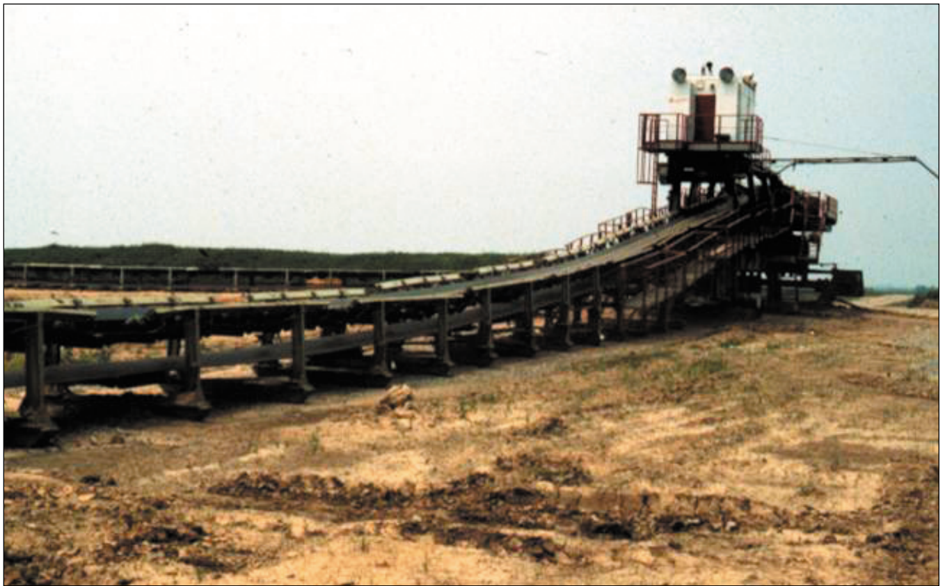
Figure 258 Arch of Illinois, Inc., Captain Mine, near Willisville, Perry County. The conveyor shows a part of the around-pit conveyor, unique in Illinois, returning empty to the wheel excavator. The belt could travel at 950 feet per minute.
