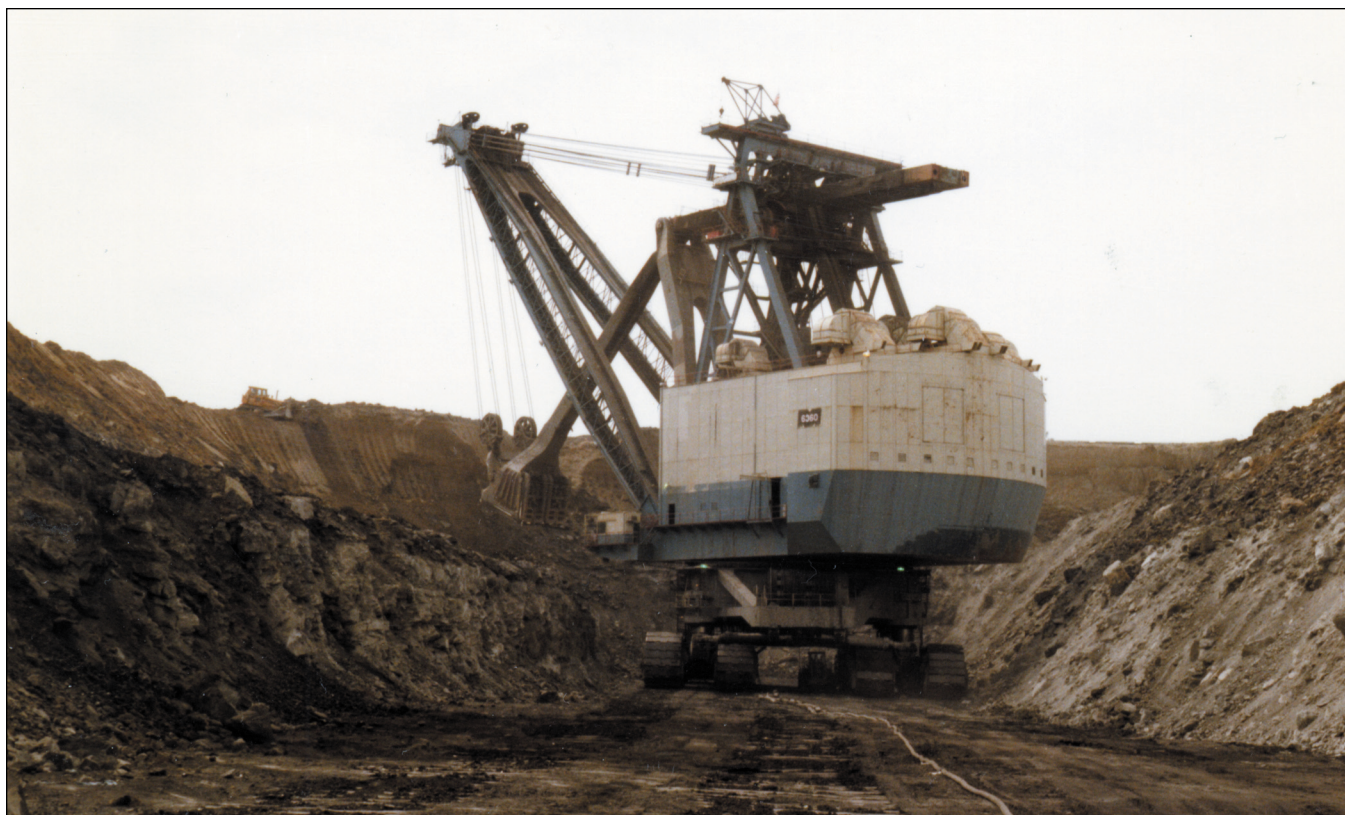
Figure 247 Arch of Illinois, Inc., Captain Mine, near Willisville, Perry County. “The Captain,” a Marion 6360 stripping shovel, was still working after 18 years.
