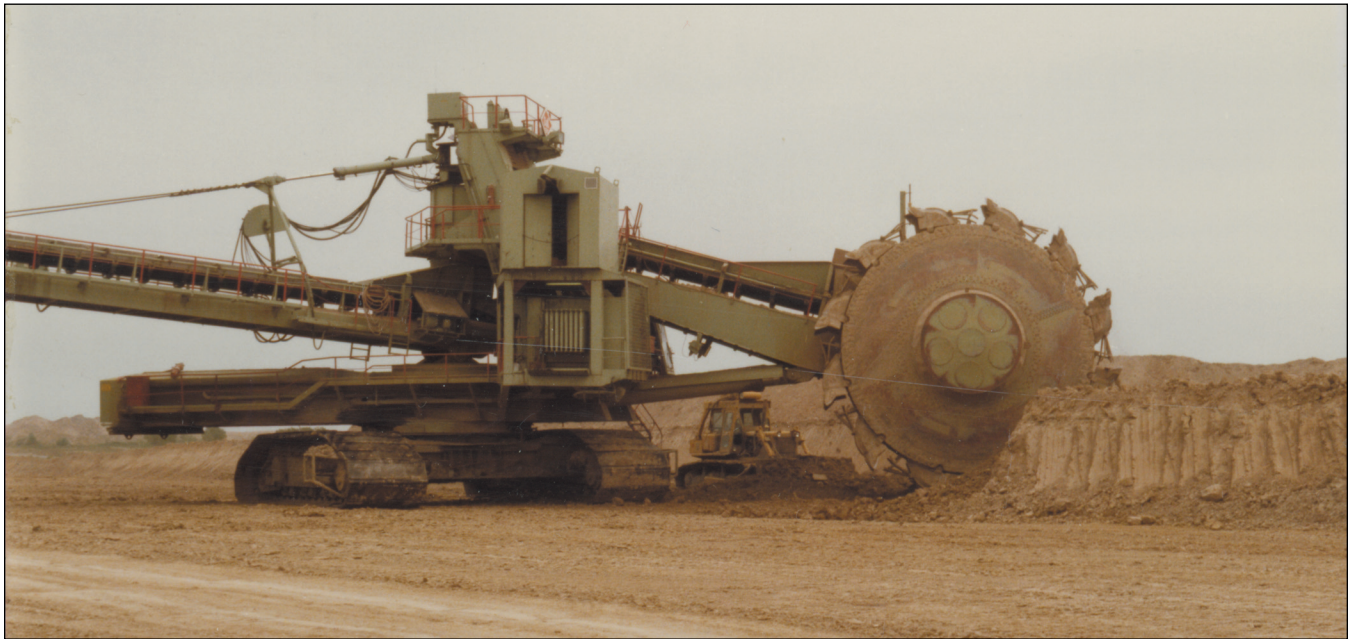
Figure 254 Arch of Illinois, Inc., Captain Mine, near Willisville, Perry County. Bucket wheel excavators were useful for reclamation because they could remove discrete layers of soil or subsoil and deposit it a much greater distance from the highwall than draglines or shovels could, which reduced the cost of reclamation. However, bucket wheel excavators could only be used for overburden that had very few rocks because rocks damaged the buckets and conveyors.
