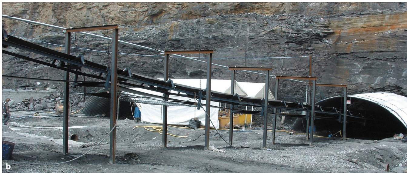
Figure 272 Illinois Fuels Company, LLC, I-1 Underground Mine, Saline County. The most common manner of accessing deep coal off the highwall in Illinois was to open a drift mine and work the coal in the usual underground mining pattern. The corrugated metal arches shown in the photographs protect people and equipment near the opening from rocks falling from the highwall. Photograph (b) shows the conveyor carrying the mined coal out of the mine.
