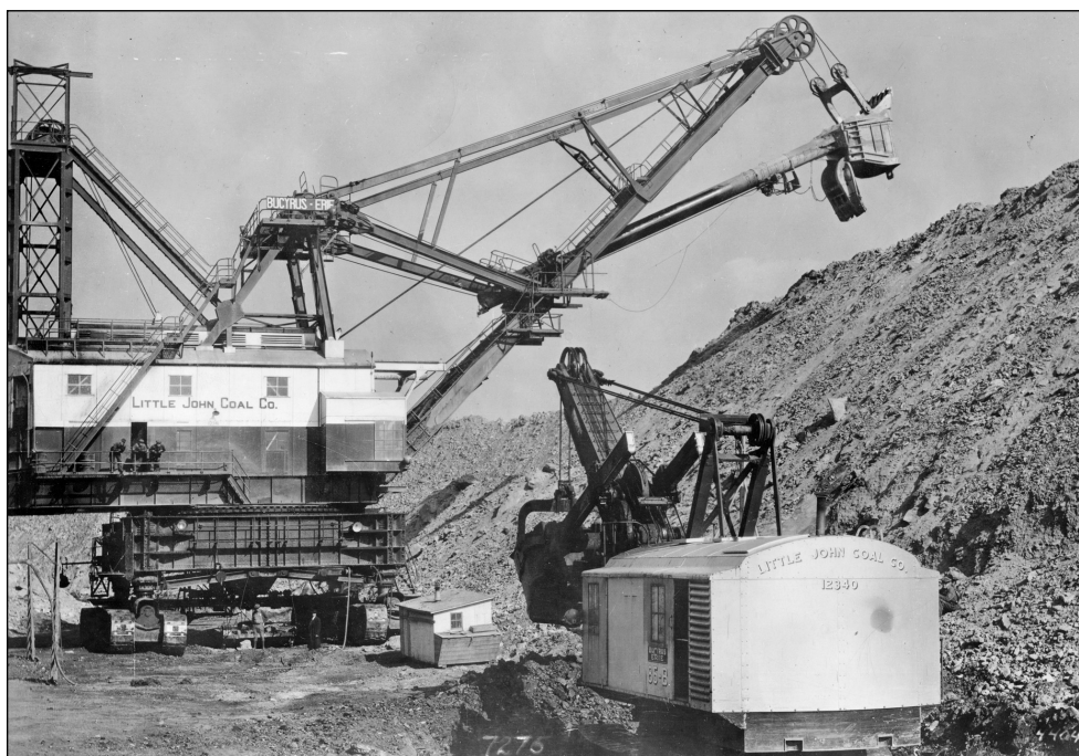
Figure 208 Fairview Collieries Corporation, Flamingo Mine, Fulton County. Bucyrus-Erie 950-B stripping shovel shown at work. This photograph shows the counterbalanced hoist mechanism at the rear of the housing very clearly.
