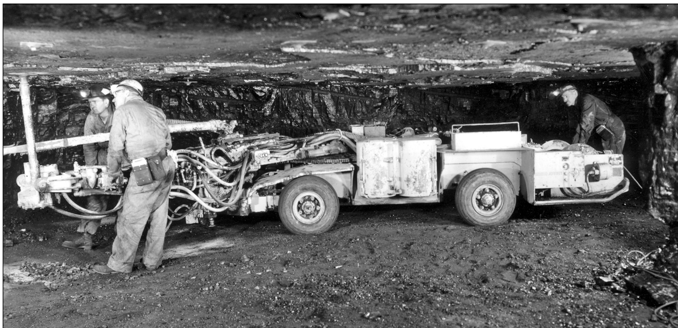
Figure 142 Mine and location unknown. The later roof bolting machines, such as this Jeffrey Model 261 in the 1950s, included an extendable boom (retracted in photograph) and remote operation (Ledvina et al. 1992).
