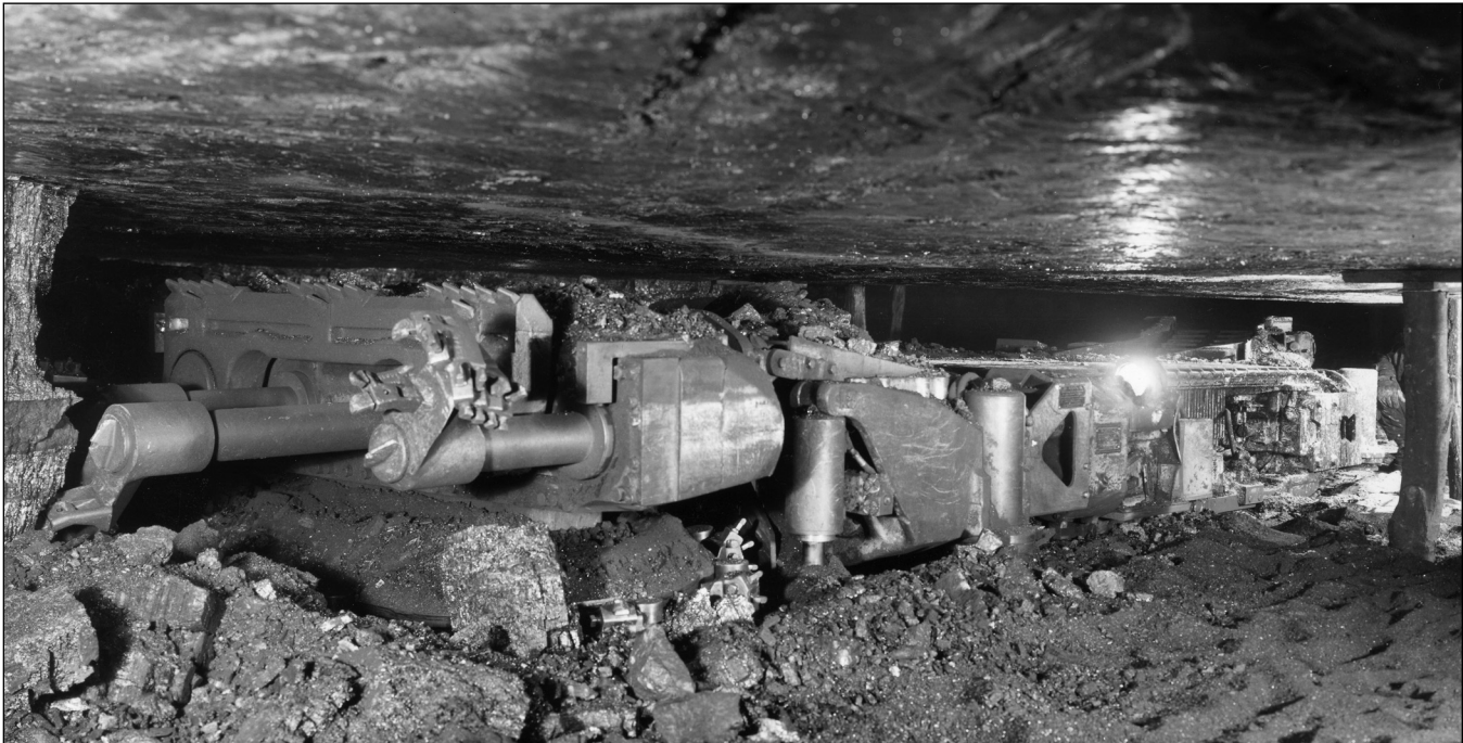
Figure 80 Mine and location unknown. A Jeffrey Colmol-type continuous miner is shown. The cutting heads, called breaker arms, are shown in the left foreground. Below the breaker arms are gathering chains that collect the coal to the center of the machine where it is conveyed behind the machine. At that point, a conveyor belt system or shuttle car can transport the coal from the face. The cutting head can move straight ahead, but also to the left and right for greater versatility. These machines came in a variety of heights to mine thin or thick coal (Jeffrey Manufacturing Company undated). The Colmol produced less dust than did other continuous miners because the bit consisted of a drilling portion and a breaking portion (Phillips 1950).
