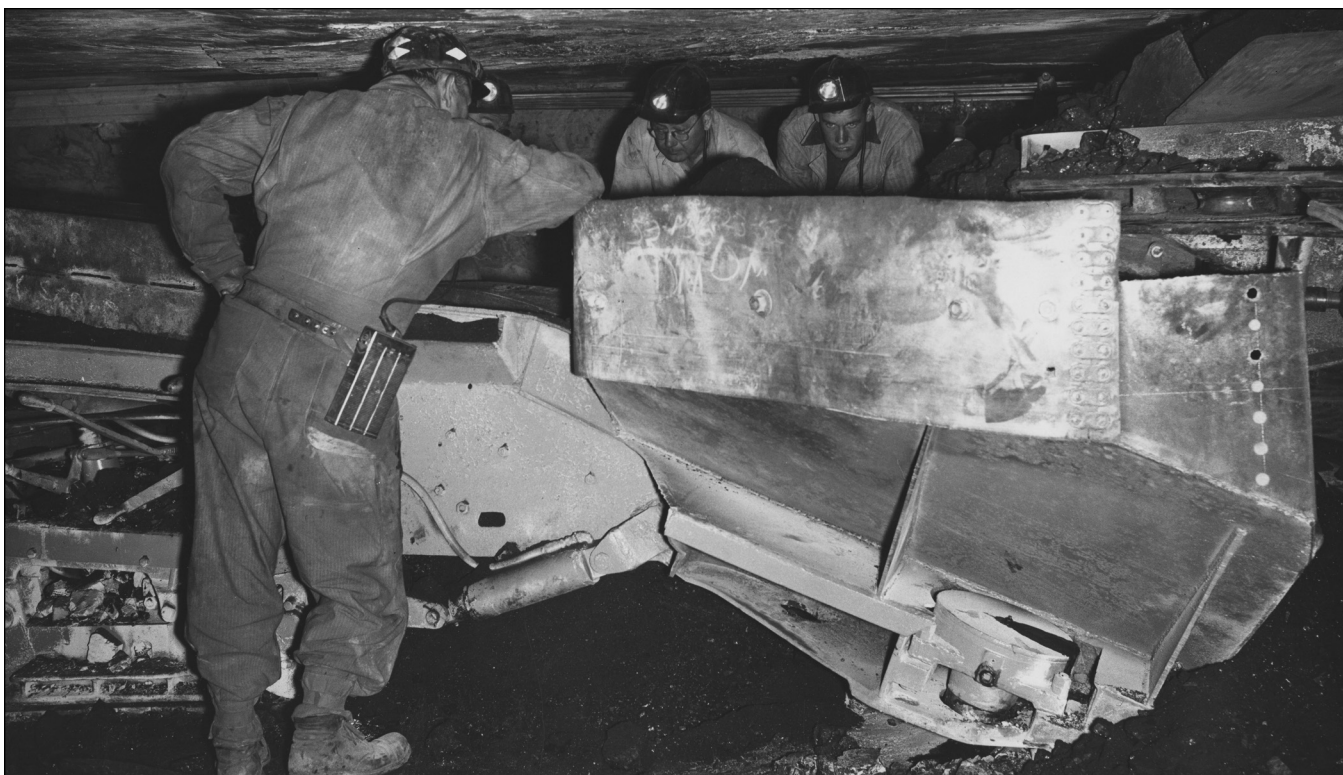
Figure 76 Sahara Coal Company, No. 5 Mine, Saline County. Shuttle buggy (mostly off picture at the right) discharging coal into a company designed transfer pickup (a redesigned loading machine) that transfers coal from the discharging buggy onto the rubber belt (Ledvina et al. 1992).
