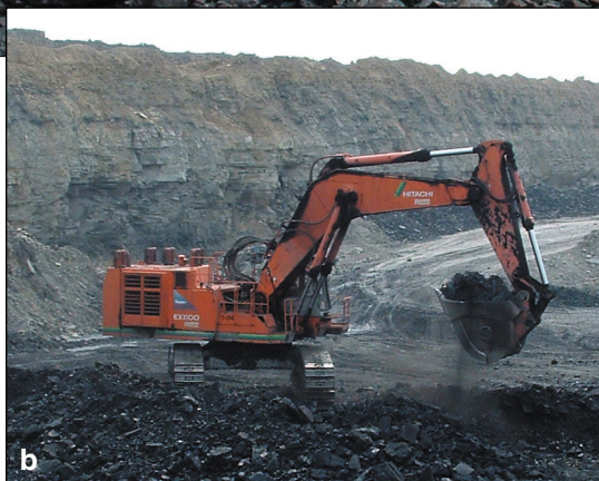
Figure 267 Vigo Coal Company, Wabash County. (a) This caterpillar loading shovel is one of three types used at this mine. (b, c) The Rudd-Hitachi EX1100 loader has a versatile bucket that swings 180 degrees.
