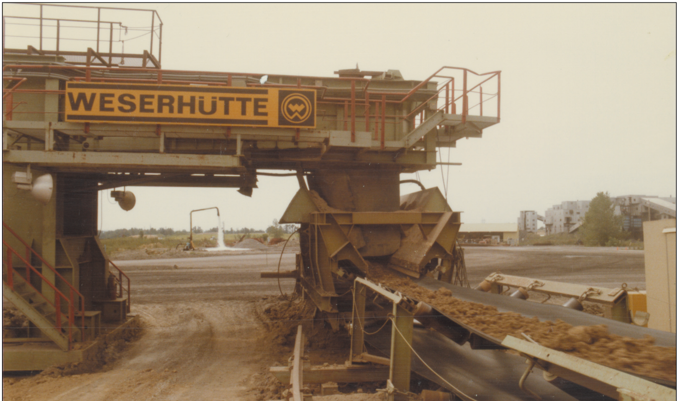
Figure 255 Arch of Illinois, Inc., Captain Mine, near Willisville, Perry County. This conveyor transported subsoil dug by the bucket wheel excavator. These Weserhütte conveyors transferred material from the wheel excavator to the around-pit conveyor system. The belt for the around-pit conveyor was almost 2 miles long.
