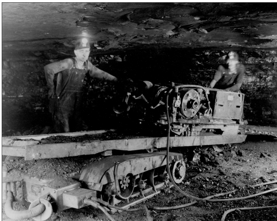
Figure 32 Bell & Zoller Coal Company, No. 1 Mine, Zeigler, Franklin County. This Joy under-cutting machine was crawler mounted and undercut wide- or narrow-faced rooms. The cutting head swiveled from side to side, which made this machine very versatile. The addition of rubber tires would have made this machine similar to modern cutters (Ledvina et al. 1992).
