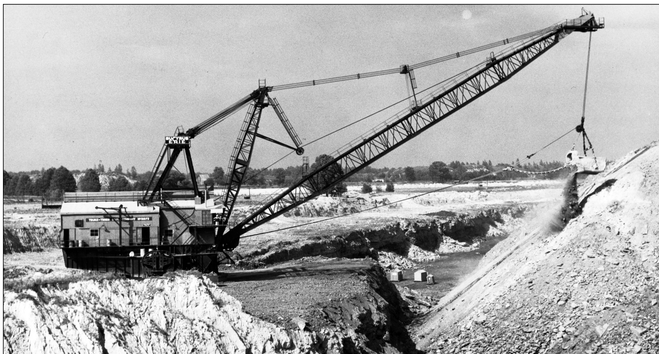
Figure 220 (below) Truax-Traer Coal Company, Burning Star Mine, near DeSoto, Jackson County. This Bucyrus-Erie walking dragline, probably an 1150-B, deposits spoil from the highwall to the other side of the pit (Ledvina et al. 1992). The 20-cubic yard bucket on a boom about 200 feet long did its job very well. This machine weighed 1,265 tons (Haddock 2001).
