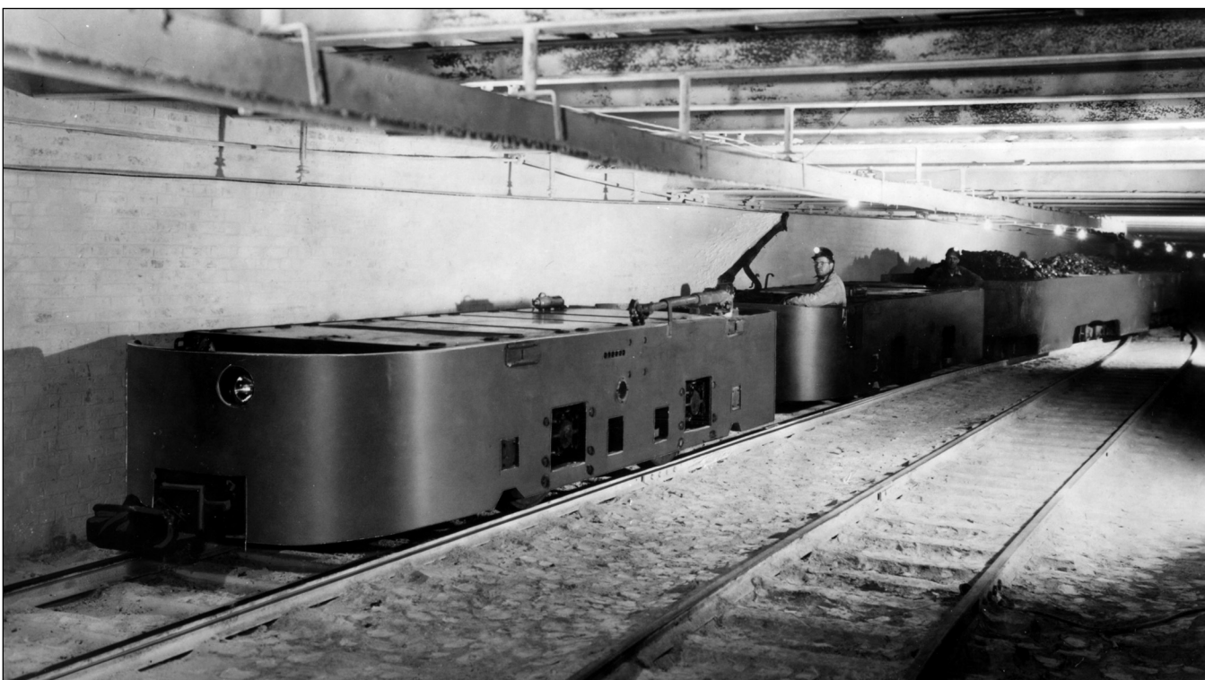
Figure 73 Mine and location unknown. These Jeffrey electric locomotives operated in tandem to pull a heavier load than one locomotive could pull alone.
