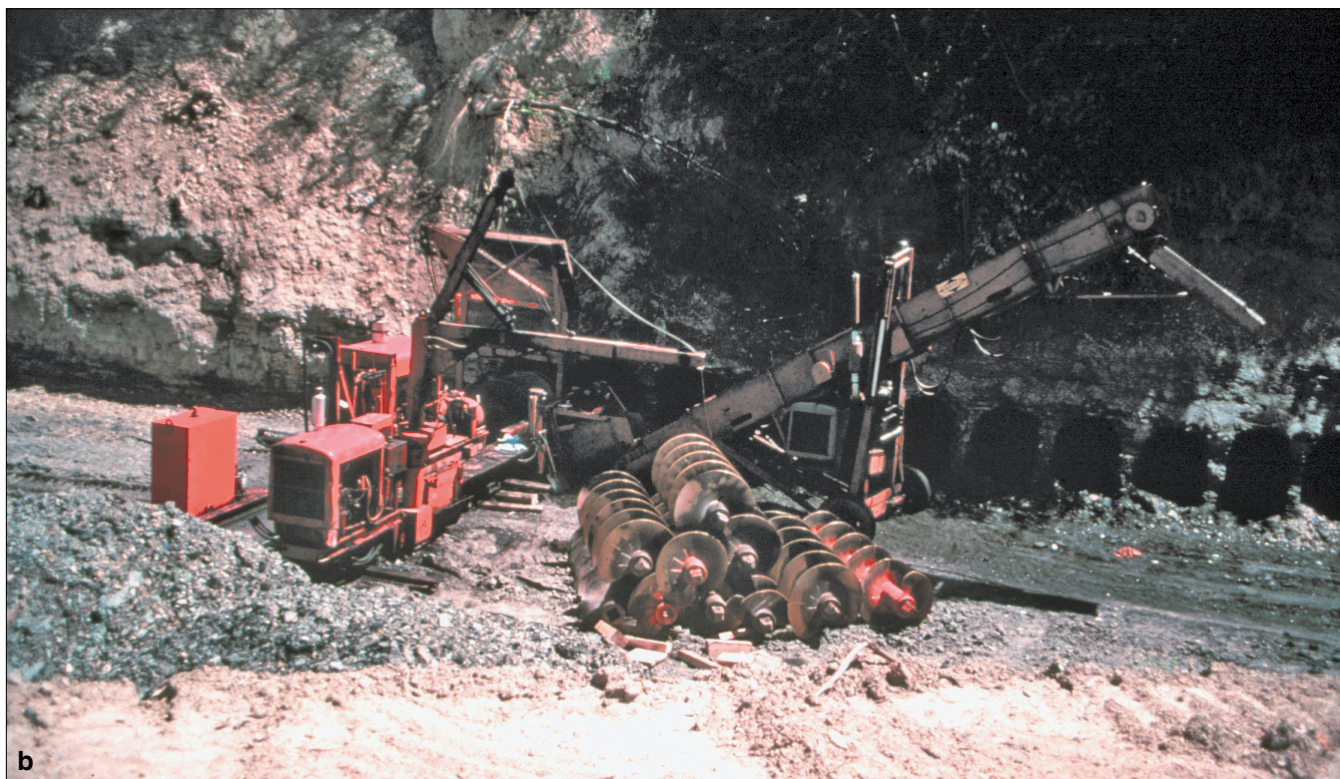
Figure 271 Lee Coal Company, Vermilion County. As photographs (a) and (b) show, little change in auger mining equipment occurred during the twenty years separating this operation from that shown in Figure 270.
