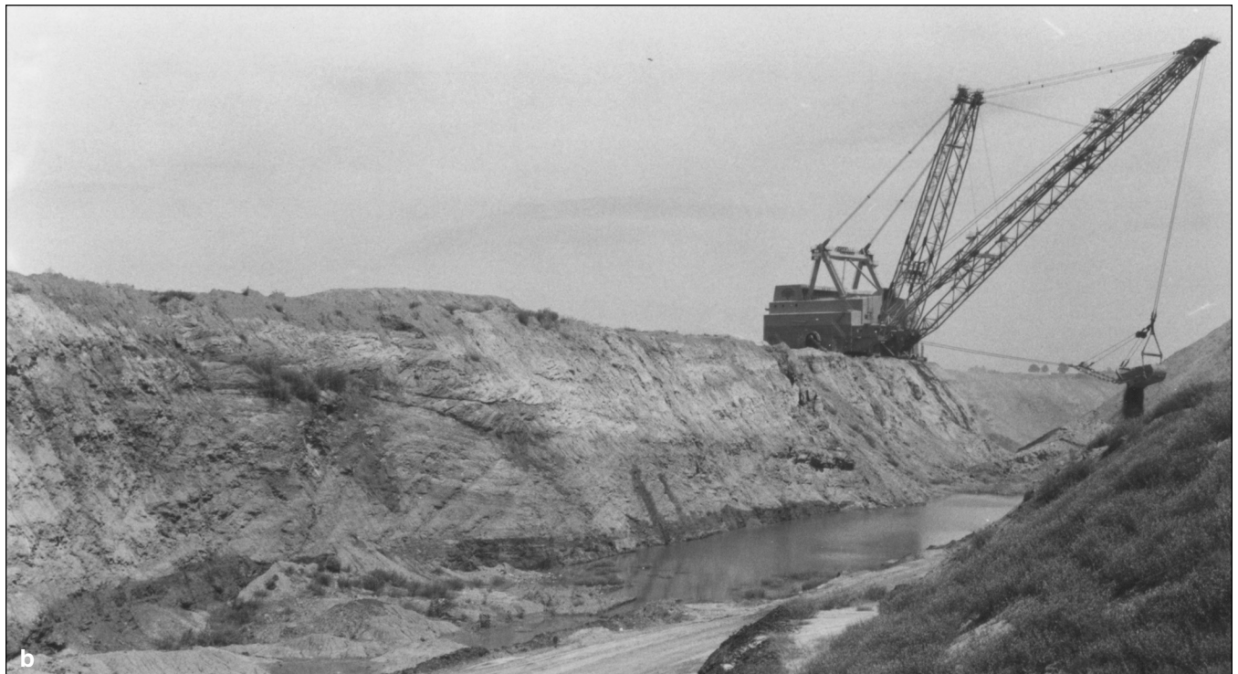
Figure 241 Consolidation Coal Company, Burning Star No. 5 Mine, Jackson County. (a,b) The Bucyrus-Erie 2570 dragline named “Big Muddy” had a 110-cubic yard bucket and a 330-foot boom. Note how close to the edge of the highwall these draglines work when the material under them is stable.
