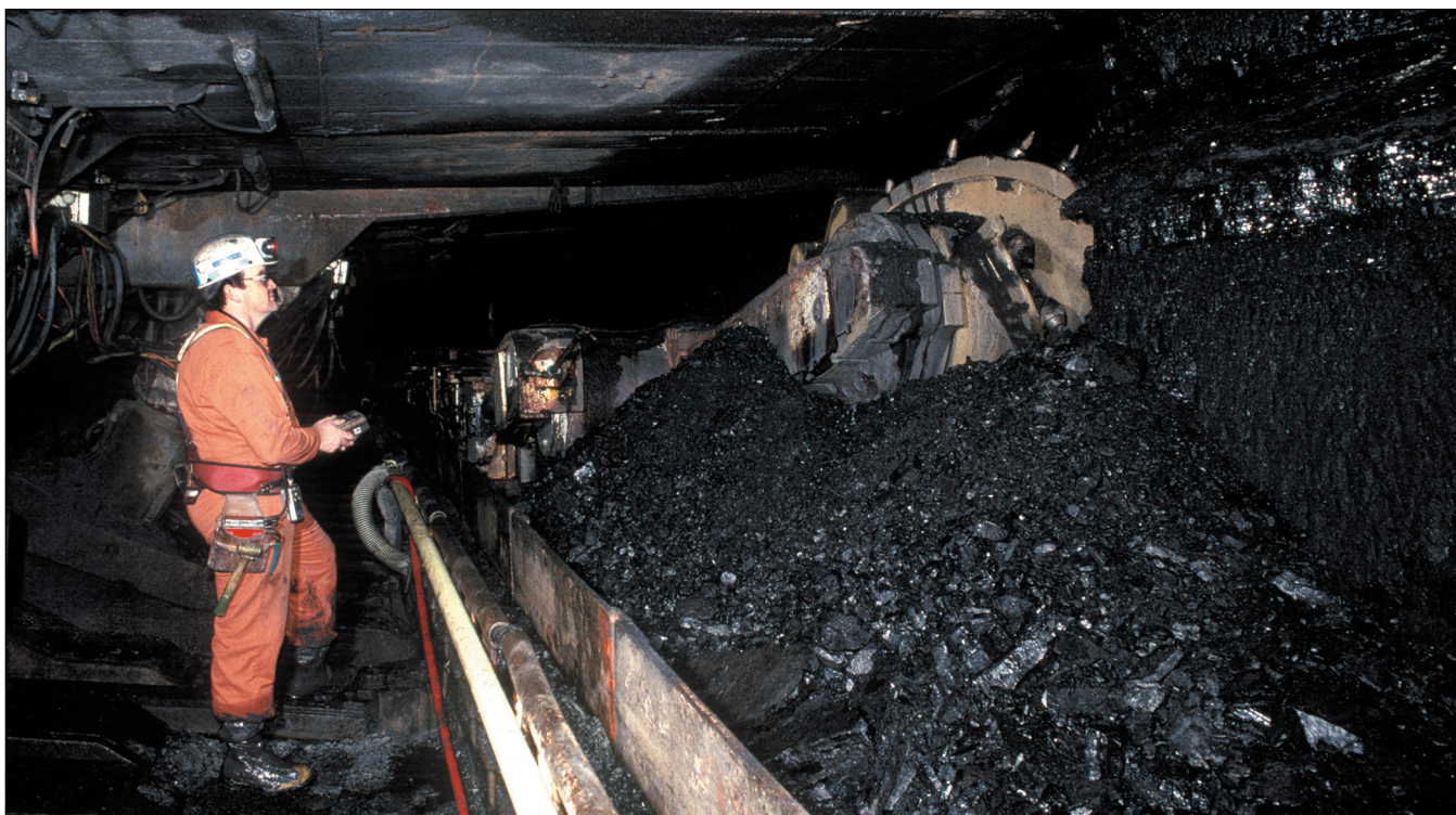
Figure 99 Kerr-McGee Coal Corporation, Galatia Mine, Saline County. Modern longwall mining is much safer for the operators who stand under the hydraulic roof shields so that rock falls are not the hazard in the longwall panel that they are in the room-and-pillar segment of the mine.
