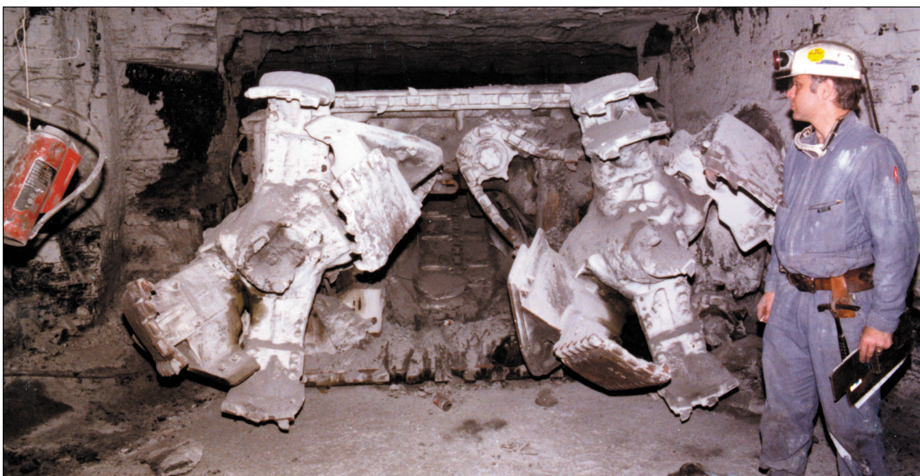
Figure 90 Old Ben Coal Corporation, No. 21 Mine, Franklin County. This Marietta boring-type continuous miner cuts a curved side wall entry. The height of the entry is determined by the height of the machine. This machine is parked in an entry mined with a ripper-type continuous miner, shown by the rectangular profile of the entry (Ledvina et al. 1992).
