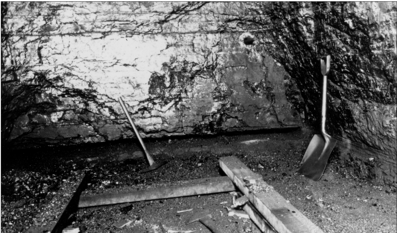
Figure 41 Mine and location unknown. The room with one shot set into a drilled hole. Shots may be fired one at a time or as multiple shots fired at once. Note the undercut coal face.
