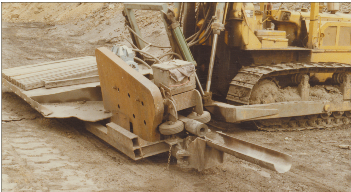
Figure 252 Arch of Illinois, Inc., Captain Mine, near Willisville, Perry County. This photograph shows the hydraulic-powered dozer attachment that loads ANFO into horizontal drill holes.
