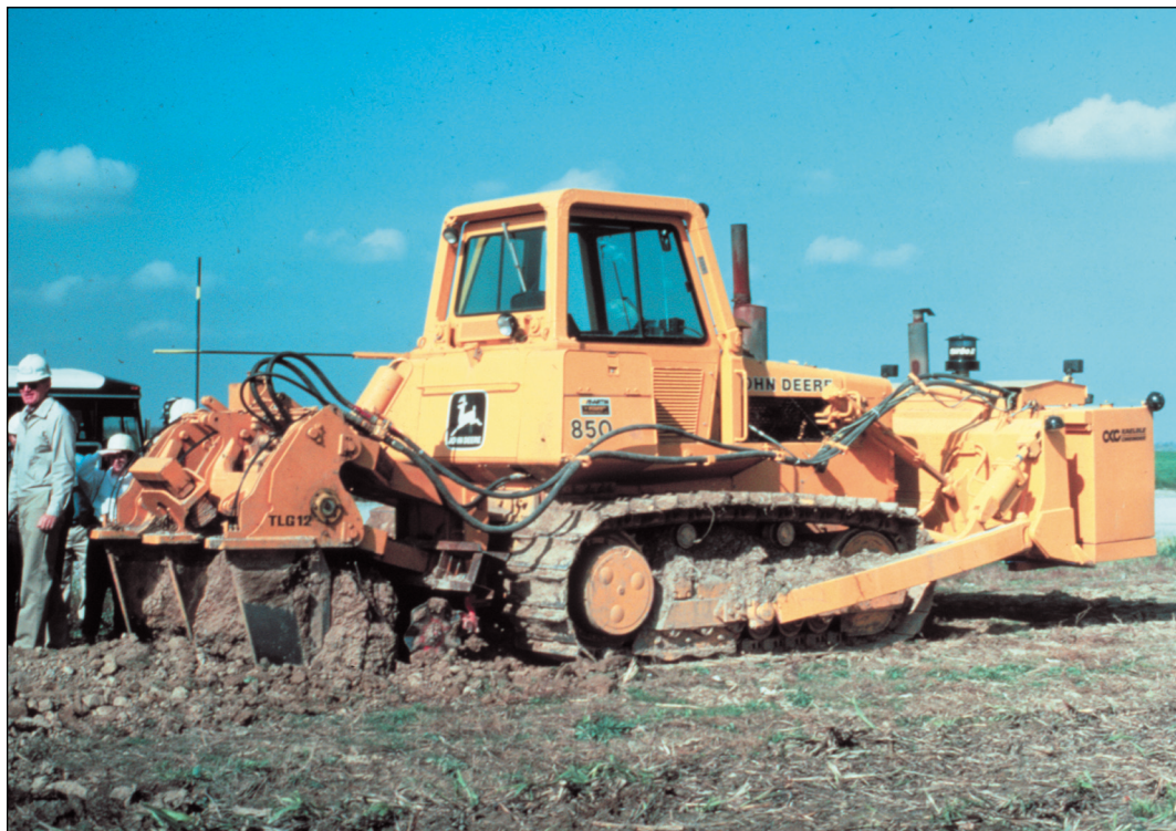
Figure 281 Arch of Illinois, Captain Mine, Perry County. With the new reclamation laws, coal companies required scrapers, bulldozers, and other equipment suitable for handling the soil layers and the more agricultural post-mining phase, as they had to show three years of productivity for prime farm land comparable to pre-mining productivity (Illinois Department of Natural Resources, Office of Mines and Minerals, undated).
