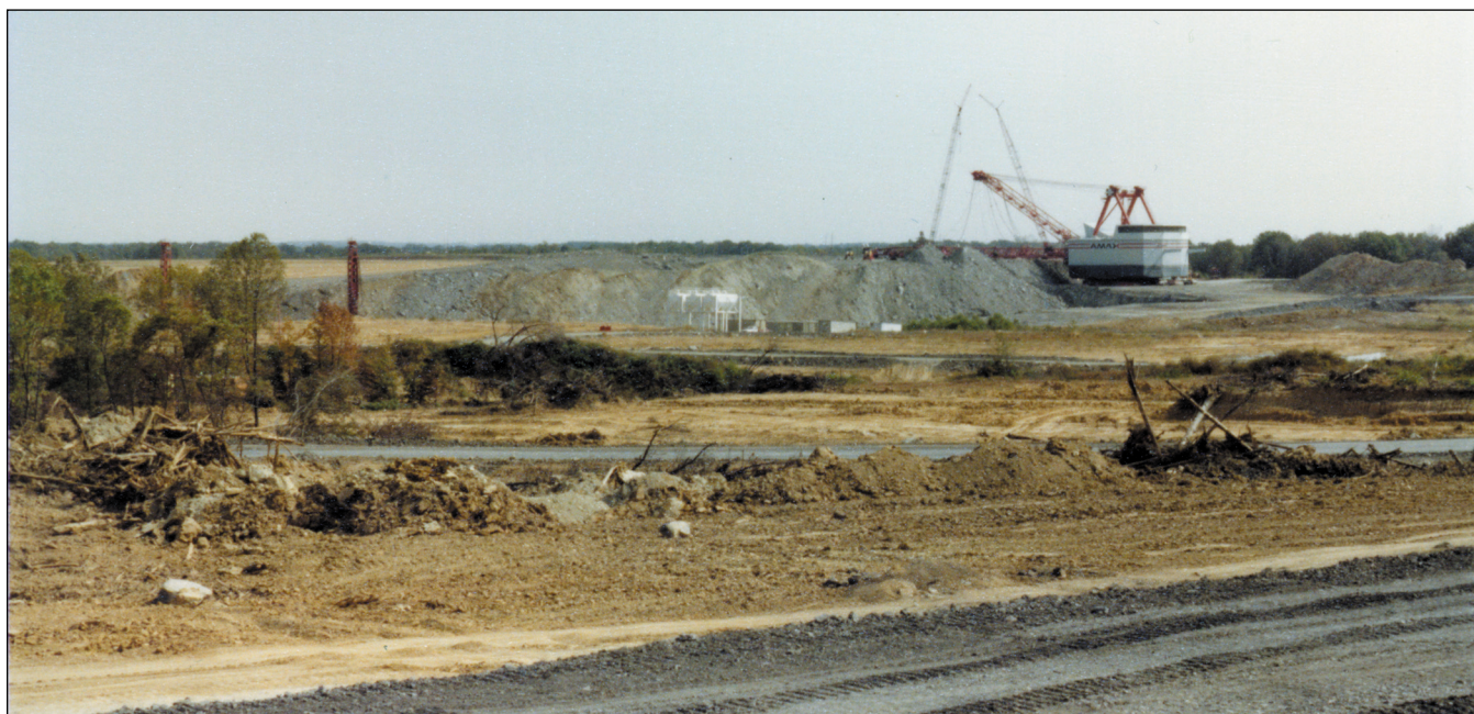
Figure 246 Amax Coal Company, Delta Mine, near Harco, Williamson County. A Bucyrus-Erie 3270-W walking dragline under construction towers over the surrounding countryside. The boom, still horizontal and supported by earth at this point of assembly, was 330 feet long. When the dragline was completed, the bucket held 176 cubic yards. The completed machine weighed 8,750 tons. Amax purchased the only two of these machines made, and they are still the second largest draglines ever built (Haddock 2001).
