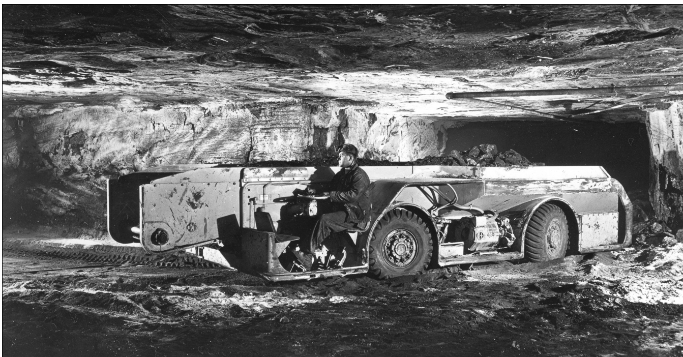
Figure 92 Mine and location unknown. Shuttle cars transported coal from the face to the secondary haulage location or collection point. The driver could face either direction with this centrally located steering wheel and dual driver seats. The conveyor for unloading is shown on the left. Many shuttle cars were electric and had to return by the same route while avoiding running over their own cable. Most were available in either AC or DC models. Turning radius and maneuverability were important factors in shuttle car efficiency (Goodman Manufacturing Company undated).
