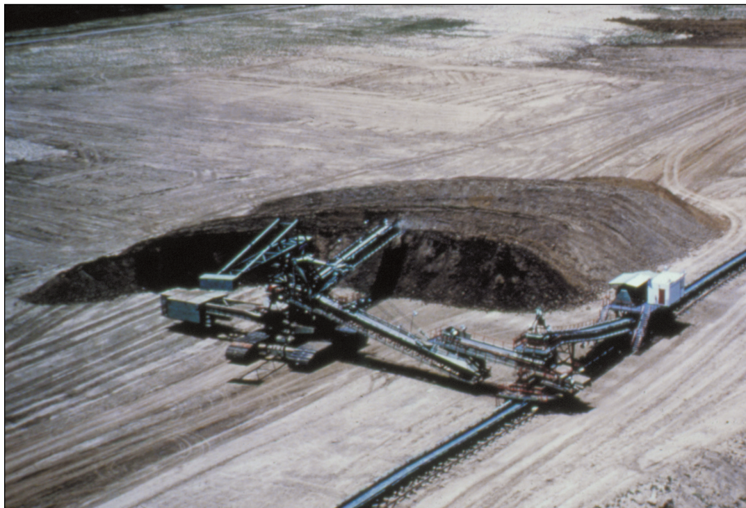
Figure 258 Arch of Illinois, Inc., Captain Mine, near Willisville, Perry County. The conveyor shows a part of the around-pit conveyor, unique in Illinois, returning empty to the wheel excavator. The belt could travel at 950 feet per minute.
