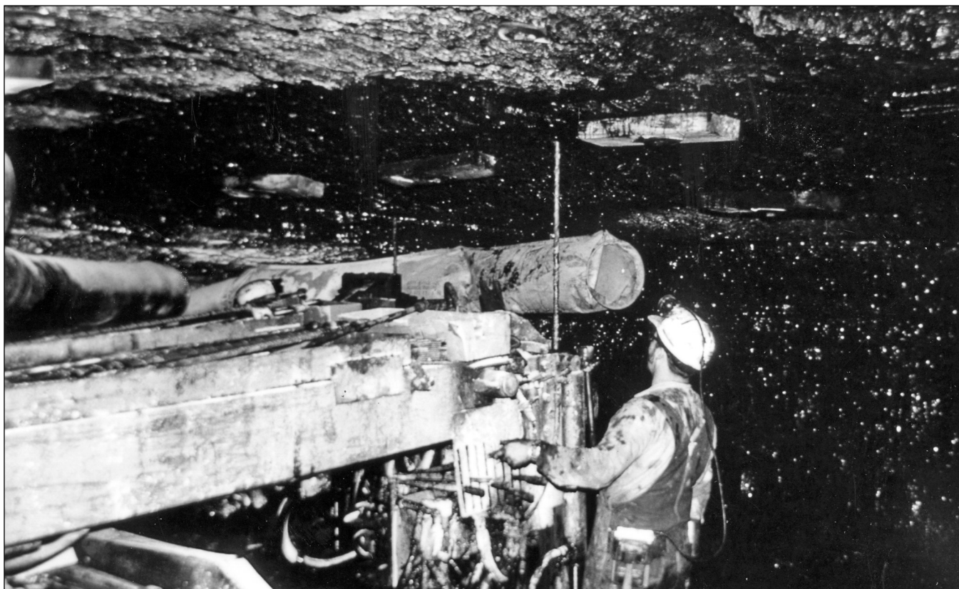
Figure 141 Inland Steel Coal Company, near Sesser, Franklin County. In thick coals with a poor roof, 1.5 to 2 feet of top coal is left to help support the roof, as shown in this photograph. In older mines, the top coal was sometimes mined on retreat just before a room was abandoned. This mine generally used 6-foot standard roof bolts and used resin bolts only in areas with bad roof (ISGS Coal Section mine notes).
