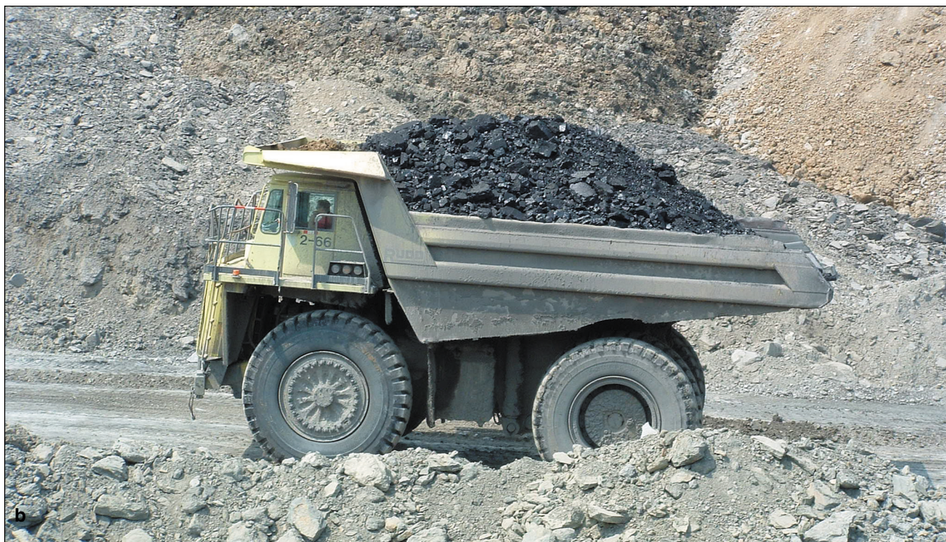
Figure 266 Vigo Coal Company, Wabash County. (a) The blocks of Friendsville Coal are shown after the machines have broken them away from the seam. This is the only location in the state where this coal has been mined. (b) A large Rudd haul truck is used to transport coal in truck-and-shovel operations.
