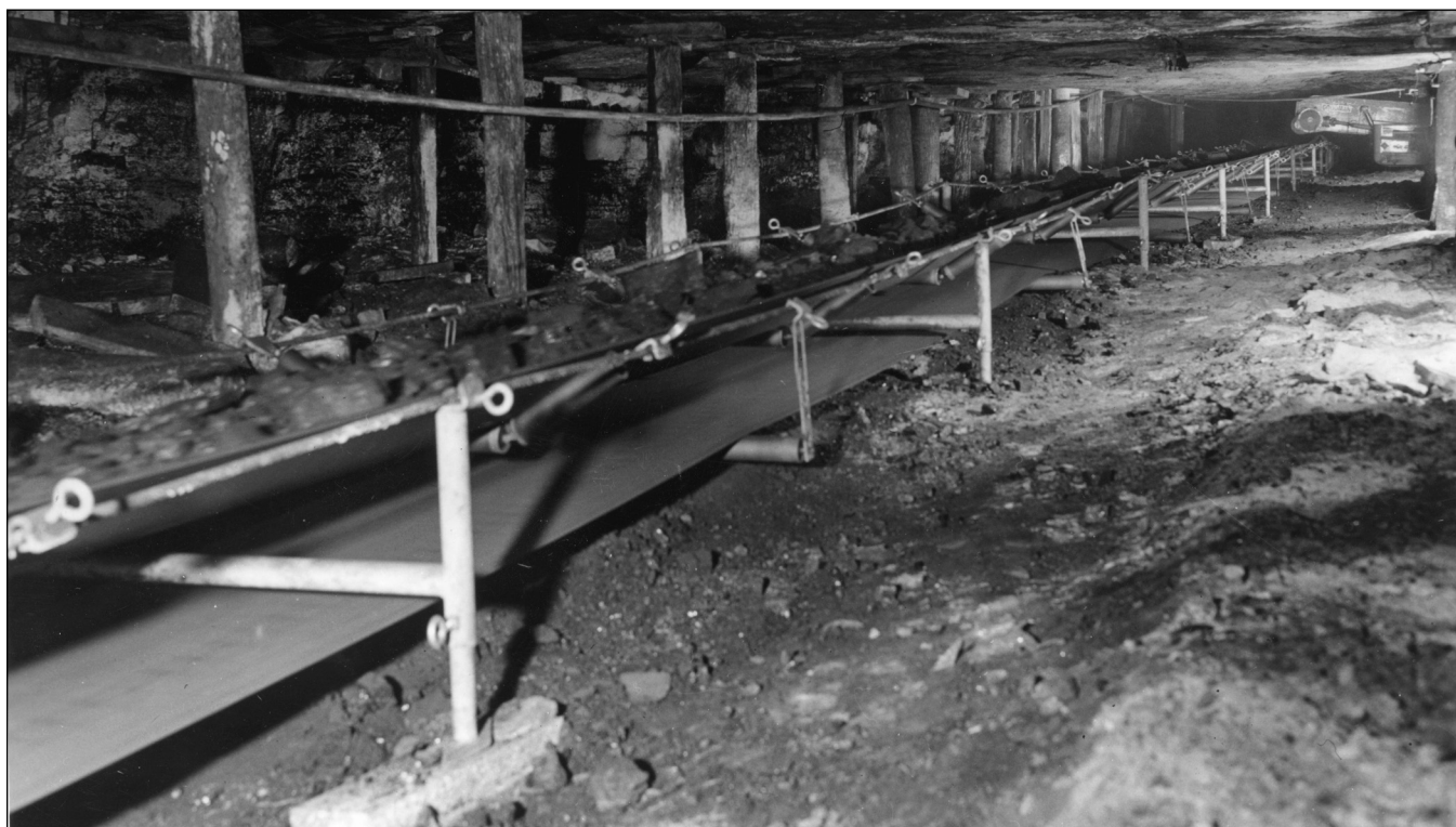
Figure 106 Mine and location unknown. Conveyor systems such as this one could be miles long and led directly to the main shaft or up the slope to the preparation plant. Later systems were developed that were mobile and could be attached directly to the continuous miner (Ledvina et al. 1992).
