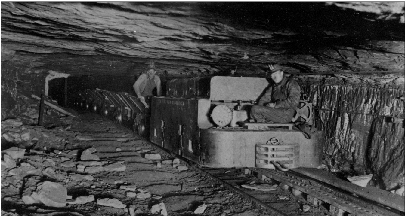
Figure 65 Mine and location unknown. As with all facets of mining, mechanization was an evolutionary process. This 30-ton rail locomotive is battery-powered, an unusual style of motor not commonly used in Illinois. Using a center gear, the locomotive meshes with the toothed center rail, enabling it to negotiate very steep grades or run on wet track with no loss of traction (Ledvina et al. 1992). The locomotive also could operate as a simple traction locomotive using only the wheels. The use of these machines was discontinued before World War I because of high maintenance costs (Beltz 1946).
