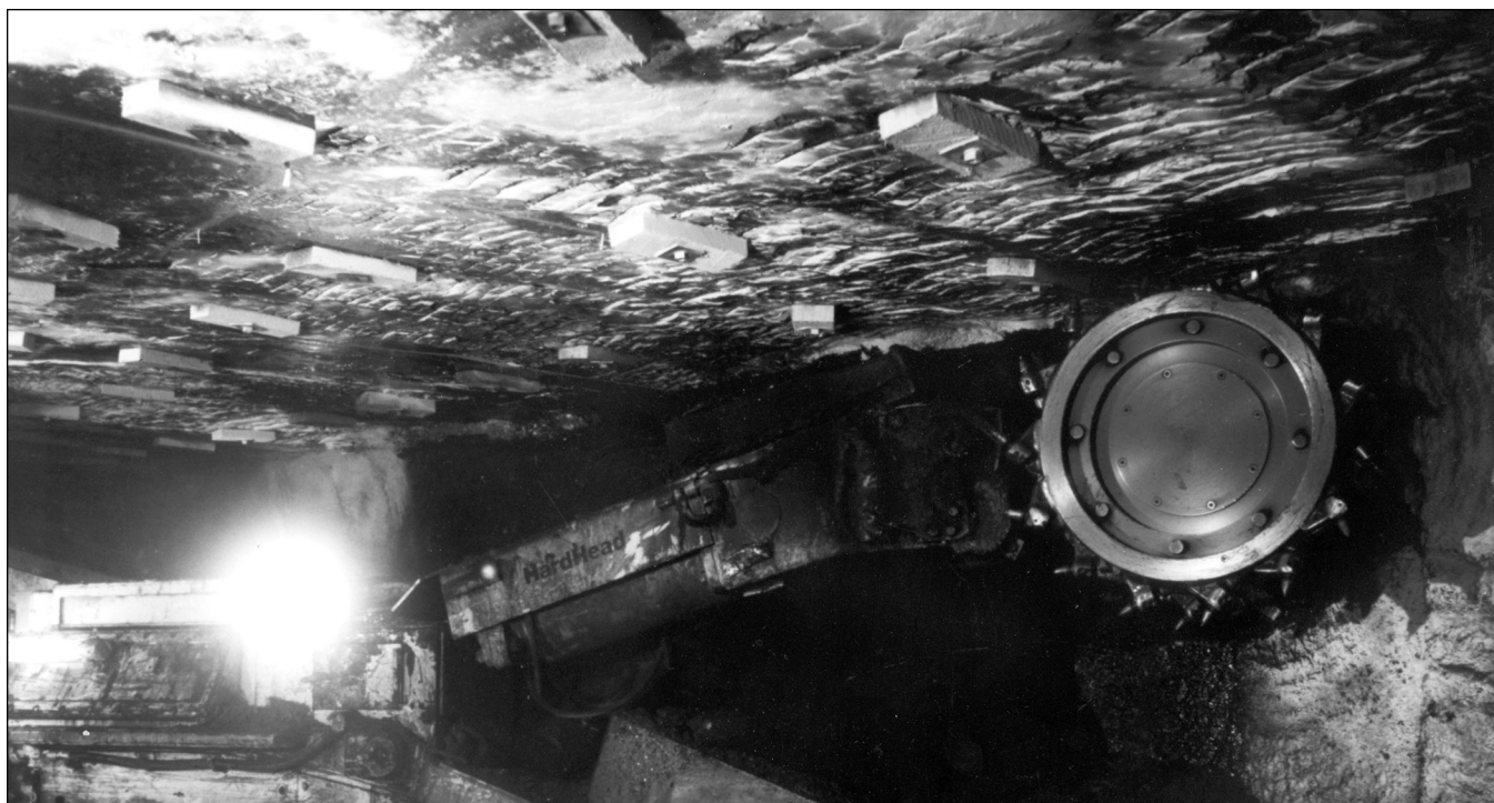
Figure 87 Mine and location unknown. Lee Norse hard head continuous miner. The Joy loading machine was eventually fitted with a series of chains or a drum to cut coal also. The drum design predominated, and the result is the truly modern continuous miner shown here. Drum-type continuous miners may have extendable or fixed width cutting heads or, in some cases, oscillating heads. This is a fixed-width type; hence, the name “hard head” (Ledvina et al. 1992).
