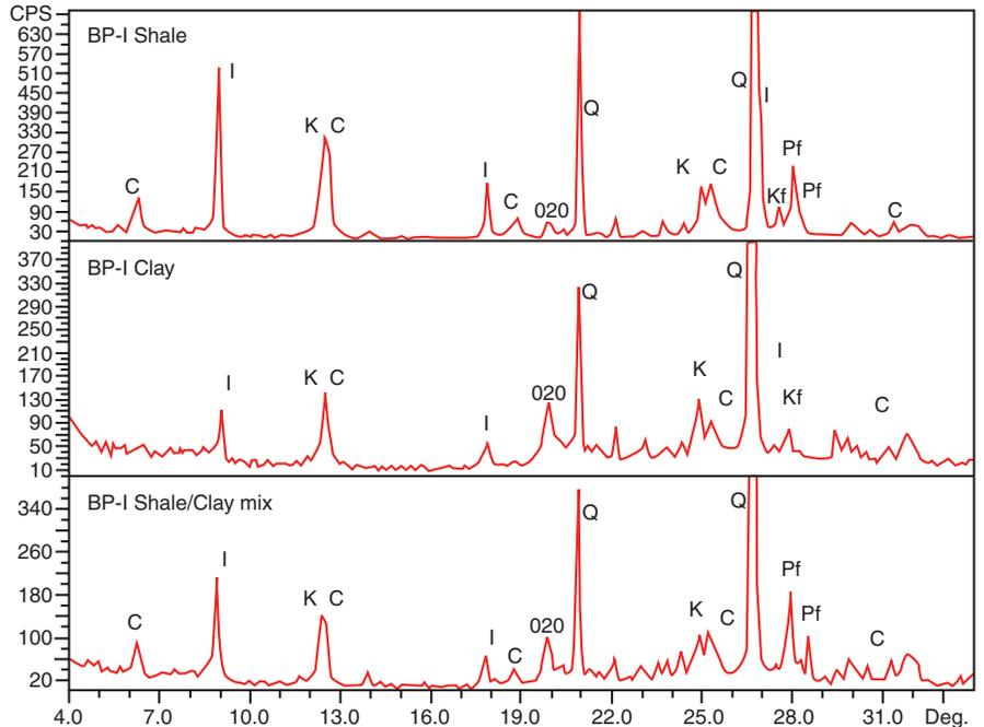
**Figure 2** X-ray diffractograms of random bulk pack of Brick Plant 1 shale, clay, and clay and shale brick mix. The mineral peak indications are chlorite (C), illite (I), kaolinite (K), (020) peak (common to all clay minerals), quartz (Q), K-feldspar (Kf), and plagioclase feldspar (Pf). CPS, counts per second.
