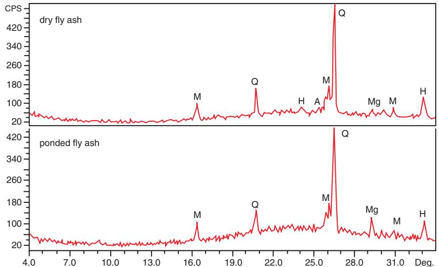
**Figure 1** X-ray diffractograms of dry fly ash and ponded fly ash samples. The mineral peak indications are mullite (M), quartz (Q), hematite (H), anatase (A), and magnetite (Mg). The broad “hump” in the background between about 13 and 30 degrees  $2\theta$  is due to abundant noncrystalline glass in the samples. CPS, counts per second.
