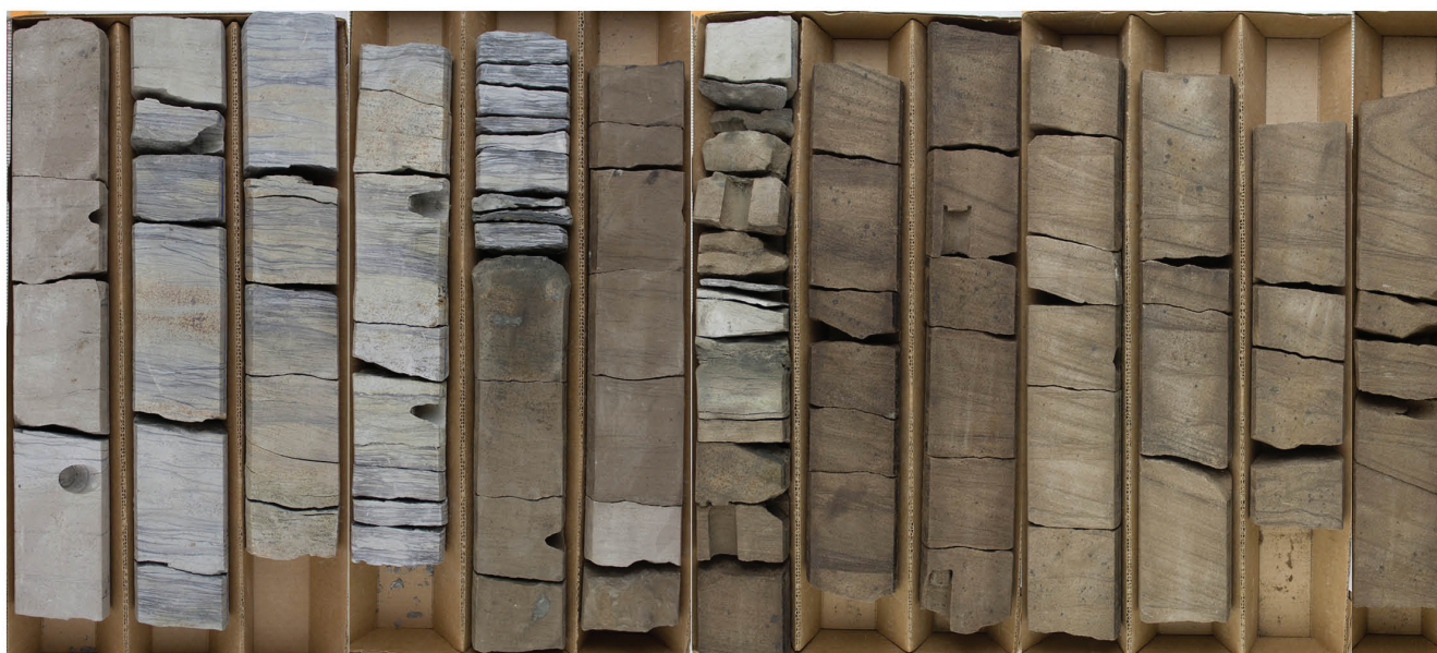
Figure 5 Core from the C.T. Montgomery B-34 well. The top of the core is in the upper left corner and proceeds downhole toward the bottom right. Each box segment is 2 ft (0.6 m) long. The core shows a typical upward change in facies from dominantly cross-bedded and ripple-bedded sandstone to heterolithic strata above. The change in color of the core from light brown to light gray reflects the lack of oil staining in the nonreservoir heterolithic facies. Figure 6 shows a graphical depiction of facies in the Montgomery core.
