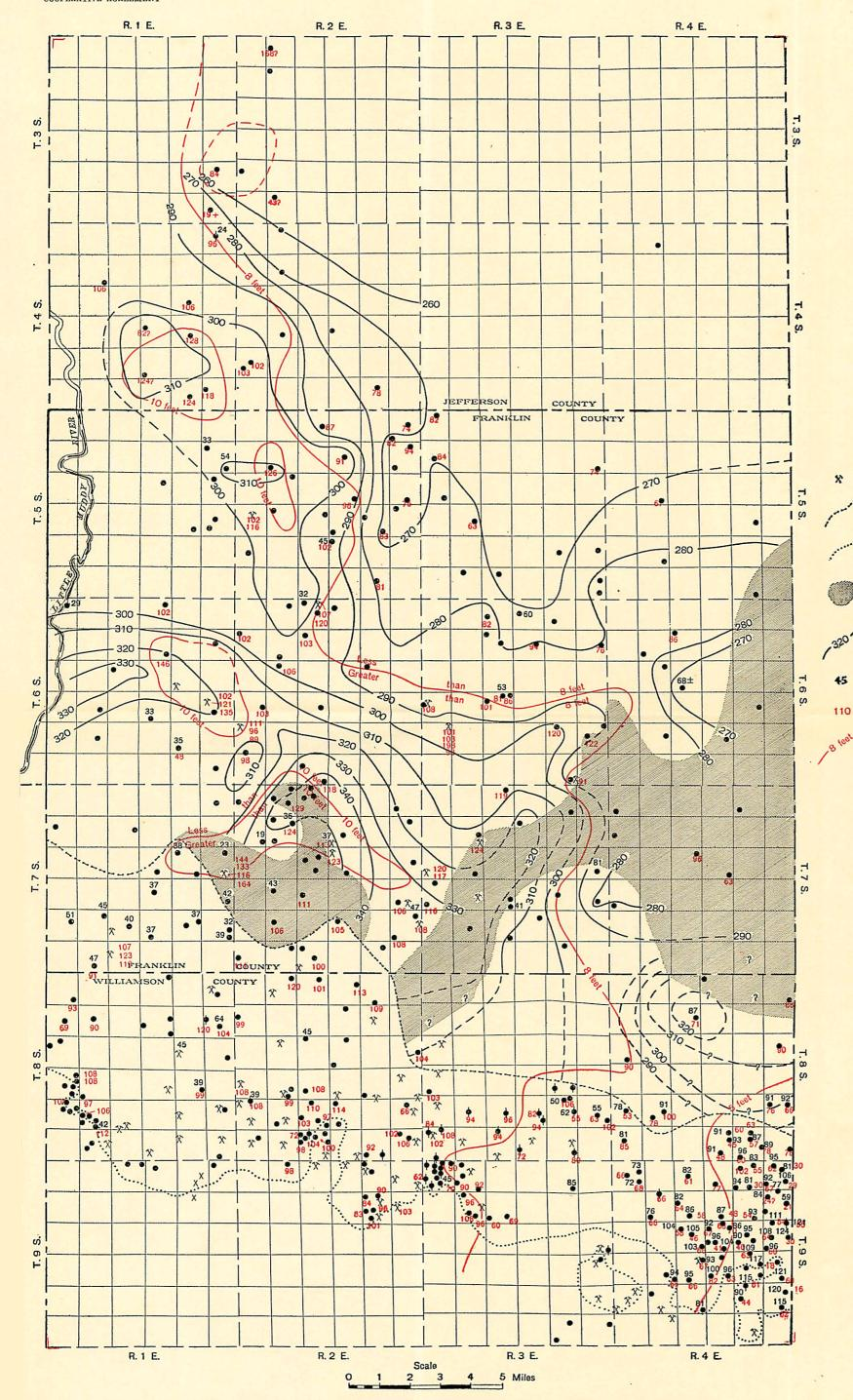
Map showing the distribution of thickness of coal No. 6, the variations in interval between coals No. 5 and No. 6, and convergent contours based on the interval between coals No. 6 and No. 9.
