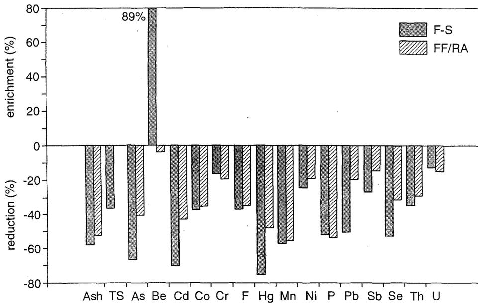
**Figure 8** Mean changes in contents of ash, total S, and HAPs in the <0.150-mm (-100 mesh) samples of 29 marketed Illinois coals as a result of F-S and FF/RA separations. The total S value was not available for the FF/RA tests. The combustibles recovery was 80%.
