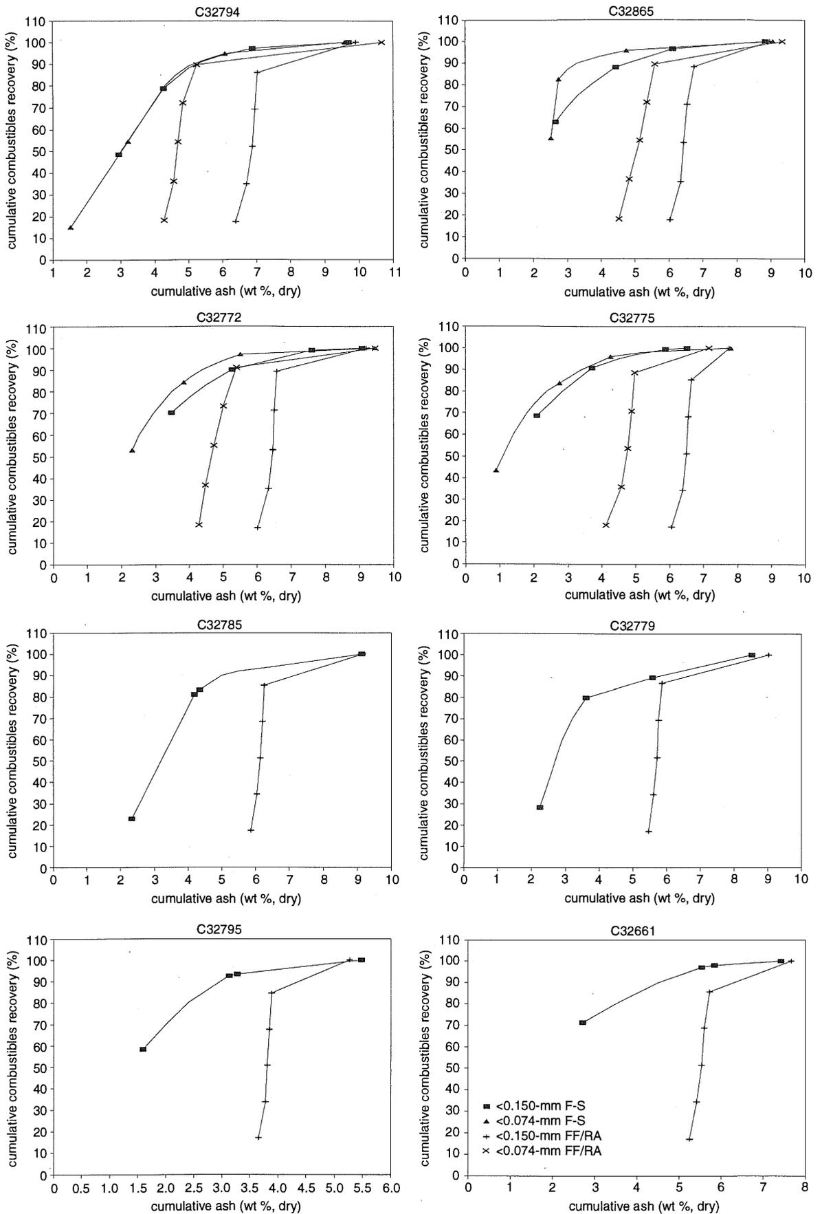
**Figure 3** Examples of ash washability (F-S) and froth flotation/release-analysis (FF/RA) curves for marketed Illinois coals ground to <0.150 mm and <0.074 mm. Sample numbers are given above the graphs. The FF/RA data are from Demir et al. (1995).
