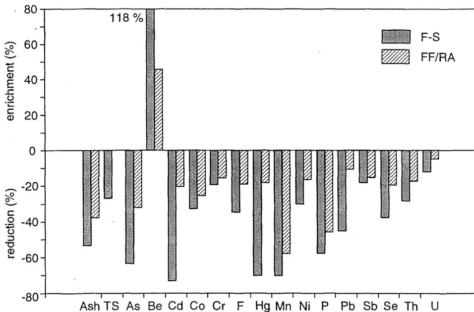
**Figure 9** Mean changes in contents of ash, total S, and HAPs in the <0.074-mm (-200 mesh) samples of ten marketed Illinois coals as a result of F-S and FF/RA separations. The total S value was not available for the FF/RA tests. The combustibles recovery was 80%.
