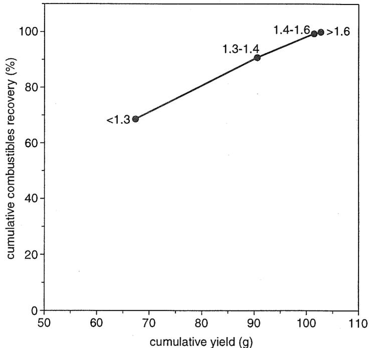
**Figure 2** Relationship between combustibles recovery and cumulative weight yield for sample C32775 separated into four F-S fractions of <0.150 mm. Specific gravities of the F-S fractions are given on the plot.
