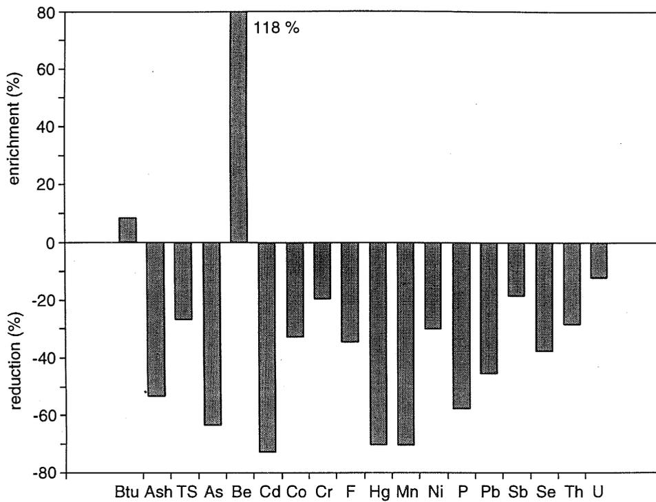
**Figure 4** Mean changes in heating value (Btu) and in concentrations of ash, total S (TS), and HAPs in the 29 samples of marketed Illinois coals as a result of float-sink separation at <0.150-mm (-100 mesh). The combustibles recovery was 80%.
