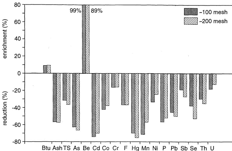
**Figure 7** Mean changes in heating value (Btu) and in concentrations of ash, total S, and HAPs in the samples of ten marketed Illinois coals as a result of F-S separation at <0.150 mm (-100 mesh) and <0.074 mm (-200 mesh) sizes. The combustibles recovery was 80%.
