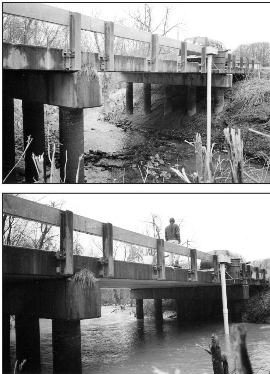
Figure 2 The bridge monitoring site at base flow (top) and flood stage (bottom). The box, pipe, and 55-gal drum mounted to the side of the bridge (on the right) contain a data logger, electrodes, and an ISCO automatic water sampler, respectively.
