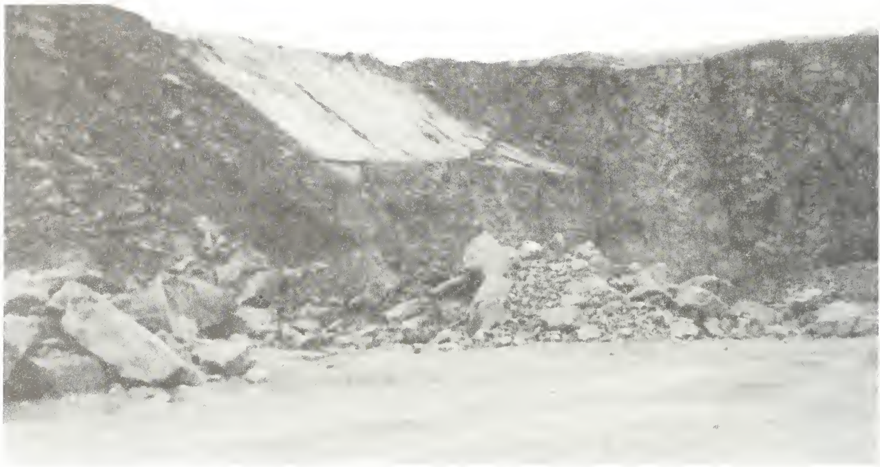
Figure 27 Large slide plane in the north highwall of North Central Materials, Manteno Quarry. The angle of the dipping beds in the highwall indicates that these sediments were deposited on the flank of the reef (photo by W. Frankie).
