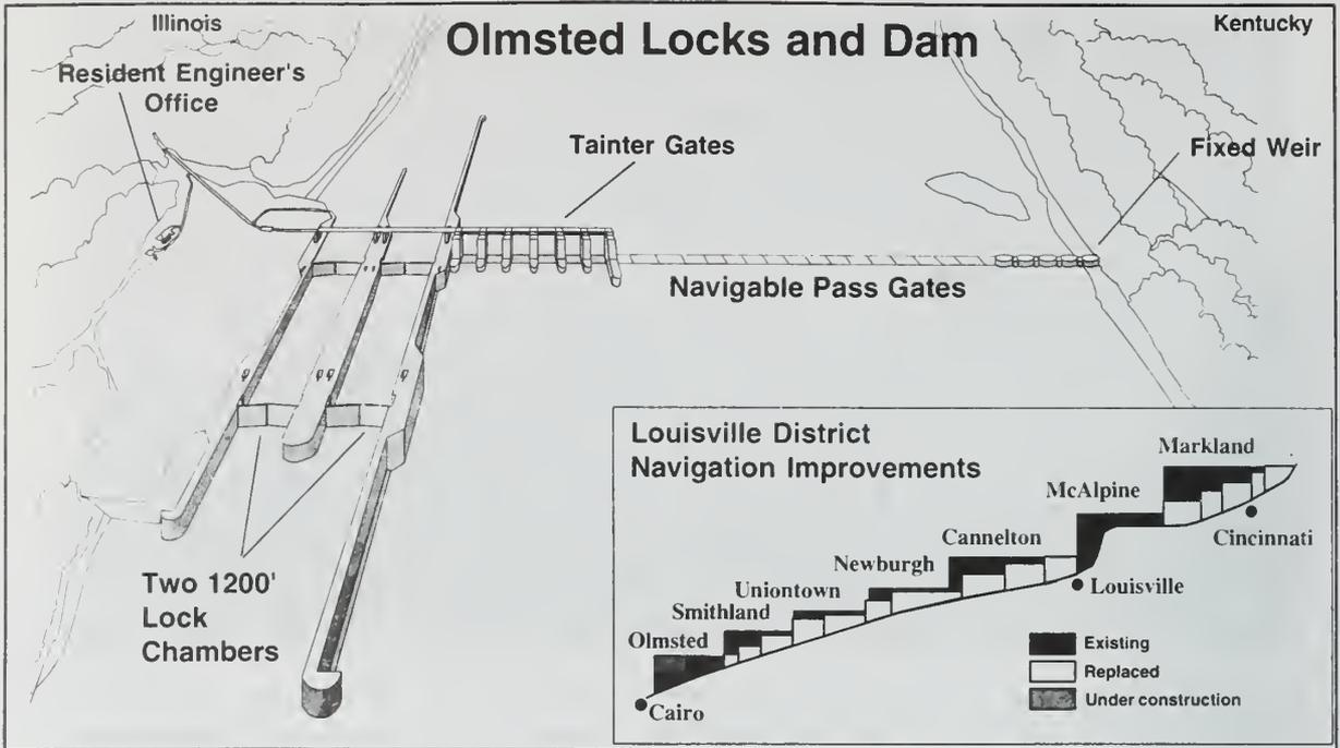
**Figure 14** Artist's rendition of the New Locks and Dam at Olmsted (modified from U.S. Army Corps of Engineers).
