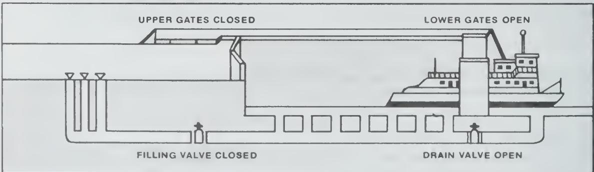
*The water in the lock has here reached the level of the downriver pool. The lower lock gates have been opened and the towboat is leaving the lock to proceed on its way downriver*
