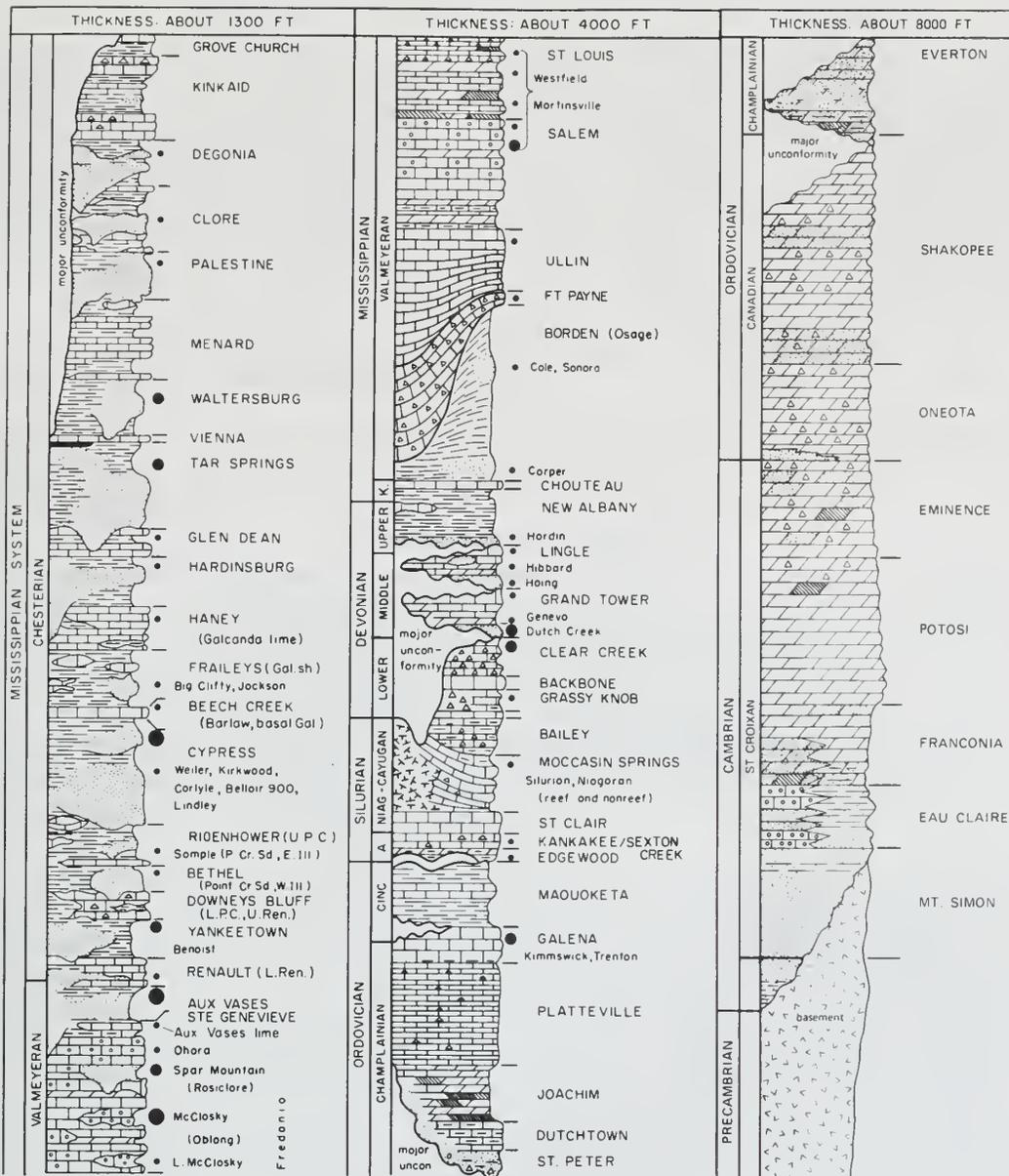
**Figure 2** Generalized stratigraphic column of the Paleozoic rocks in the field trip area. Black dots indicate oil and gas pay zones.. Unconformities are indicated by wavy lines.
