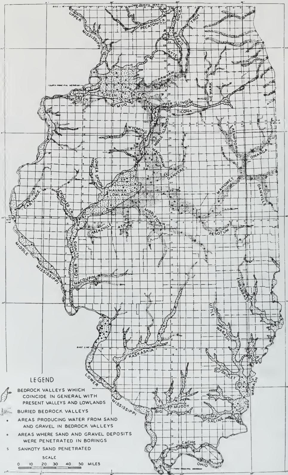
Figure 9 Bedrock valleys of Illinois (modified from Horberg 1950).
