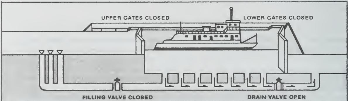
*Now the towboat is in the lock; the upper lock gates have been closed; the filling valve is closed; the drain valve is open, allowing water to drain into the downriver pool. The towboat is lowered as the water level lowers*
