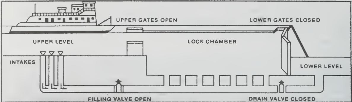
*The lower lock gates are closed; the drain valve is closed; the filling valve is open; the lock has filled to the level of the upriver pool; and the upper lock gates have been opened to allow the towboat to enter the lock*
