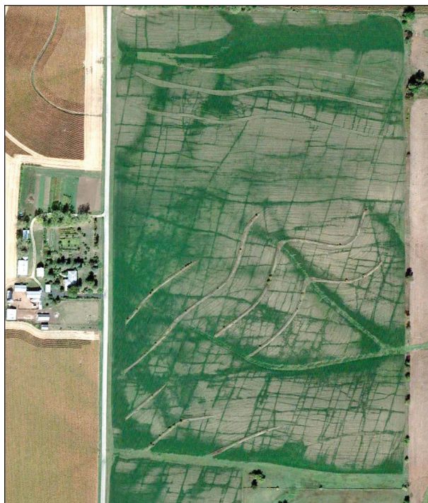
Figure 18 Vegetative crop lines showing fracture and crevice patterns in underlying Galena Dolomite (from Panno et al. in preparation b).
