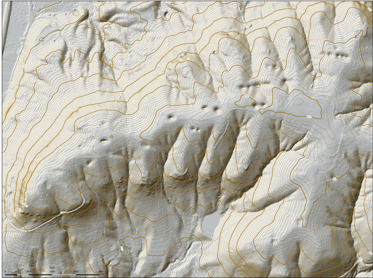
Figure 12 En echelon cover-collapse sinkholes in loess overlying crevices in Silurian dolomite, as shown on a LiDAR (light detection and ranging) shaded relief elevation model. Map by Donald E. Luman.
