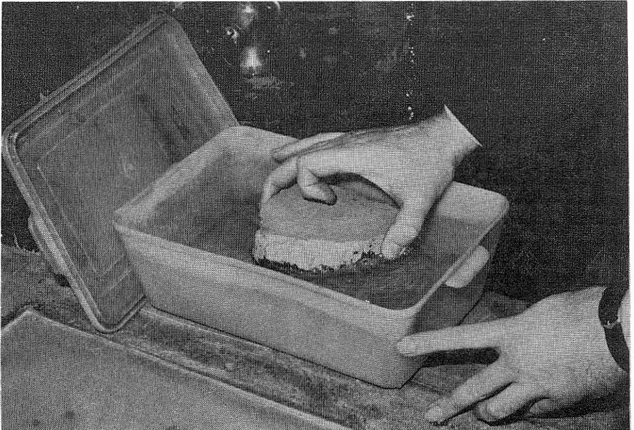
Fig. 12 - Etching a coal-ball slice in 5 percent hydrochloric acid. The untreated surface of the slice is coated with latex paint. The froth of bubbles at the edge of the slice is carbon dioxide released by the reaction of the calcite in the slice with the acid.
