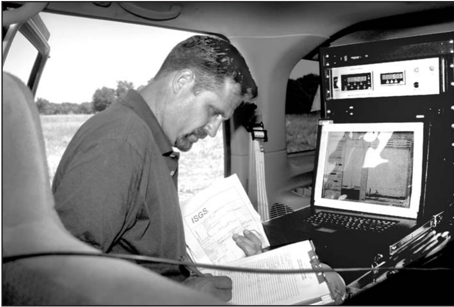
Figure 40 ISGS geologist records information obtained by a sonde as part of a downhole geophysical logging project near Benton, Illinois.
