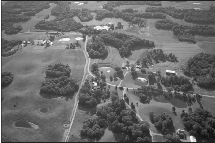
Figure 35 Sinkholes dot the karst terrain of Monroe County in southern Illinois.
