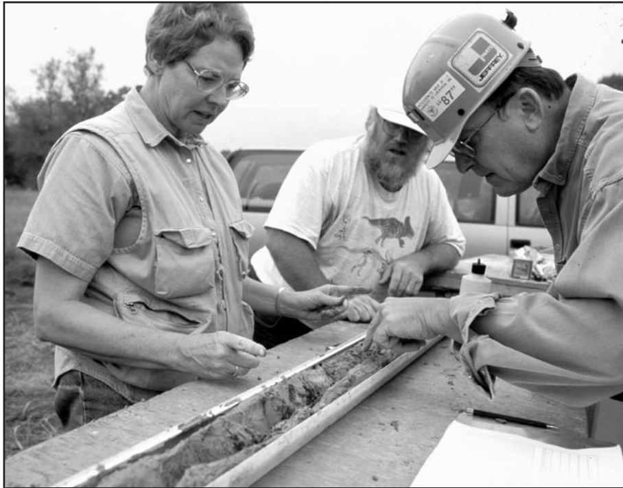
Figure 33 ISGS staff examine a core obtained by a drill rig near Kellerville in Adams County. Drill rigs are used to extract cores, sometimes to depths of several hundred feet, which are then described and analyzed by geologists. These data are basic to making three-dimensional geologic maps and cross sections.
