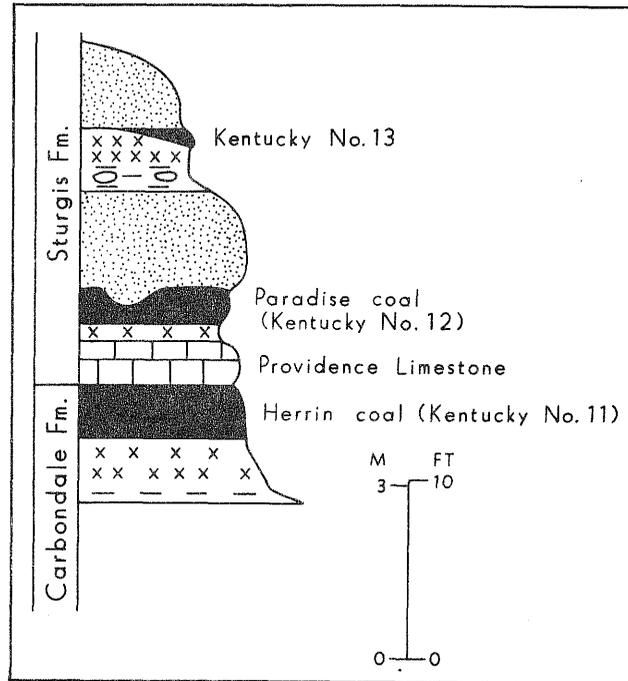
Figure KY-20. Sturgis-Carbondale boundary at Milepost 51, Western Kentucky Parkway. The Paradise coal, absent in the Homestead Mine, is here as much as 5 feet (1.5 m) thick.
