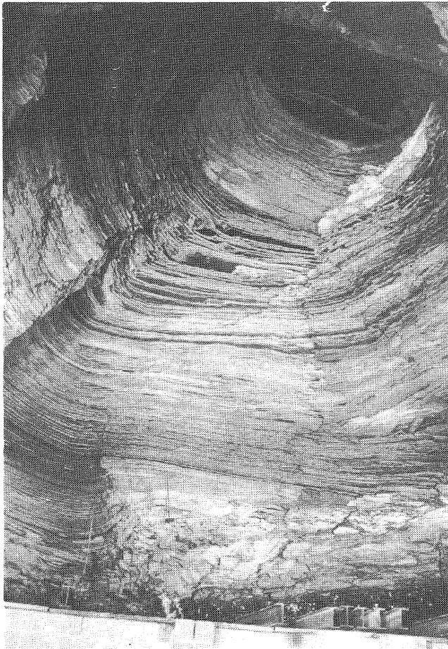
Figure 4. Large roof fall (30 to 40 ft [9 to 12 m] high) in thinly bedded sandstone of the Energy Shale adjacent to the sediments in the Walshville channel. The bedding planes of the sandstone are coated with abundant mica and carbonaceous debris which allow it to break readily into layers. Falls propagate upward with almost vertical walls. In many places the sandstone is porous; the water it contains creates additional mining problems.
