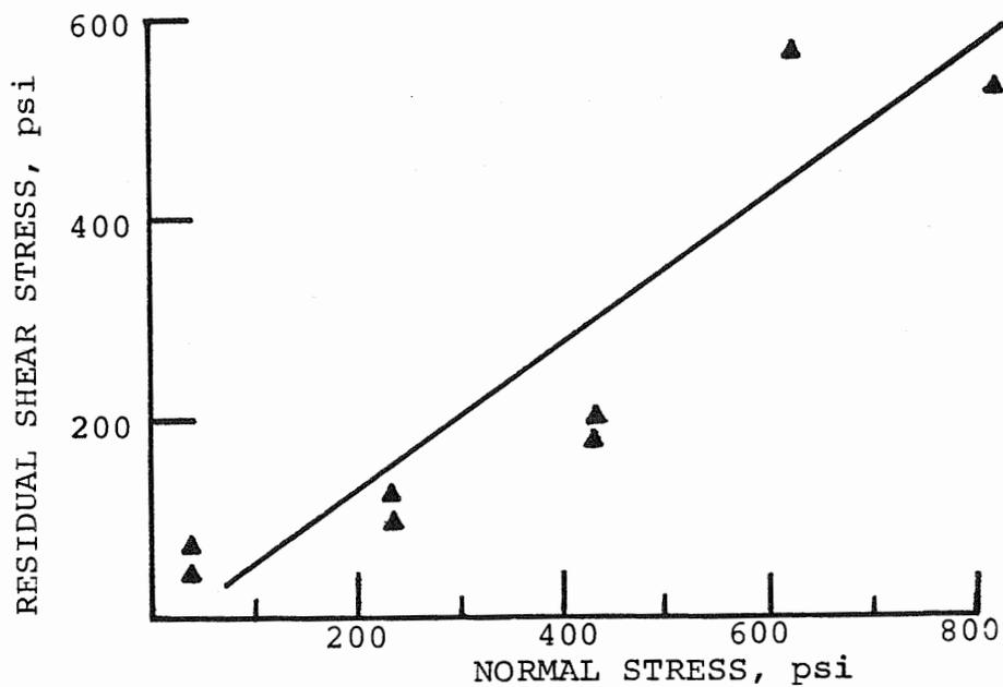
FIGURE 4.17 Residual shear strength-normal stress relationship for coal at Mine 2.
