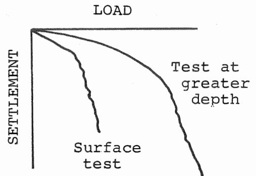
FIGURE 2.3 Modes of bearing capacity failure (after Vesic, 1963).
