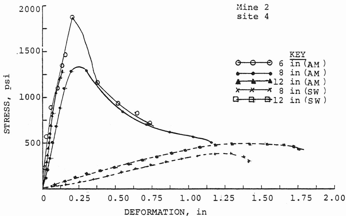
FIGURE A-2 Stress - deformation curves for immediate floor strata based on plate load tests.
