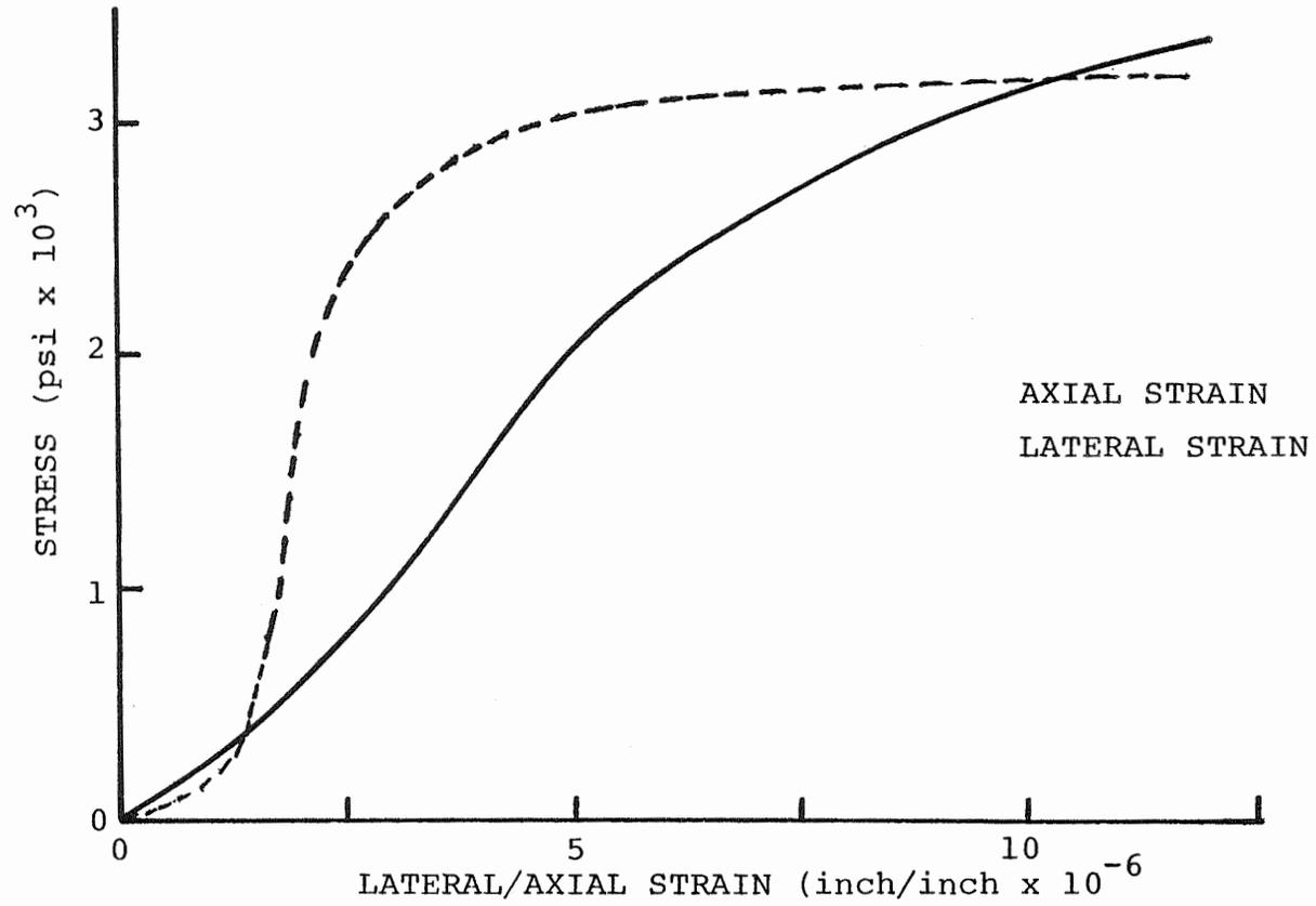
FIGURE C-1. Typical axial stress-axial strain and axial stress-lateral strain curves for a discontinuous rock mass.
