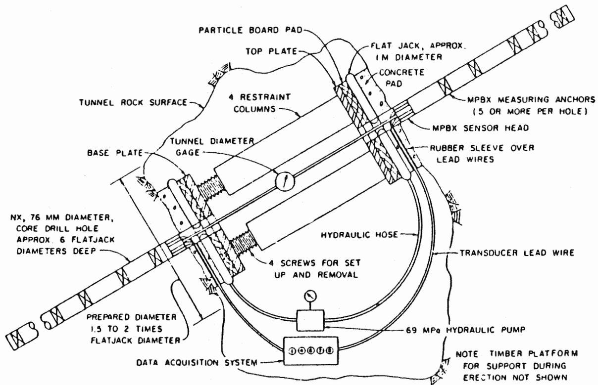
Figure 2.12 In-situ Deformability Measurement Technique (ISRM, 1978)
