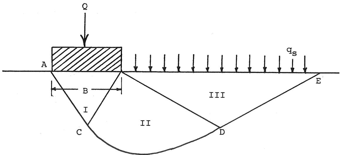
FIGURE 2.1 Bearing capacity analysis of shallow foundations.
