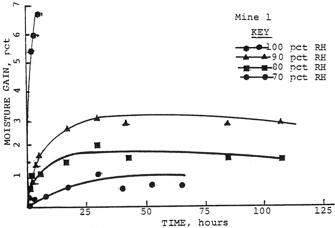
FIGURE 4.18 Moisture gain data for immediate floor strata at mine 1 at different relative humidities
