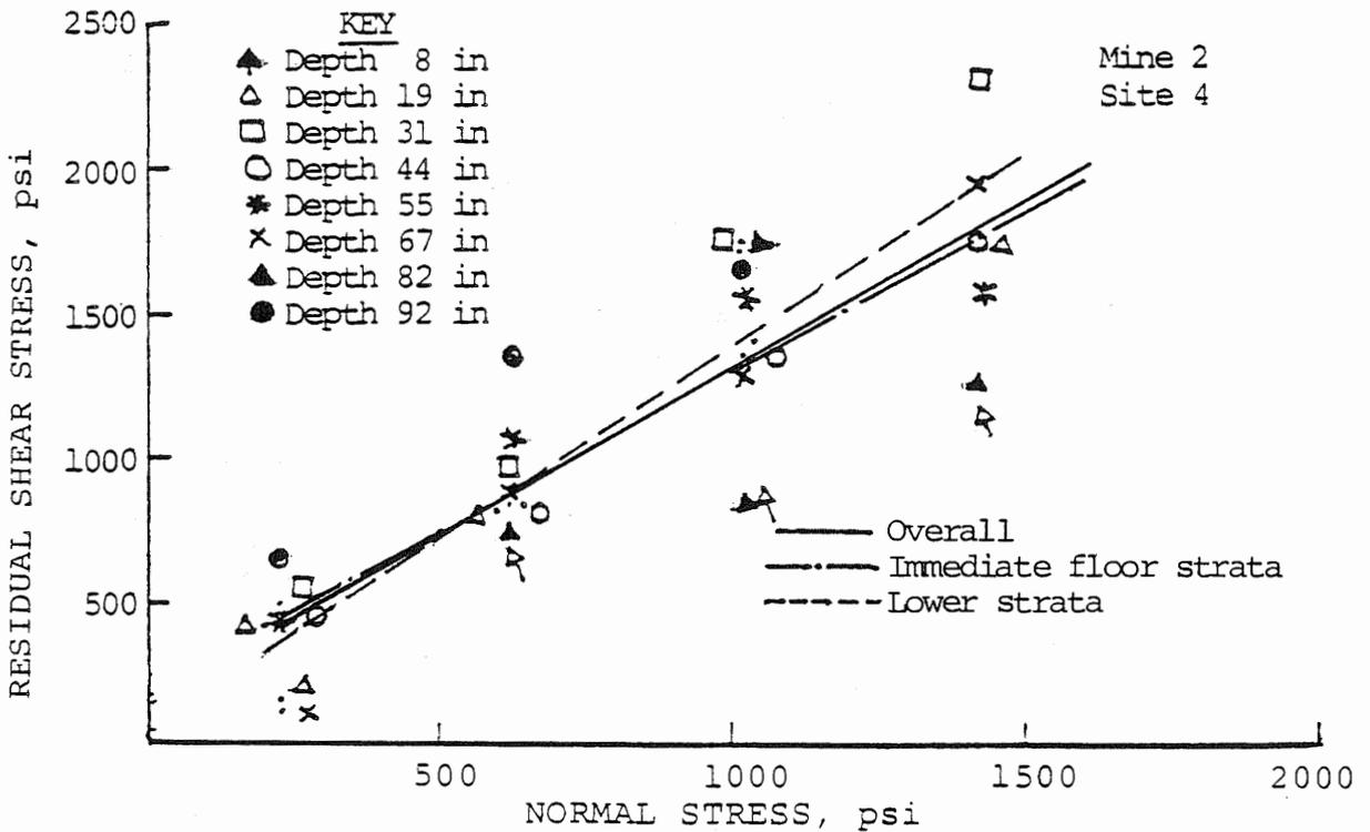
FIGURE B-10 Shear strength - normal stress relationships for immediate floor strata.
