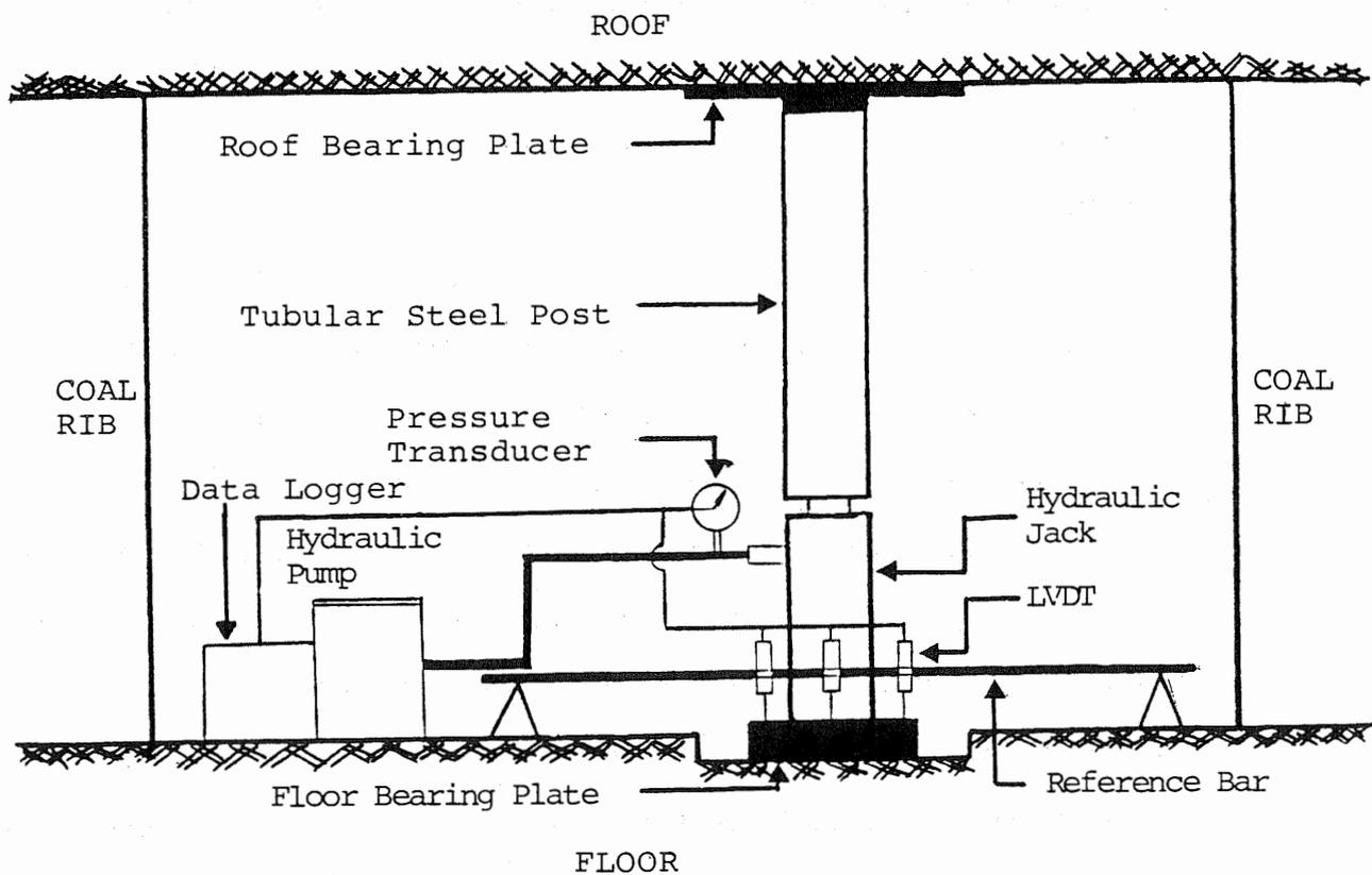
Figure 3.1. Bearing Capacity Measurement Setup.
