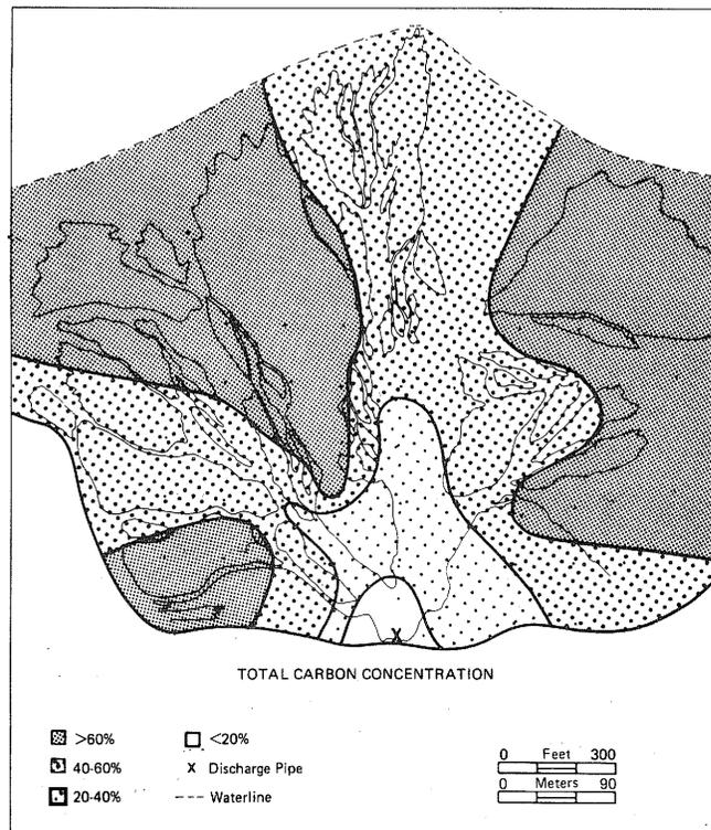
Figure 7. Carbon concentration in the slurry deposit.
