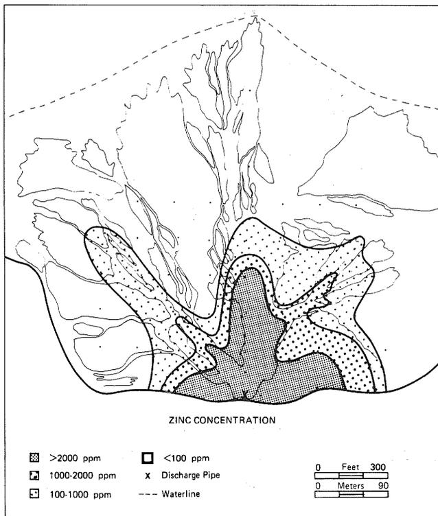
Figure 6. Zinc concentration in the slurry deposit.
