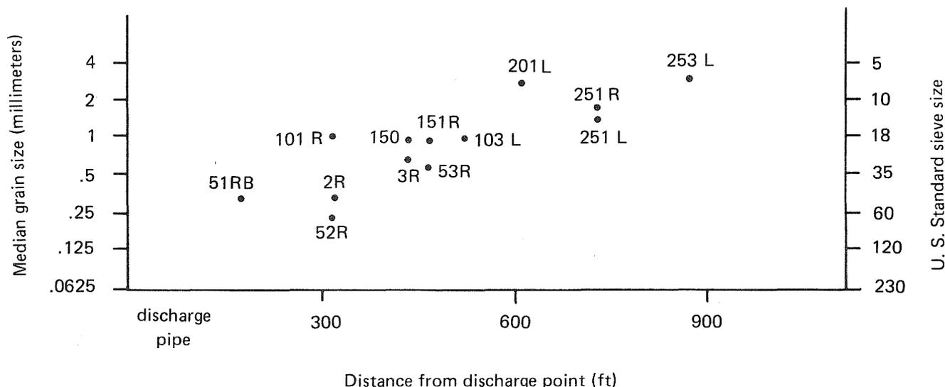
Figure 2. Increase in slurry particle size with increasing distance from the discharge pipe.
