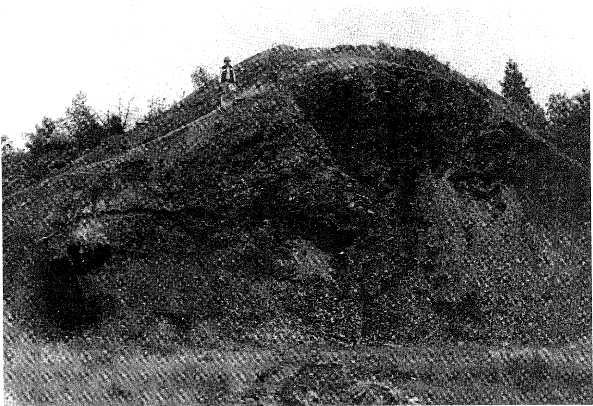
Figure 3. A borrow pit in a mining gob pile at Toluca, Marshall County (NW¼ NE¼ Sec. 8, T 29 N, R 1 E). The shaly mining gob has been burned to a hard, red, bricklike gravel that is used locally as surfacing and fill material.
