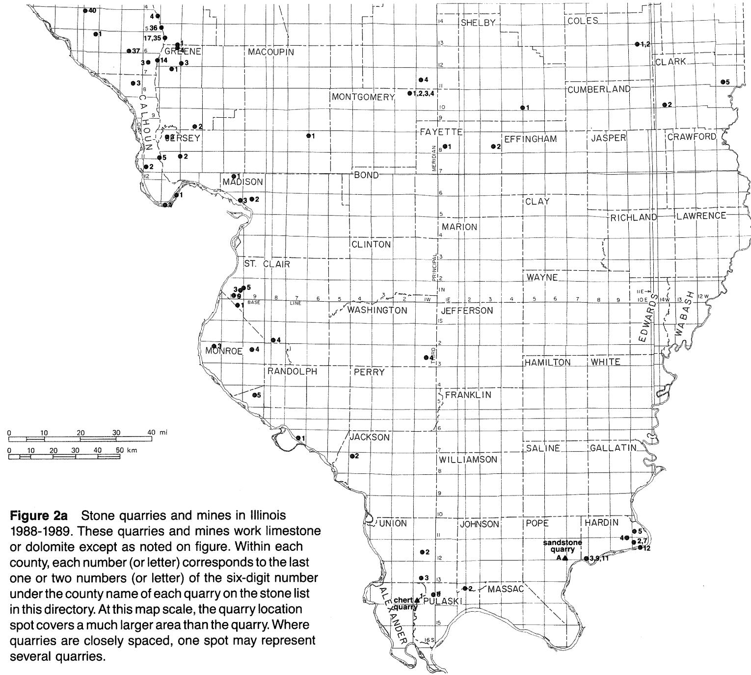
**Figure 2a** Stone quarries and mines in Illinois 1988-1989. These quarries and mines work limestone or dolomite except as noted on figure. Within each county, each number (or letter) corresponds to the last one or two numbers (or letter) of the six-digit number under the county name of each quarry on the stone list in this directory. At this map scale, the quarry location spot covers a much larger area than the quarry. Where quarries are closely spaced, one spot may represent several quarries.
