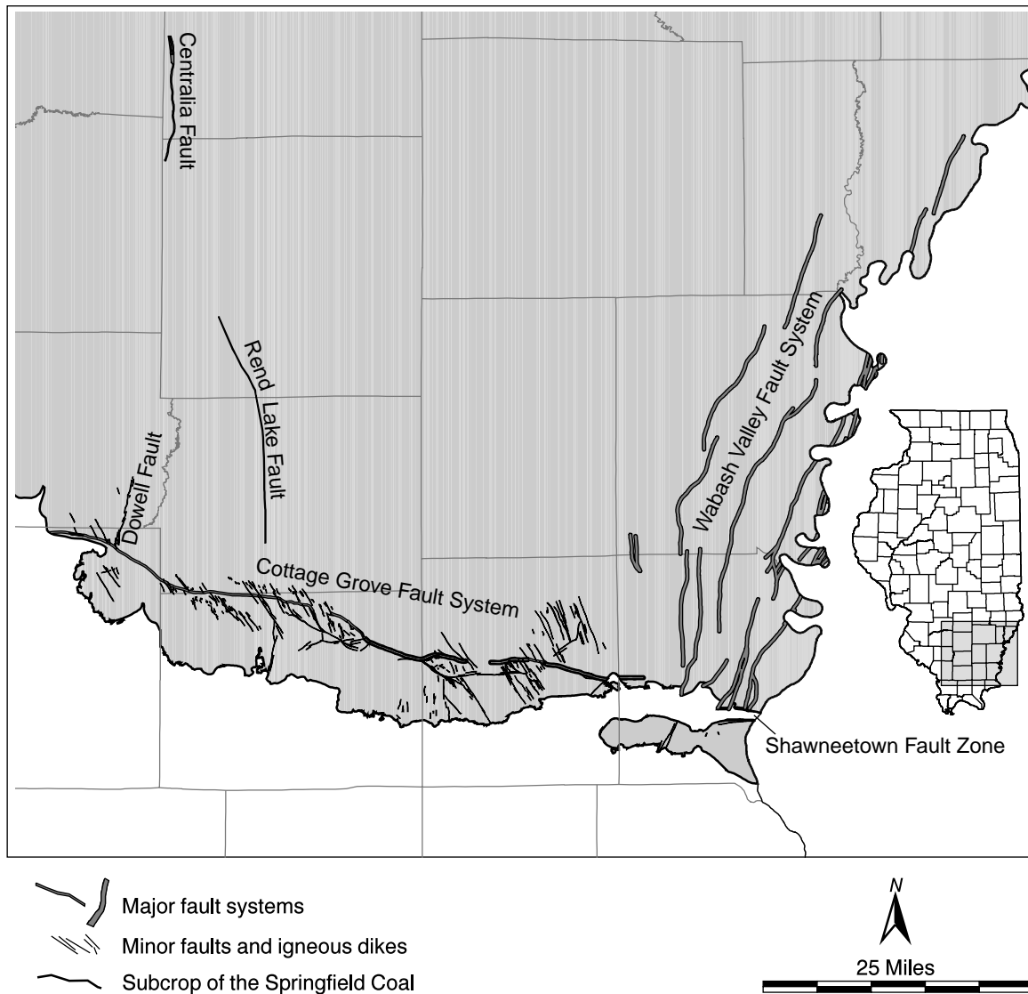
Figure 22 Areas of Springfield Coal affected by faults and igneous dikes.
