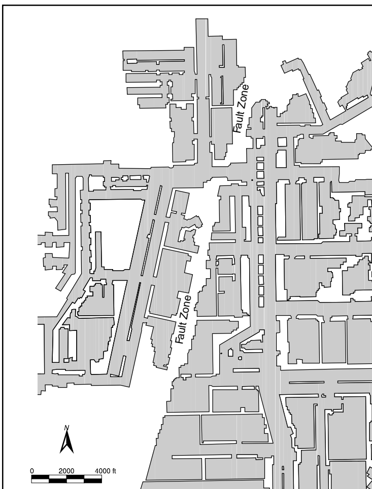
Figure 21 Unmined areas adjacent to one of the faults in the Wabash Valley Fault System (from Treworgy et al. 1998).
