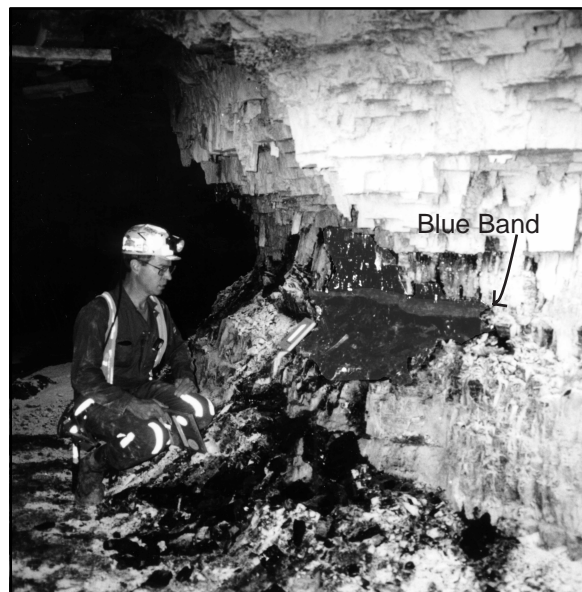
Figure 31 Rib rashing in the Herrin Coal; note the position of the blue band.
