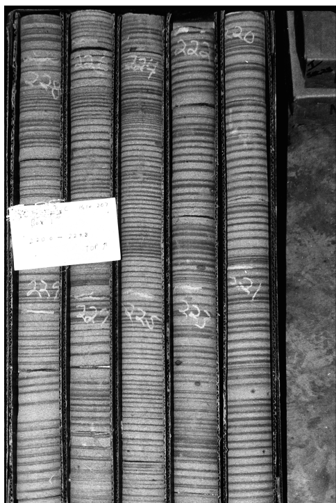
Figure 34 Core of the laminated siltstone and shale facies of the Energy Shale, Douglas County (Coal Section files, ISGS).
