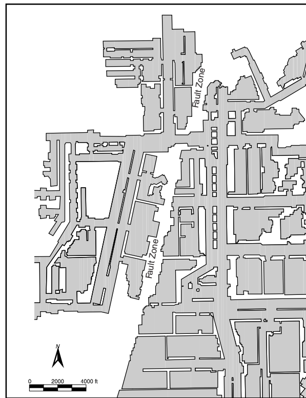
Figure 28 Unmined areas adjacent to one of the faults in the Wabash Valley Fault System (from Treworgy et al. 1998).
