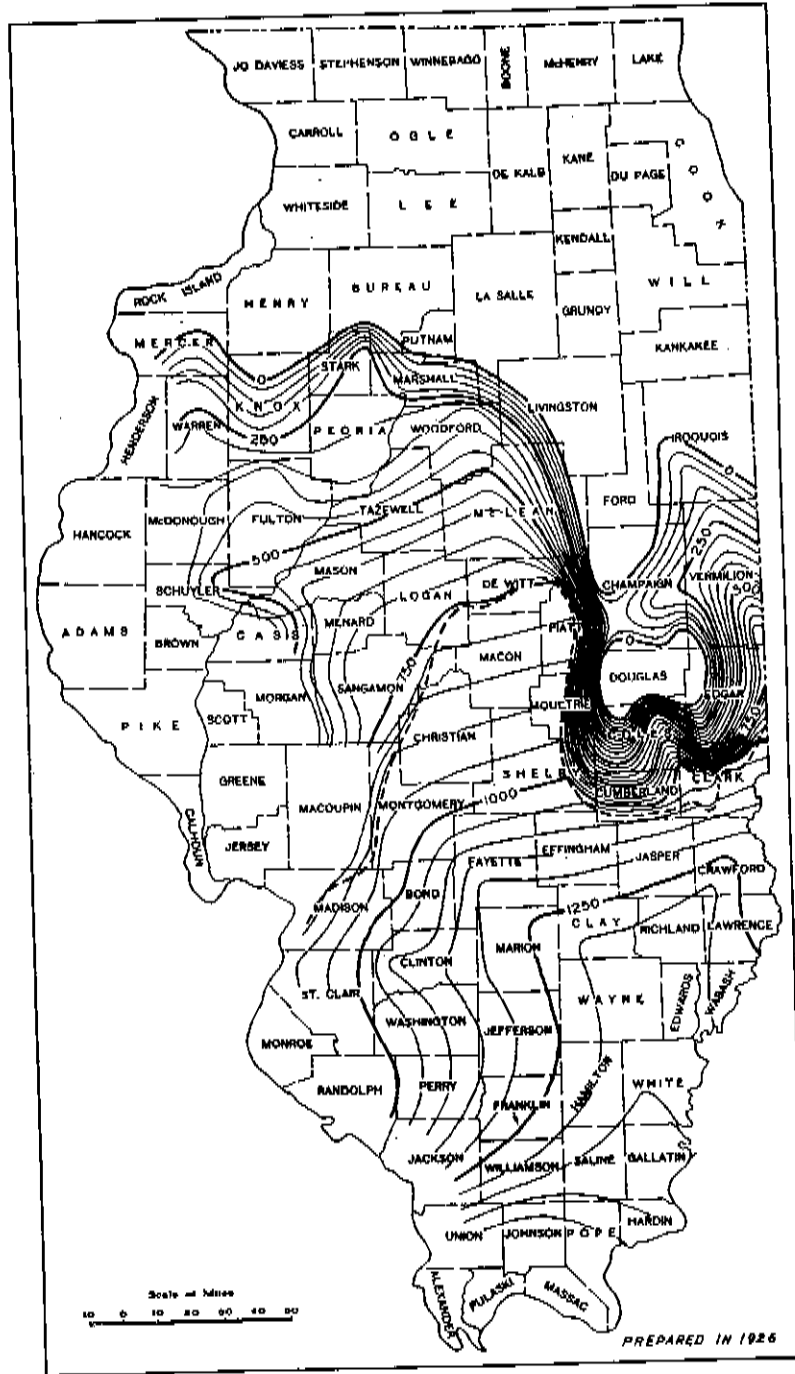
FIG. 7.—ISOPACH MAP SHOWING THE THICKNESS OF THE LOWER MISSISSIPPIAN STRATA For correction see explanation below Plate I
