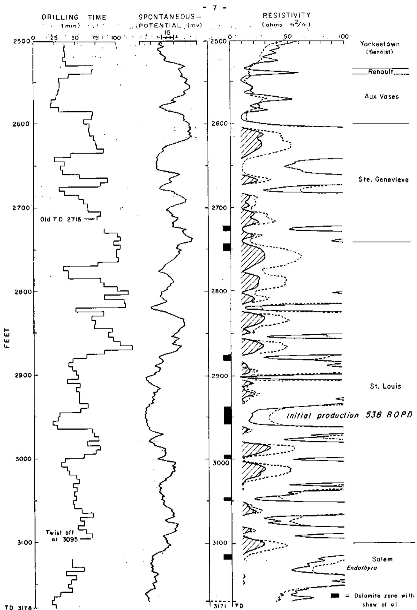
Fig. 4 — Drilling time log and electric log of Union Oil Company of California
