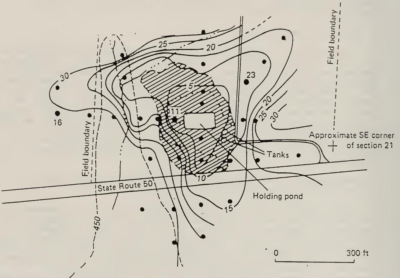
— 10 — Contour showing apparent resistivity; interval 5 ohm-meters
