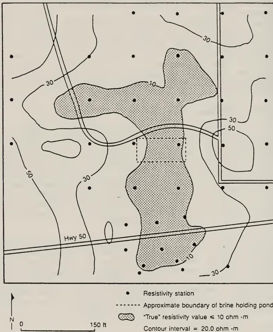
Figure 9-14. "True" resistivity contours at site A. Approximate depth is 6 meters.
