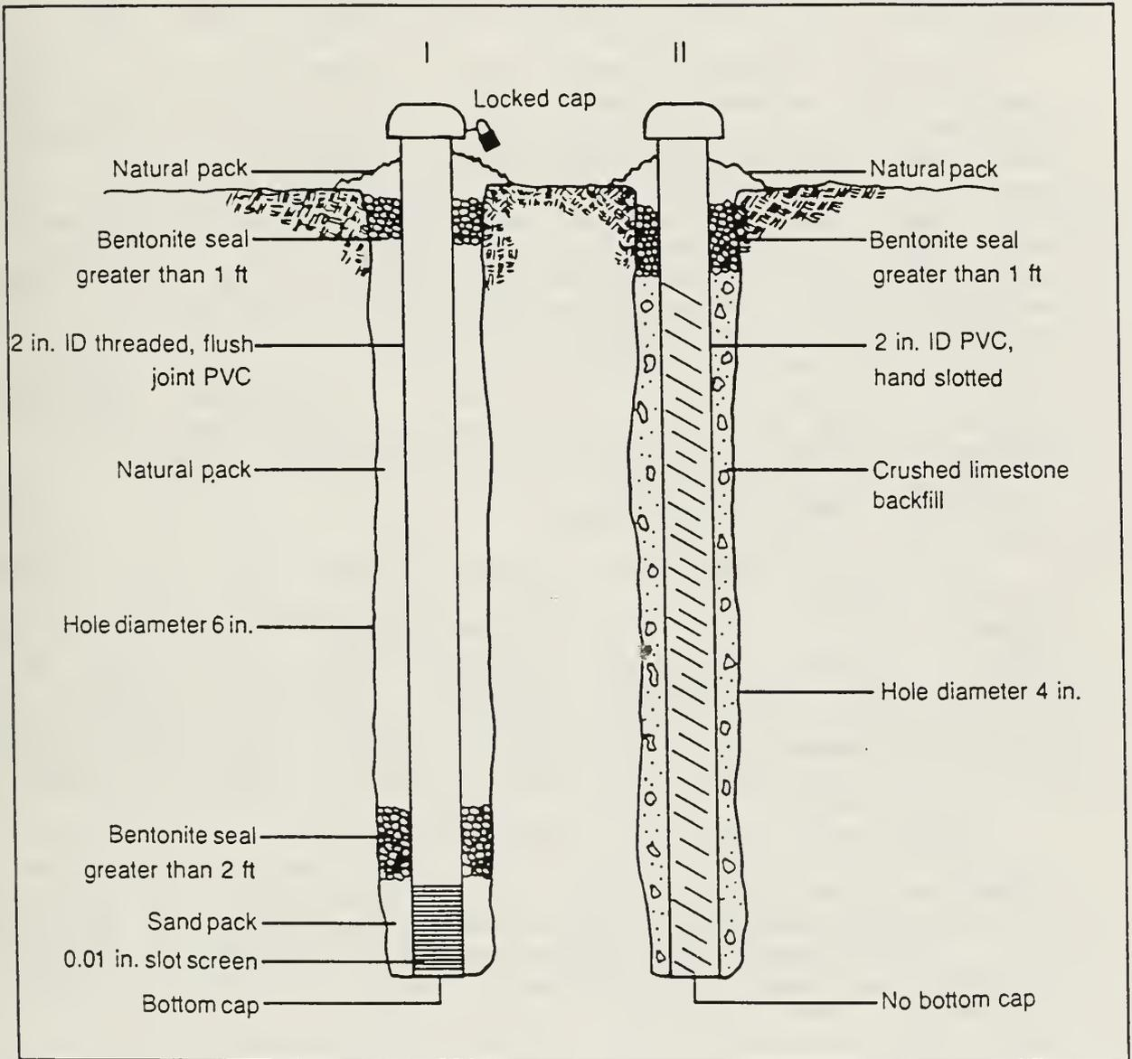
The piezometers were constructed of 2-inch diameter, threaded, flush-joint PVC pipe. Each well was completed with a 2.5 foot, 0.01 inch slotted screen at the base. The annulus of the borehole was filled with; 1) silica sand to the top of the screen, 2) a bentonite seal of at least 2 feet overlying the sand pack, 3) cuttings from the lower seal to near surface, and 4) another foot of bentonite at the surface (figure 9-2).
