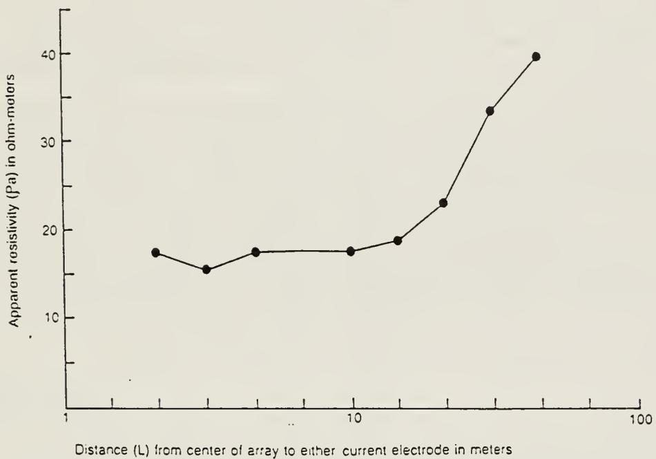
Figure 9-7. Layering parameter solution for VES curve presented on figure 9-6.
