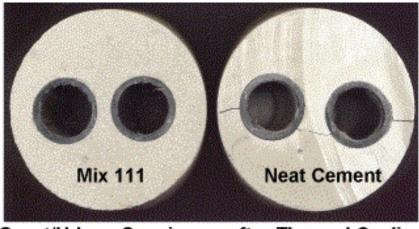
Grout/U-loop Specimens after Thermal Cycling
