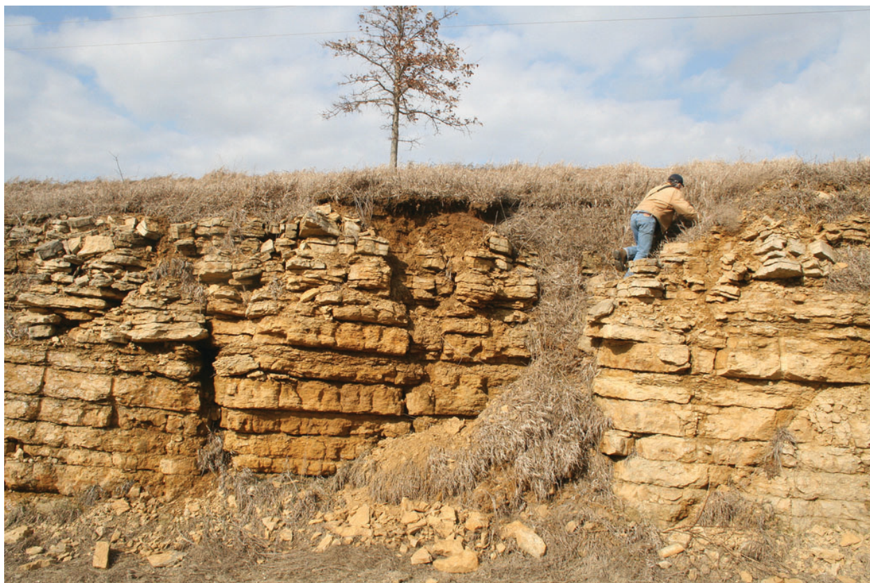
Figure S11. A closeup of the above road cut showing numerous crevices between 1 to 6 inches wide. Bedding planes were prominent throughout the exposure.
