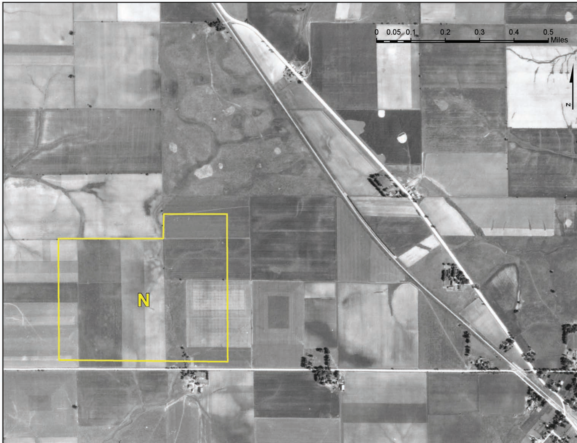
Figure 7. Aerial photograph in vicinity of the site for the proposed dairy facility taken July 1, 1947. The area near the top center part of the photograph shows what appear to be sinkholes in a pasture located just north to northeast of the Traditional North (N) site. In the 2005 aerial photograph, the pasture has been converted to row crops and almost all traces of the sinkholes have been obscured (Figure 6).
