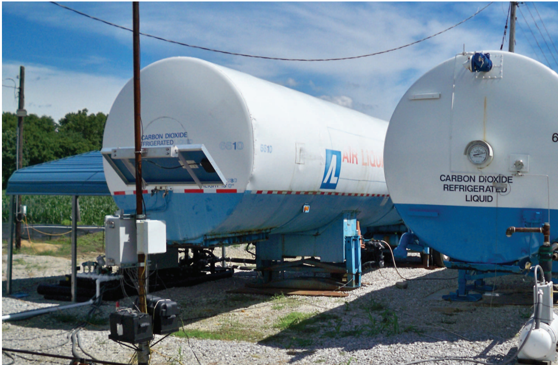
Figure 46 Portable Air Liquide CO 2 storage tanks. Tank capacity is 55 tonnes (60 tons) of CO 2 . Photo courtesy of Trimeric Corp.
