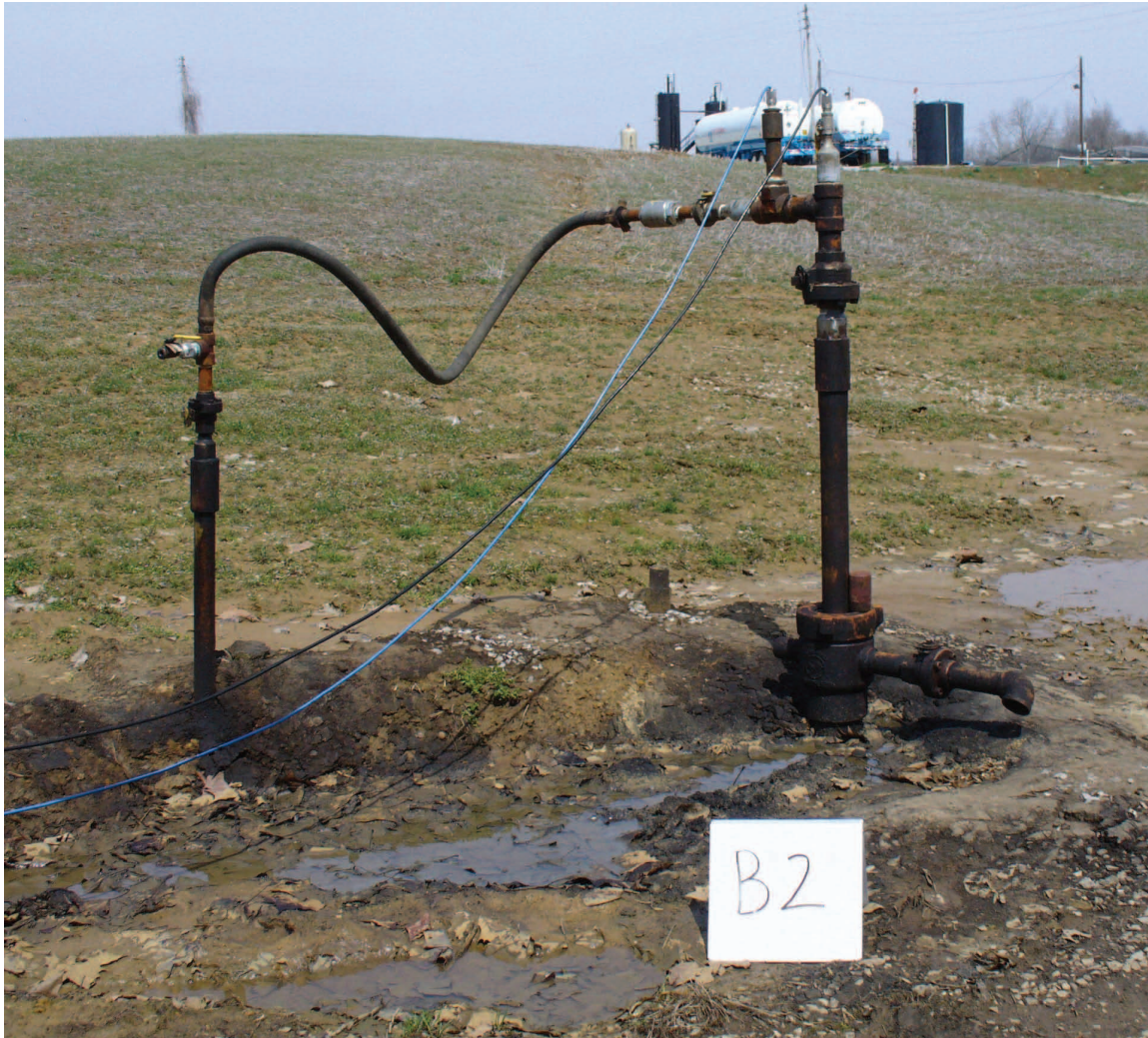
Figure 57 A typical production wellhead (right), IB-2 (B2), at the Bald Unit. The Bald Unit tank battery and CO 2 storage tanks are visible in the background. The cables emerging from glands on the wellhead are for pressure (black cable) and temperature (blue cable) gauges. Production flow line is to the left.
