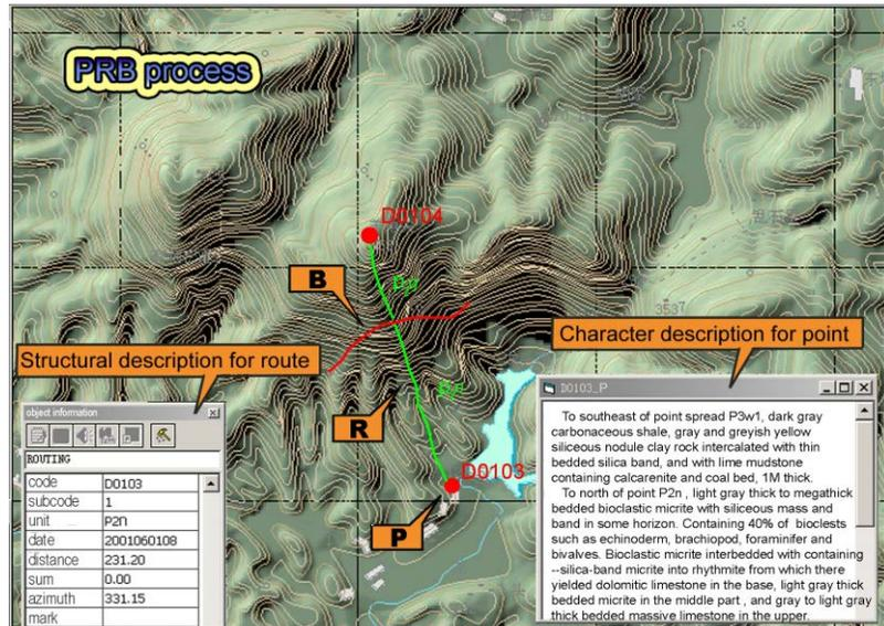
Figure 2. Concrete expression of the PRB process.
