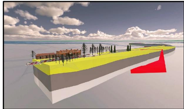
Figure 4. Example of BIM infrastructure design elements integrated with geological subsurface information, including faults. (BGS)
