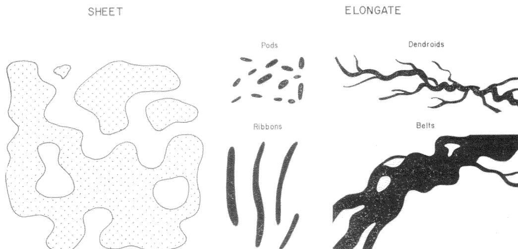
Fig. 7—Patterns of sheet sand bodies and the four types of elongate sand bodies—pods, ribbons, dendroids, and belts.
